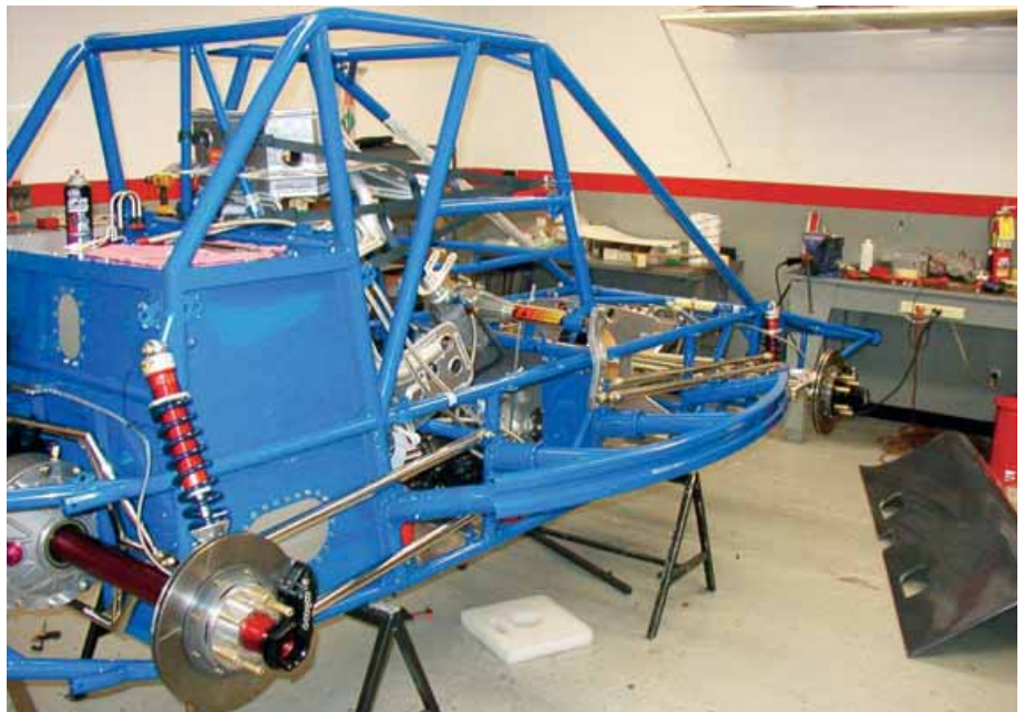
The side-mounted crush structures locate in hard points along the side of the chassis preventing intrusion
