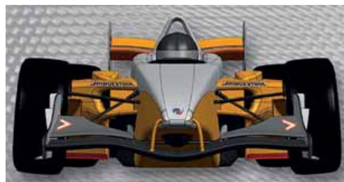
The 2007 Champ Car will be smaller and lighter, powered by a 775bhp version of Cosworth's 2.65-litre V8
