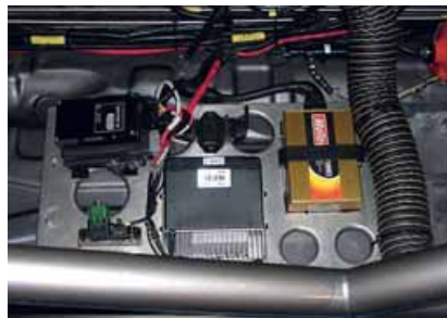
MoTeC's M880 ECU installed in the WTCC Chevrolet Lacetti
