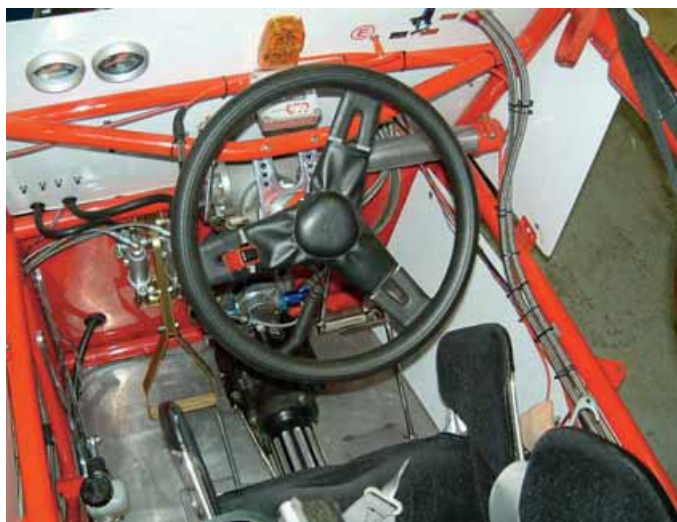
At 34 inches the cockpit is some 5 inches wider than previous Silver Crown cars
