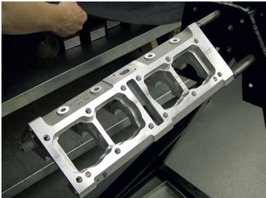
Everything on the RST is pared down to the minimum to make it lightweight, here the crankcase
