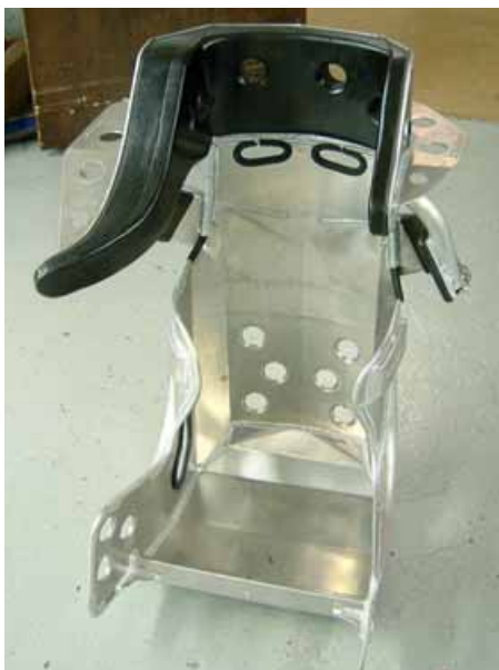
All-embracing seats were a mandatory requirement of the new Silver Crown cockpit specifications
