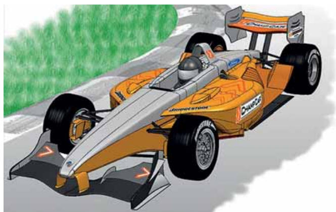
The 2007 Champ Car will be smaller and lighter, powered by a 775bhp version of Cosworth's 2.65-litre V8
