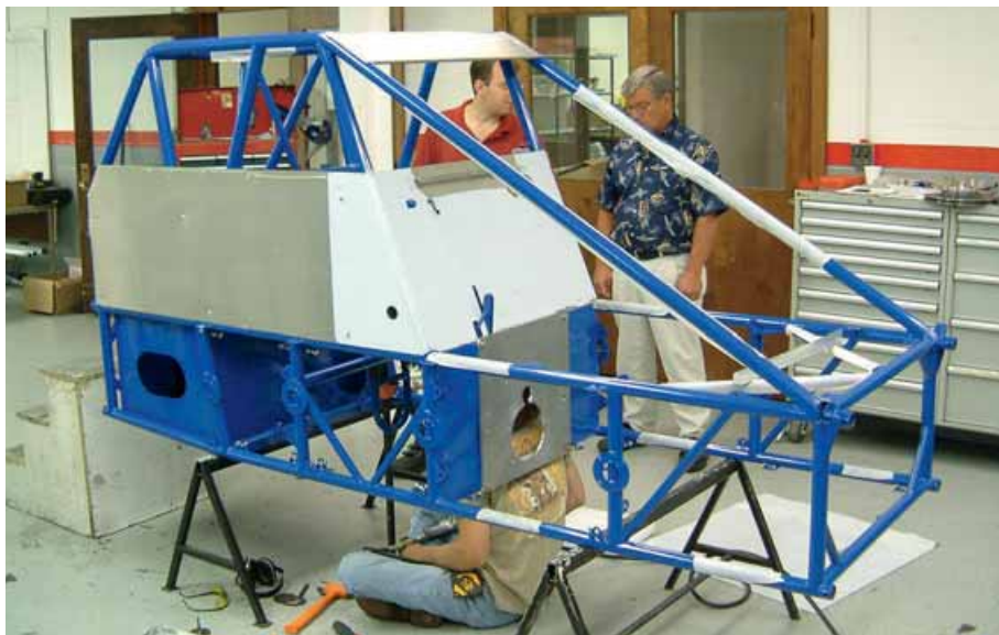
Basic chassis is a simple triangulated frame with a roll structure design dictated by USAC's regulations
