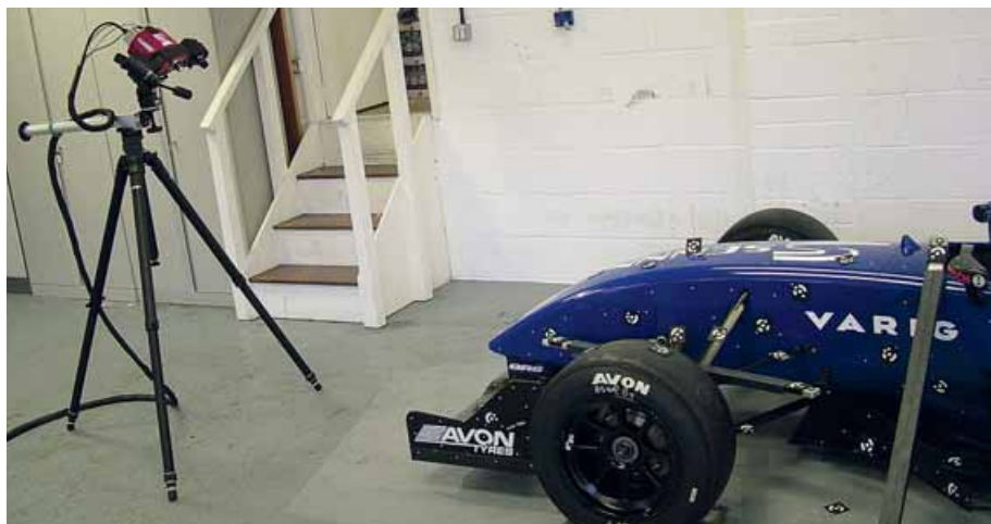
Physical Digital's ATOS optical scanner in operation at RR Racing's Woking headquarters
