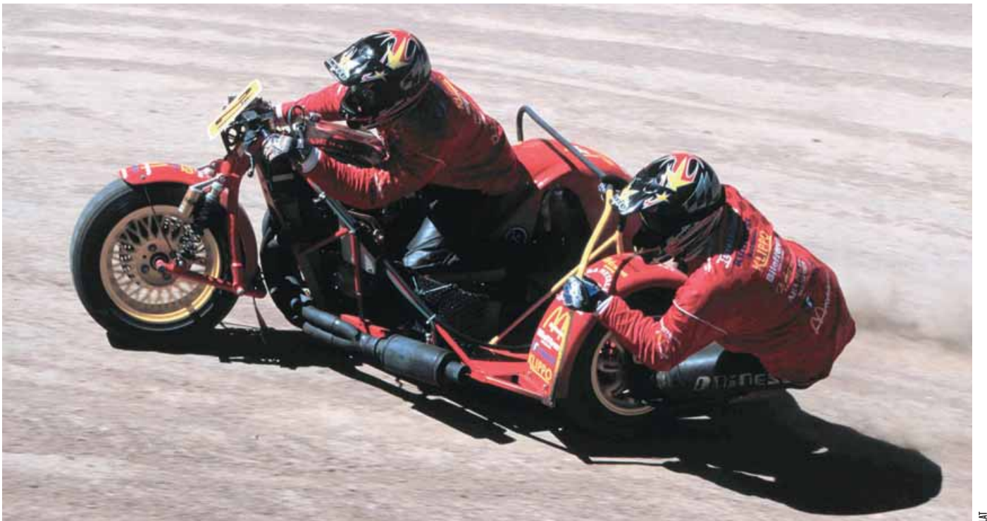
2000 Pikes Peak Hillclimb. Swedes Anders Nilsson and Tom Grindberg demonstrate the art of motorcycle sidecar racing. Even with the optimum centre of gravity – as far away from the two-wheeled side as possible – and a wheel spread as wide as regulations permit, rollovers are a very definite possibility
