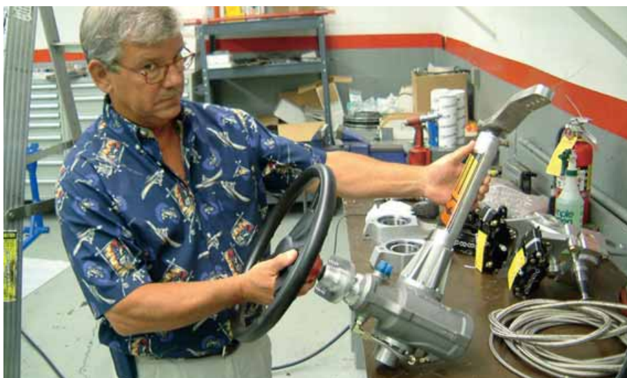
Ron McMahon holds the worm and sector steering system with power assistance and detachable wheel
