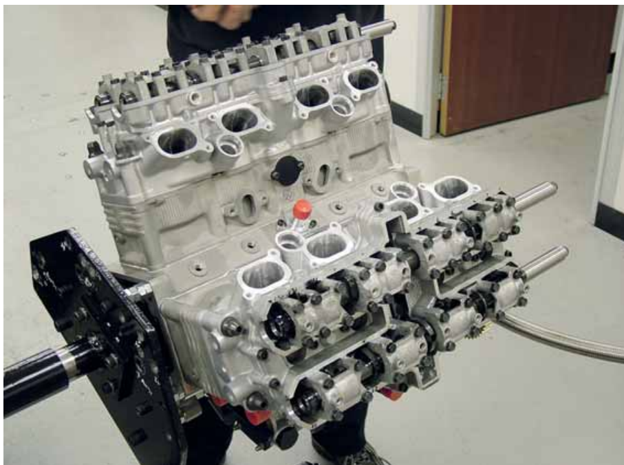
The V8 is being productionised at Mountune's Essex HQ, the engine specialist will also market the engine Cavity left in the centre of the engine where the timing chain would have sat, RST cams now belt driven
