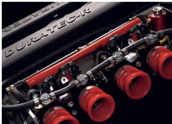
Webcon's Alpha-managed throttle bodies on a Ford Duratec-R engine
