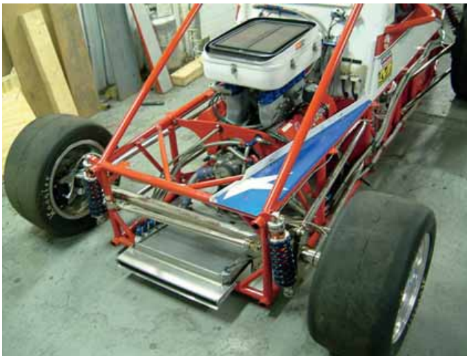
New rules mandate a symmetrical chassis to reduce adhesion on paved ovals
