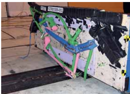
Crash testing of the mandatory, detachable front, rear and side structures has allowed a known level of driver protection to be incorporated into the cars
