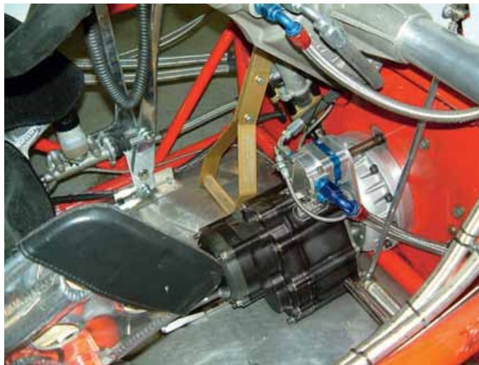
Transmission is a two-speed unit, unusually for a Silver Crown racecar
