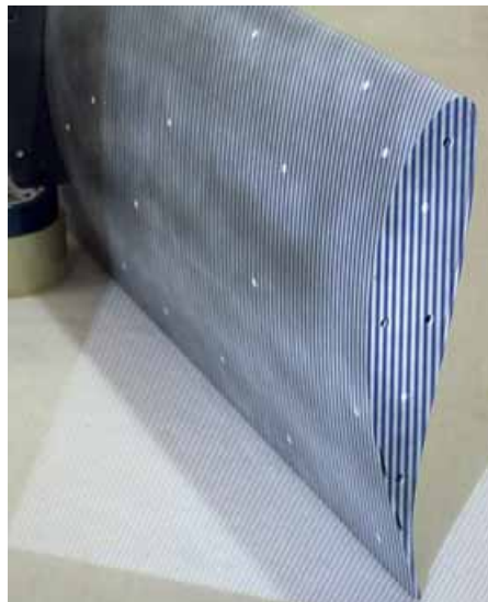
Figure 4: setting up the ATOS optical scanner to measure a wing mainplane (McBeath)
