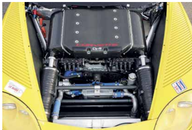
Engine placement is limited by regulations mandating stock firewall location
