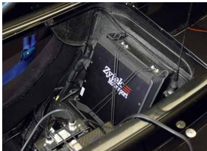
Zytec's management unit on its own race winning LMP1 sportscar, the 04S
