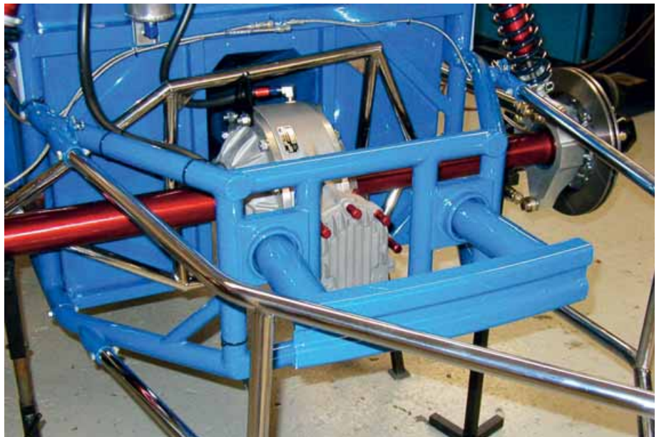
A similarly replaceable crush structure is used at the rear inside the removable tail supporting frame
