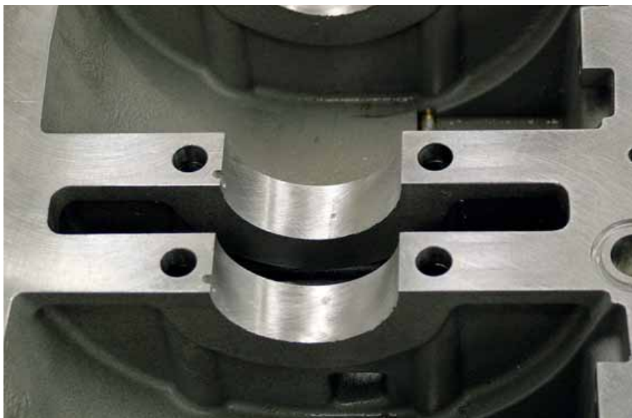
The V8 is being productionised at Mountune's Essex HQ, the engine specialist will also market the engine Cavity left in the centre of the engine where the timing chain would have sat, RST cams now belt driven
