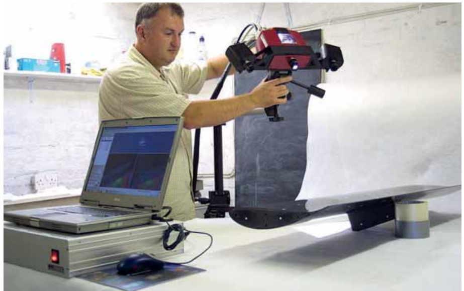
Figure 4: setting up the ATOS optical scanner to measure a wing mainplane (McBeath)
