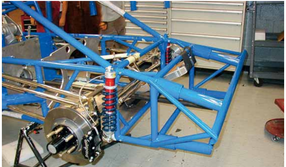
Front crush structure is removable and feeds loads into the chassis at rigid nodes dispersing forces
