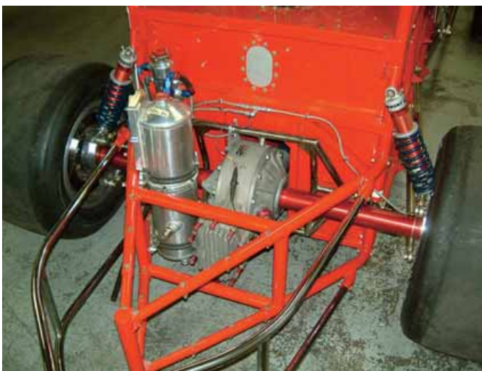
Panhard rod is a truss-like structure located above and below the differential
