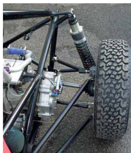
Front suspension (above) features double unequal length wishbones, fabricated uprights and 8in of suspension travel
