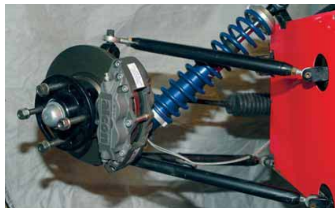
Front suspension (above) features double unequal length wishbones, fabricated uprights and 8in of suspension travel
