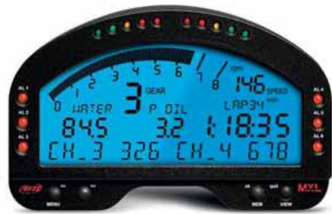
Aim units are available as in-dash displays or as steering wheel versions under the company's MyChron brand. A smaller kart version has also recently been launched
