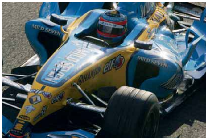
Renault's side pods are roughly aerofoil shaped, with a complex array of winglets and chimneys. Smaller radiator inlet shape is similar to that used by McLaren
