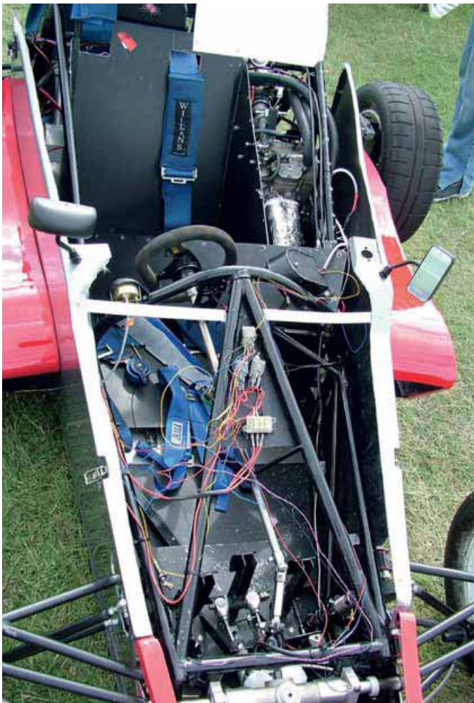
Here's an example of a wiring loom in an FSUK car that has not been properly thought out. It works, but for how long?
