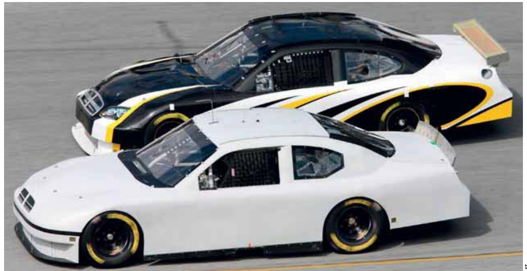
Rear, boot-mounted wing seen at Daytona looks to be a sign the COT did not perform as expected, aerodynamically
