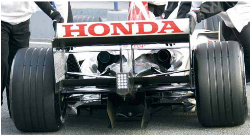
Central rear wing supports are catching on this year as a way of taking loads out of the end plates and freeing up their design. Toyota was one of the pioneers last year with BAR [left] who, as Honda, is retaining the design on its cars
