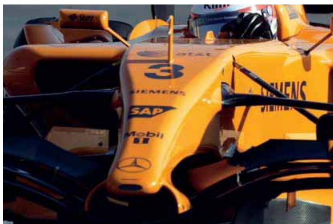
McLaren has employed some cunning structural engineering to get its 2006 spec nose (left) through the FIA crash test. Compare it to the 2005 spec nose (above)
