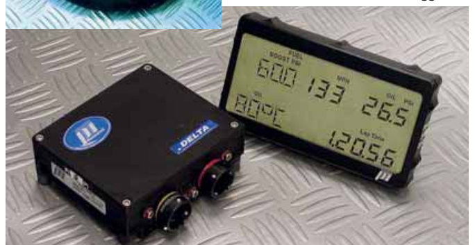
Pi Xpress X Sport (above). Compact C-dash (below) connects to Pi Research's Delta Lite logger
