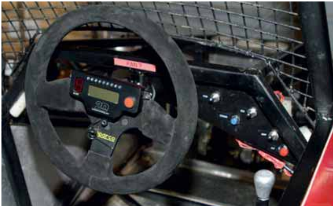
EFI Gear Dash offers a wealth of instant feedback through 16 input channels
