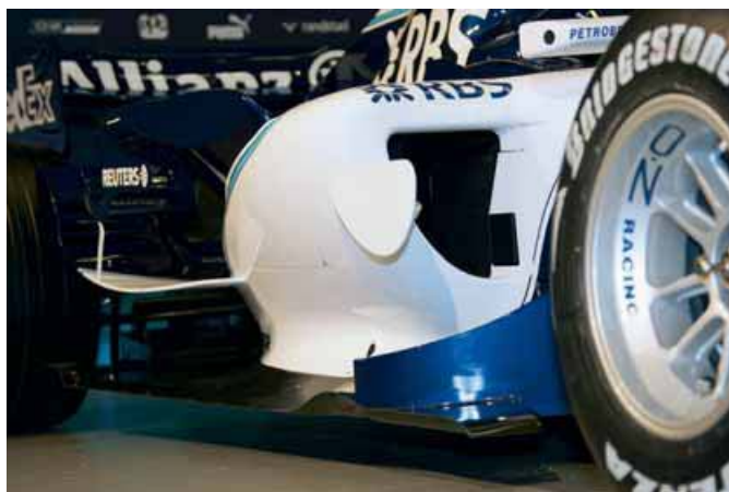
Williams' aerodynamic development is already proceeding at a rapid rate, as alterations to the radiator duct show – left, at the launch, and right, just days later
