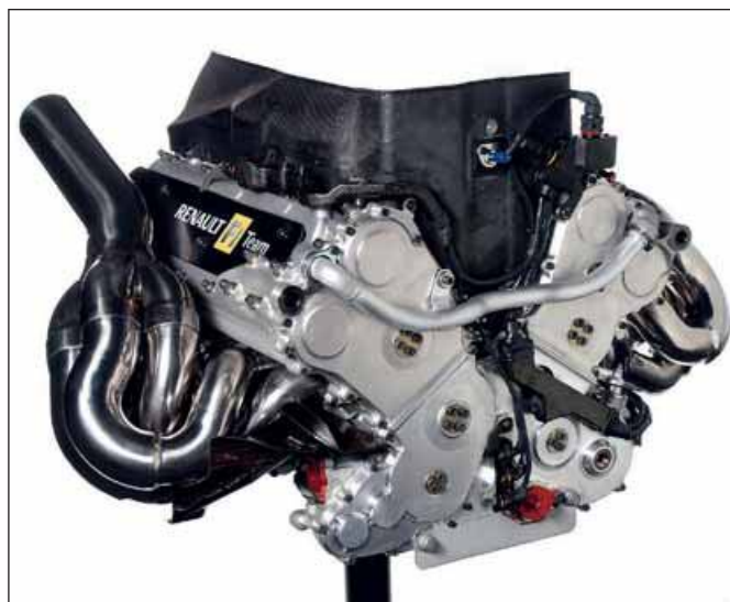
Renault switched to a 90-degree V8 (above) from a 72-degree V10 (below)
