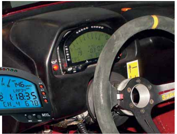
Aim units are available as in-dash displays or as steering wheel versions under the company's MyChron brand. A smaller kart version has also recently been launched
