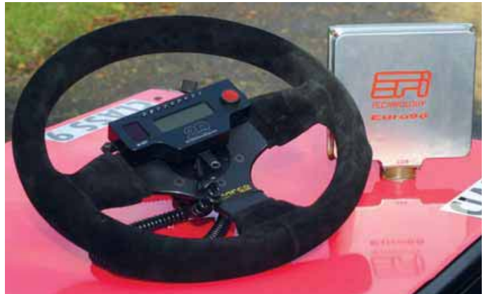
EFI Technology ECU allows driver to switch between maps to suit track conditions
