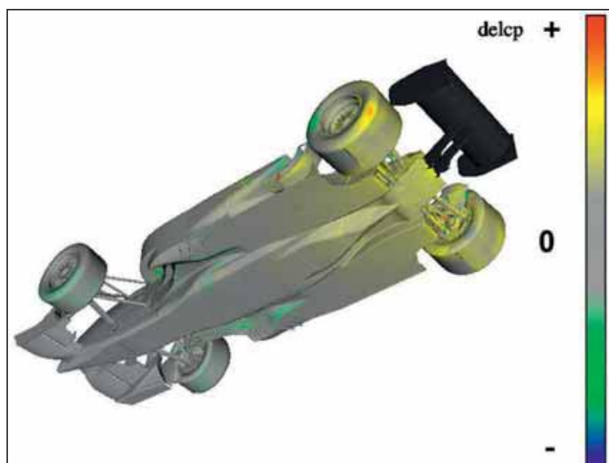
Figure 8: moving the rear wing backwards saw increases in static pressure in the rear underbody, which lost downforce there (Advantage CFD)
