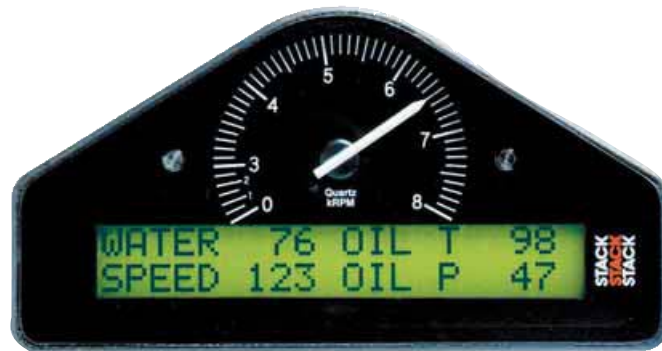
Stack dash displays such as its 8100 (right) are fully programmable yet retain an analogue tach, as it claims most racers prefer it. 8130 series (left) is street unit
