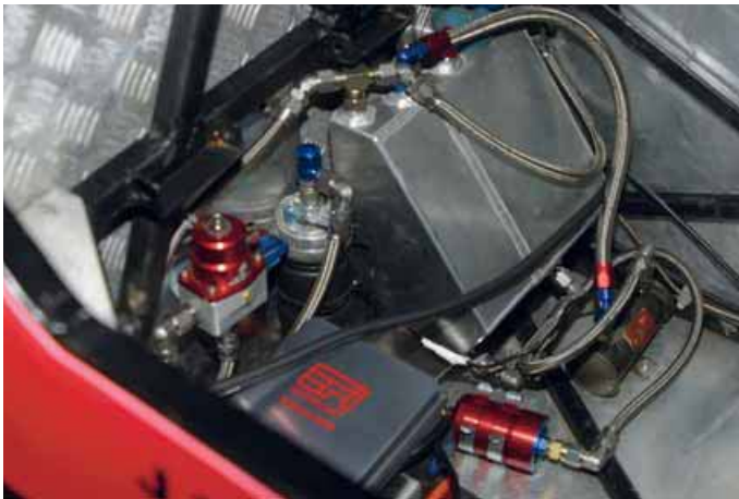
Ancillary components are carefully sited for a low polar moment of inertia
