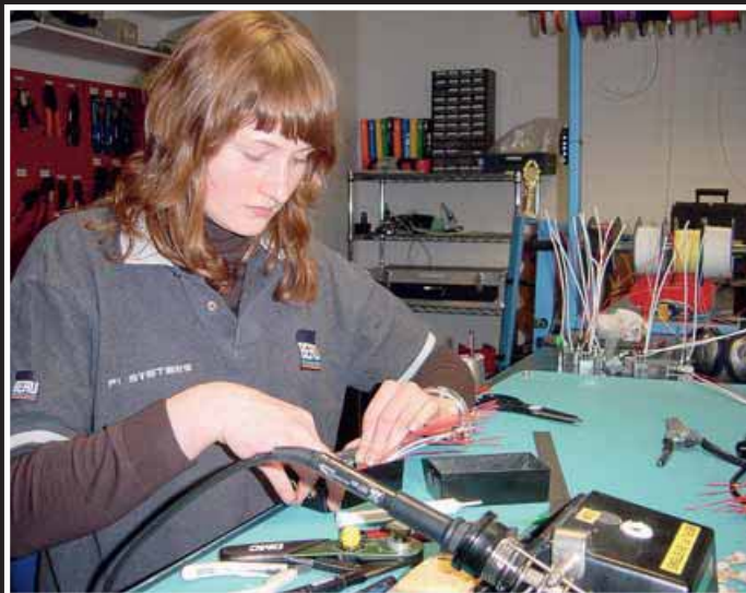
Loom construction is relatively straightforward but requires concentration, some specialist tools and nimble fingers
