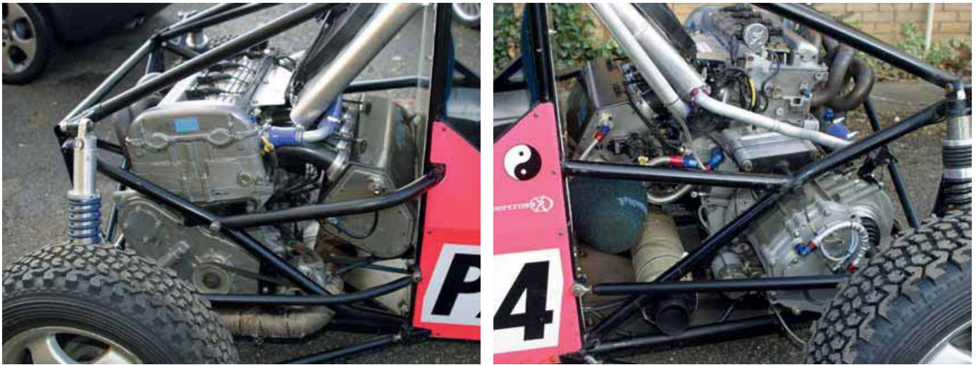
Placement of engine with induction side inboard reduces rearward weight bias. Sodemo engine and Xtrac gearbox are exactly as per BTCC spec Astra, bar the ECU
