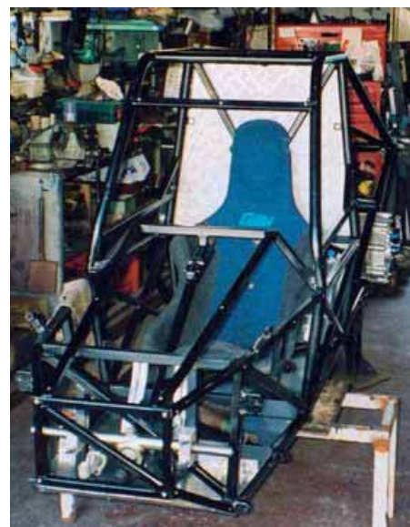
Chassis was mocked-up in wire mesh first to ease placement of components and seating position, then CAD modelled prior to final build
