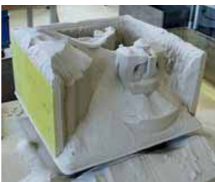
Unsintered sand is poured away leaving the shape of the cores
