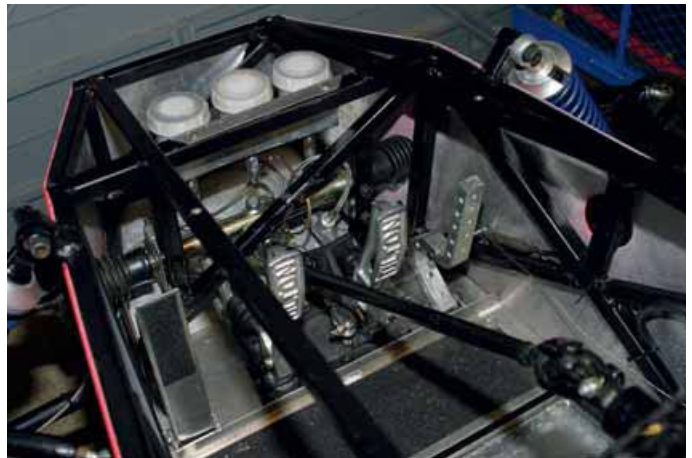
Tilt pedal set and unassisted rack and pinion steering are simple and effective
