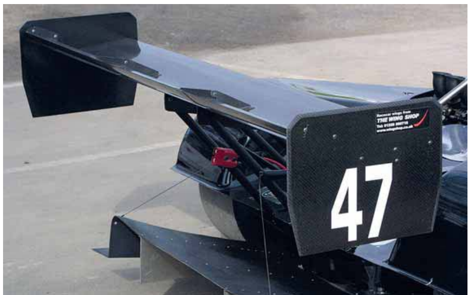
Figure 12: positioning a rear wing to better interact with the underbody can yield gains in downforce (McBeath)
