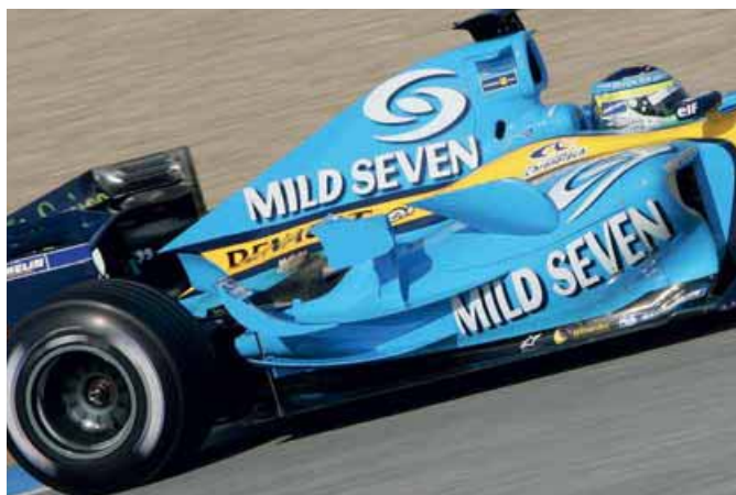
Renault's side pods are roughly aerofoil shaped, with a complex array of winglets and chimneys. Smaller radiator inlet shape is similar to that used by McLaren
