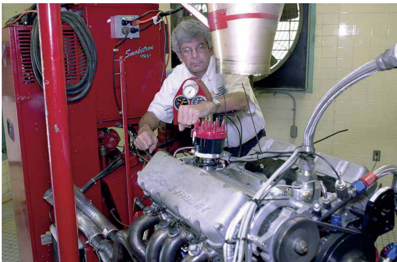
Hoekstra with the Smoketron, the machine Smokey Yunick built to spin test Nextel Cup race engines, donated to the engine optimisation programme in 2000
