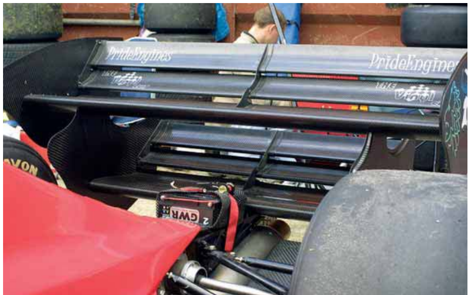
Figure 11: the GWR Predator uses the maximum permitted span for its upper wing tier but the lower tier was kept narrow to avoid the rear wheel wakes (the central battery location was temporary by the way!) (McBeath)
