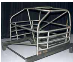
Impact absorbing left-side door bars and a bespoke floor are new for COT
