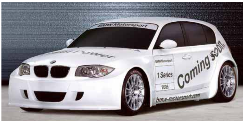
BMW's 1 series – unusually for a passenger car, is reputed to have a roll axis parallel to the ground
