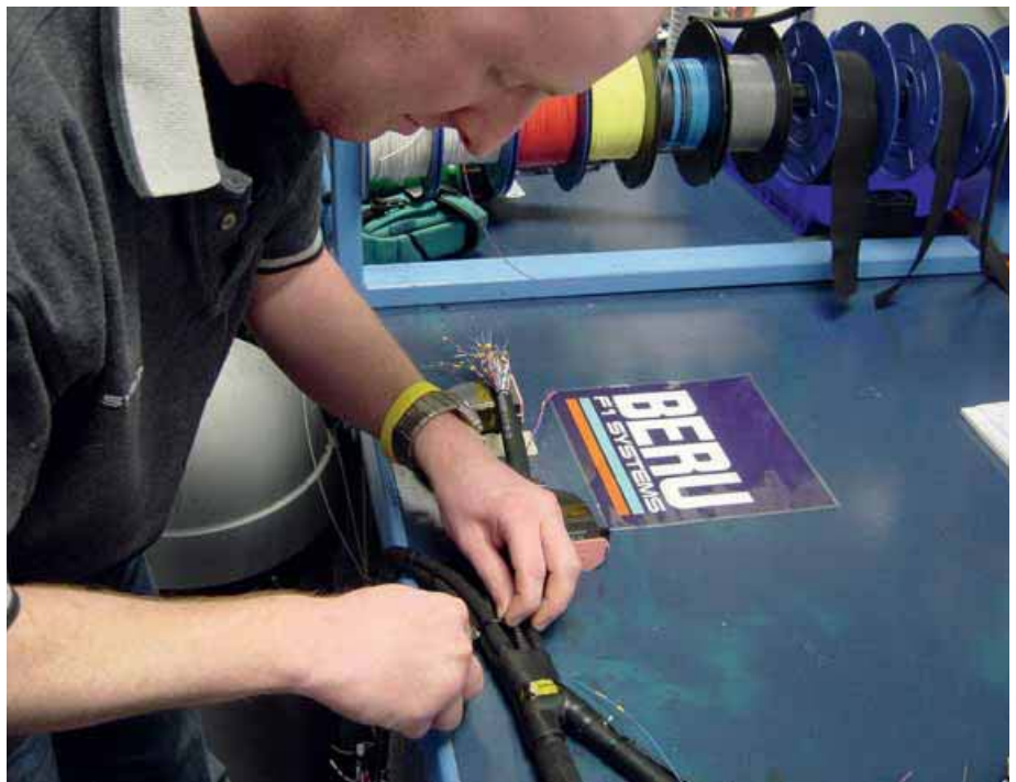
Heat shrinking a finished loom keeps things neat and provides a valuable barrier in a hostile environment
