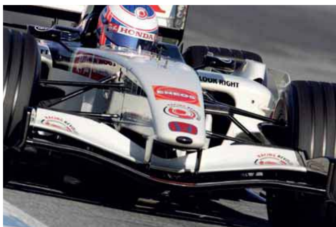
Honda Racing F1 has opted to use a shallow chord front wing this year (left) after the BAR-Honda of 2005 (right) suffered from aerodynamic problems
