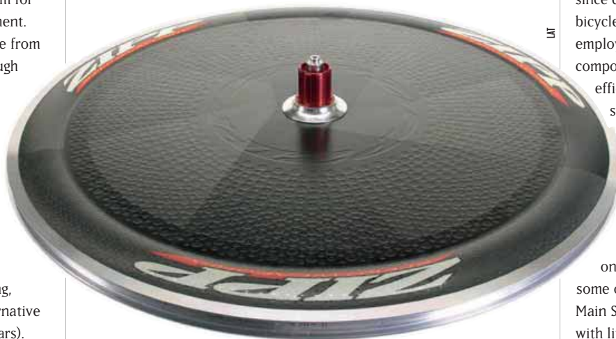
Zipp's latest bicycle wheel has a concave bulge to re-capture and control airflow coming off tyres of various widths. Dimple size and density varies by location around the disc relative to air velocity
