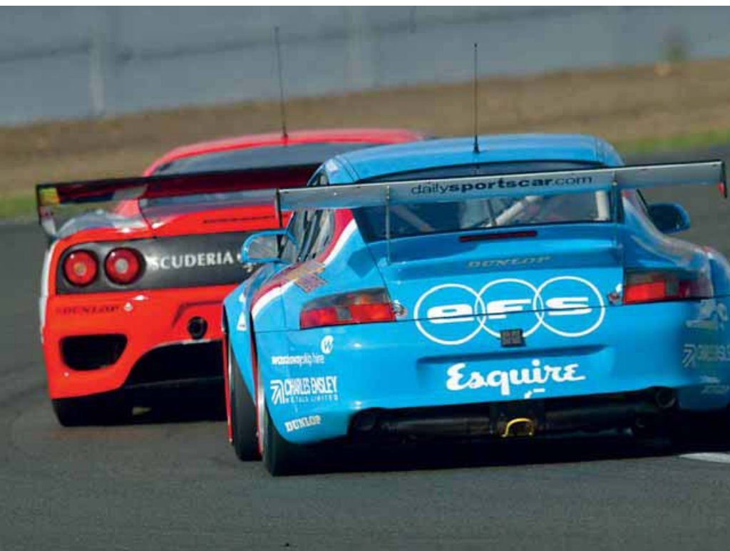
GT and touring car regulations force rear wings to be masked by the body making them much less efficient
