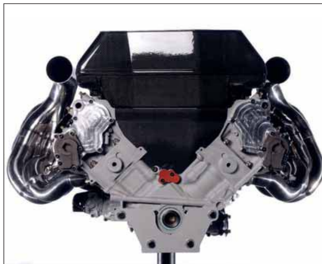
Renault switched to a 90-degree V8 (above) from a 72-degree V10 (below)
