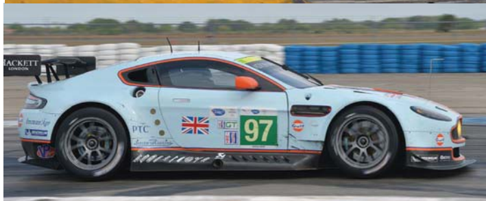
The new GTE model features brand new side sills, added to counter the problem of having the exhaust running down the side of the car
