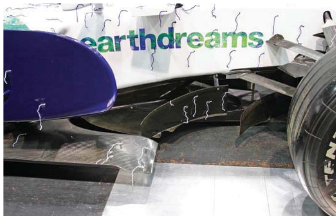
Photo 2: removing the bargeboards from the Honda RA107 had a massive effect on downforce
