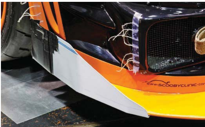
Sealing the end fences to the wheel arches increased the effect
