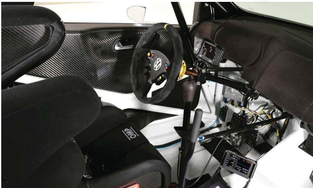
The Polo R cockpit. Drivers have a four-position map switch to help VW engineers to tailor the car to rallying conditions
