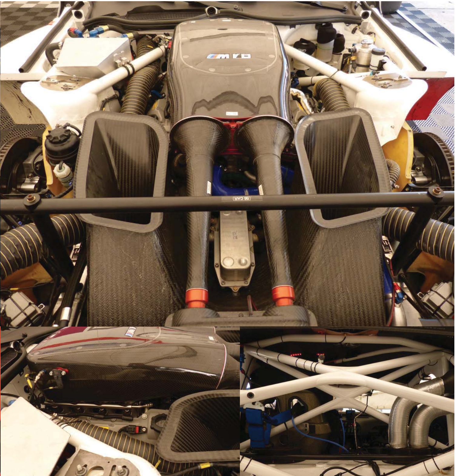
The changes to the engine concerned the switch to a sonic restrictor
