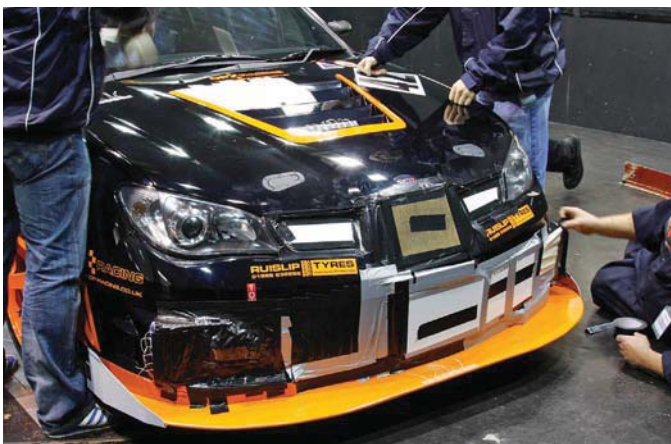
Blanking off the front apertures had a significant effect on front downforce
