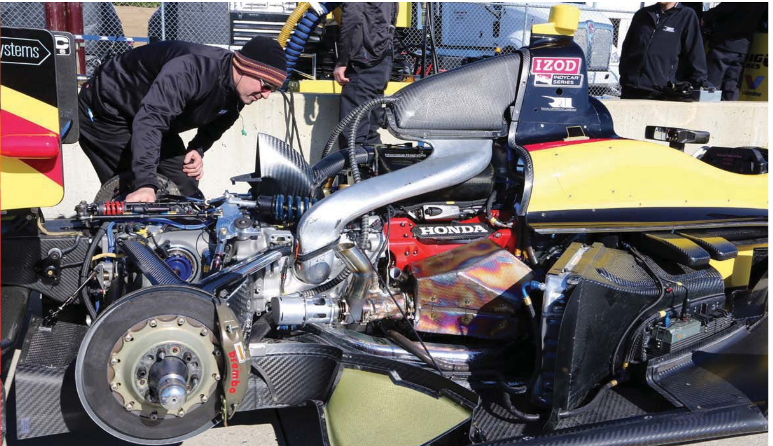
IndyCar is taking advantage of the progress made by fuel companies seeking 500 bar pressure for F1 to increase DI pressure to 300 bar in 2013
