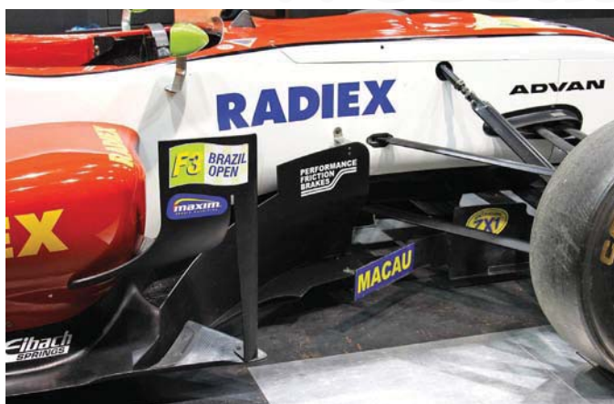
Photo 3: bargeboards and vortex generators proliferated in many single-seater categories; this is the Dallara F308 in 2011 specification
