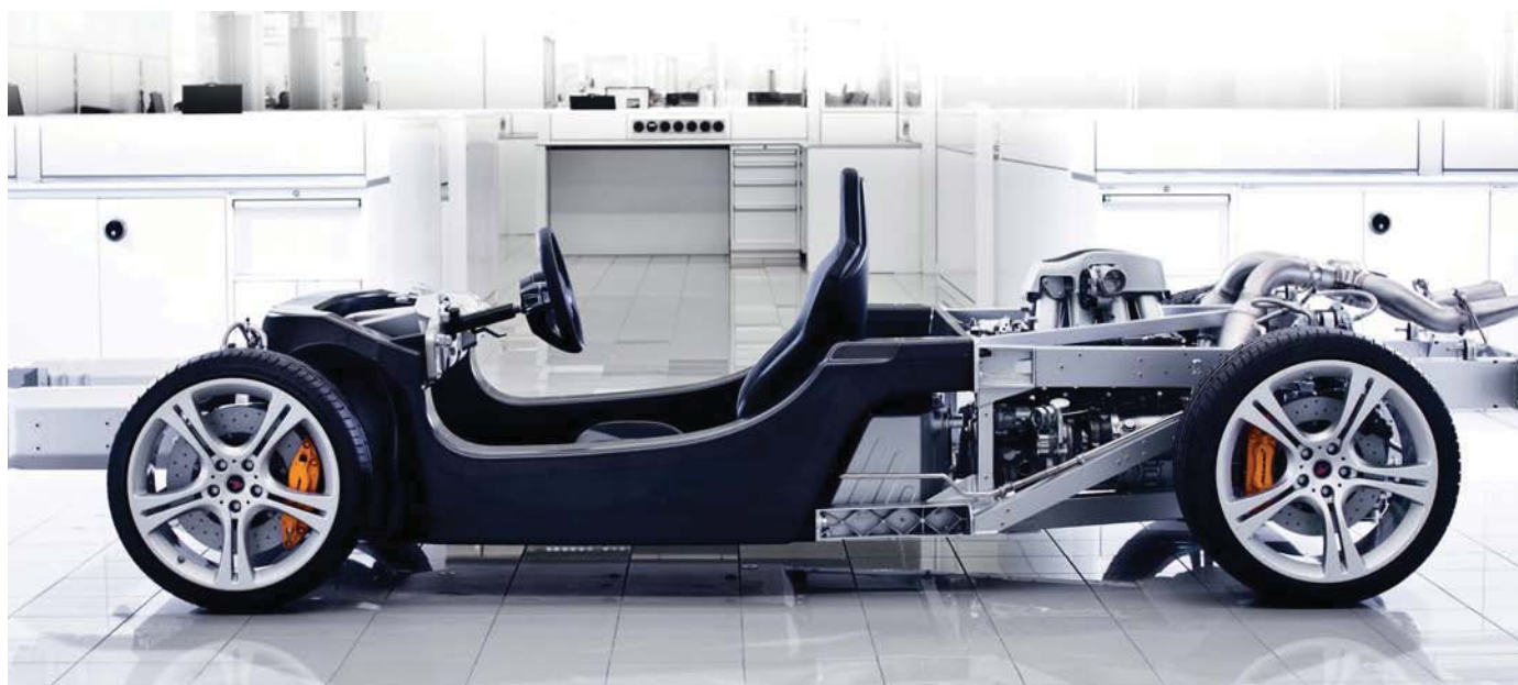
With the outer body panels removed, it is obvious how the carbon-fibre MonoCell integrates into the McLaren MP4-12C road car chassis
