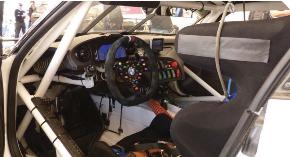
BMW had to change the driver seat to aid quicker pit stops, and introduce air conditioning to meet regulations
