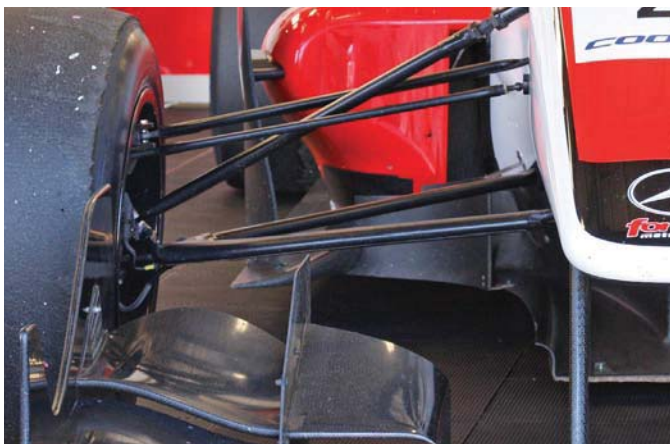
The pushrod going to the upright on the Dallara F312
