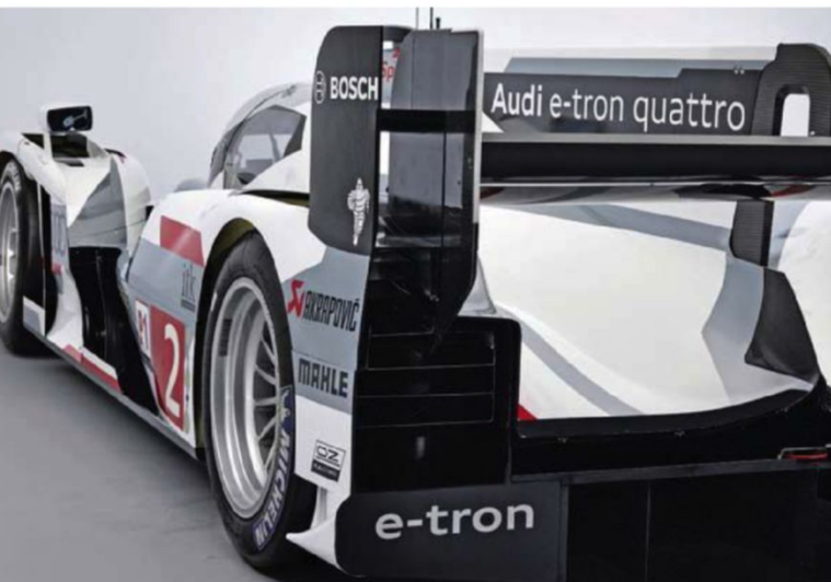
Audi is believed to be playing with the air pressure behind the rear wheel to reduce drag (see separate feature).
