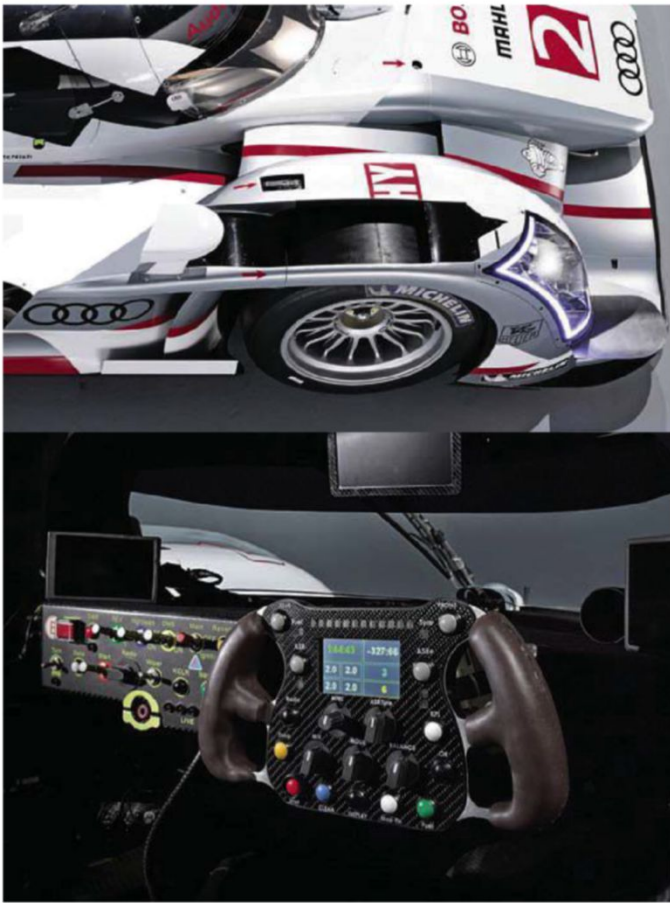
Audi has introduced screens to the cockpit linked to a roof-mounted camera to help with forward and rearward visibility
