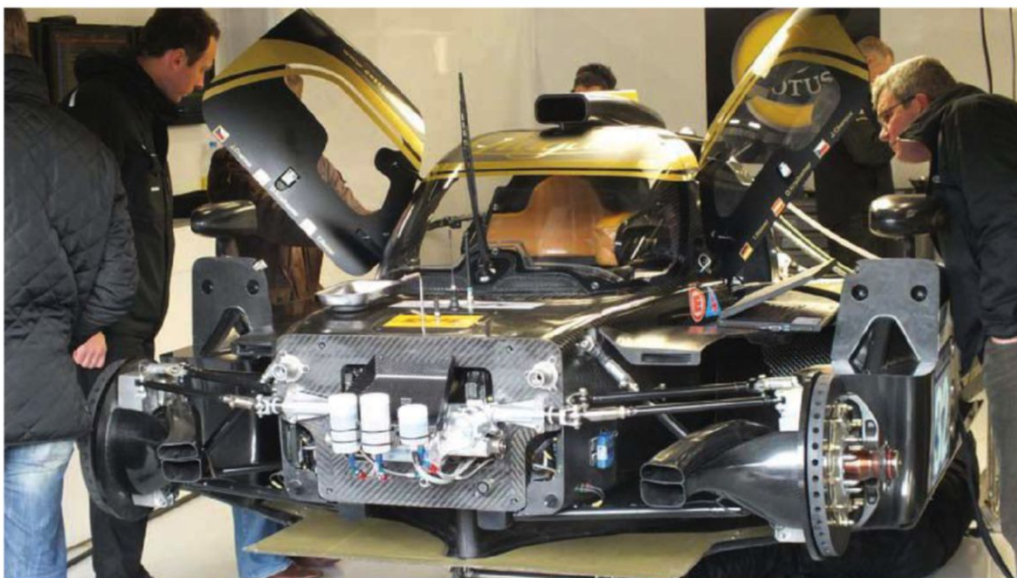
The Lotus features torsion bar front suspension, not seen on an LMP2 design since the Porsche RS Spyder
