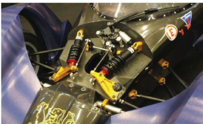
Quality-name components on the new Praga include Koni dampers, Cosworth ECU, a ZF Sachs clutch, Hewland JFR gearbox and AP Racing brakes
