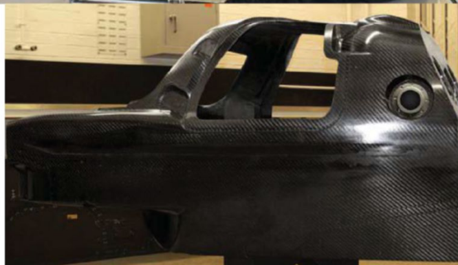
Bodywork consists of carbon sandwich composite panels, with quick release nose, rear diffuser, wheel arches, rear end and rear wing
