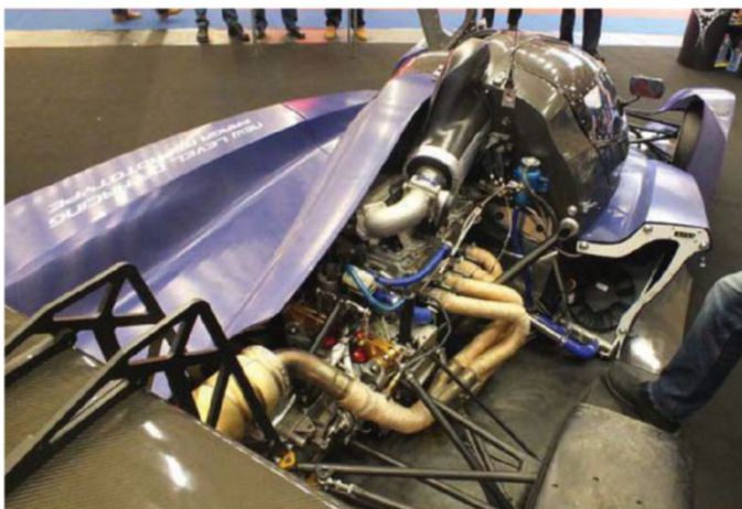
The R1 features a Renault Sport Formula 2.0 engine, capable of 210bhp, although Praga has a 532bhp Suzuki Hayabusa-based model in development
