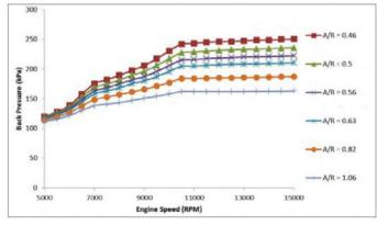
Figure 6: engine back pressure for different turbines on a 2014 F1 engine
