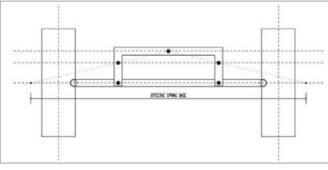
View of the spring base on the proposed warp-soft interconnected suspension
