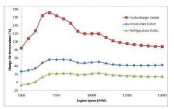
Figure 9: charge air temperature overview
