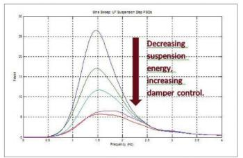
Figure 4: (above) acceleration plot for a racecar
