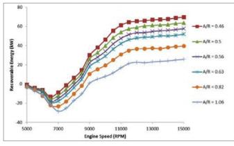
Figure 5: recoverable exhaust energy for turbines on a 2014 F1 engine
