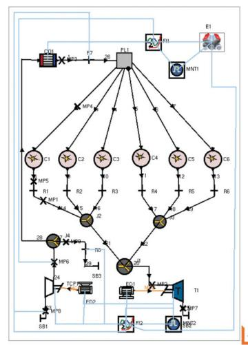
Figure 4: AVL Boost 2014 Formula 1 engine model
