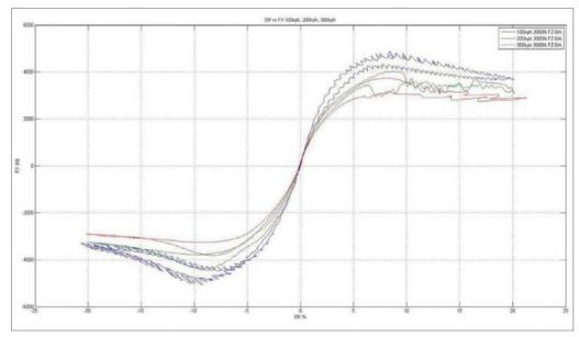
Figure 3: slip ratio and speed sweep results
