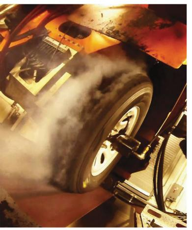
Figure 2: slip ratio test
