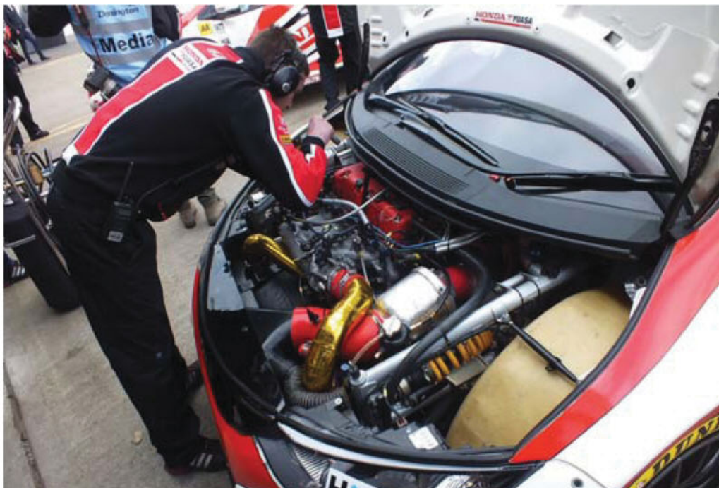
The Civic Tourer features a production-based 2.0-litre inline four engine developed by Neil Brown Engineering
