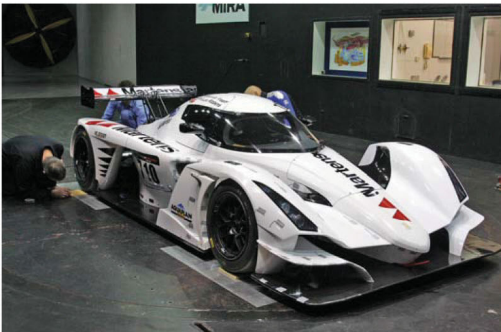
Inserting shims under the Praga R1's tyres to alter ride height
