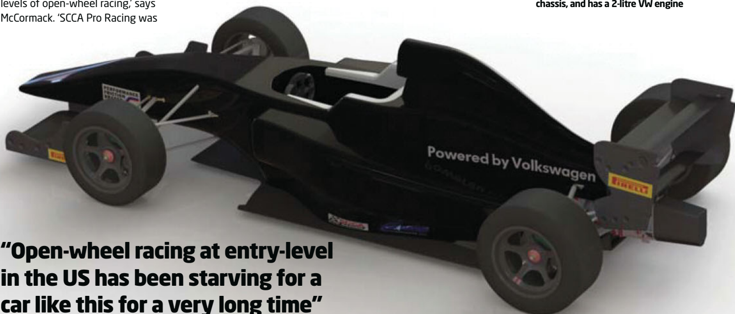
The FL15 features a carbon composite chassis, and has a 2-litre VW engine
