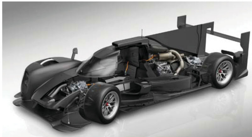
Above: highlighting the MGU-K (front) and MGU-H (rear) on the 919 Hybrid, and how they connect to the li-ion battery. The front generator is operated as a single electric motor and drives the front wheels via a differential. This gives the car a temporary all-wheel drive system
