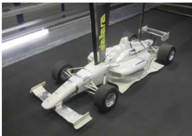
A scale model of the IL-15 in the Dallara wind tunnel facility in Parma, Italy
