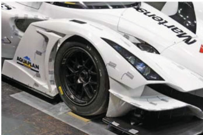
The effect of rake was assessed by dropping the front back down to +10mm
