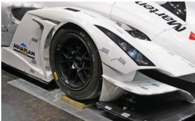
The maximum ride height increase was 24mm at front and rear
