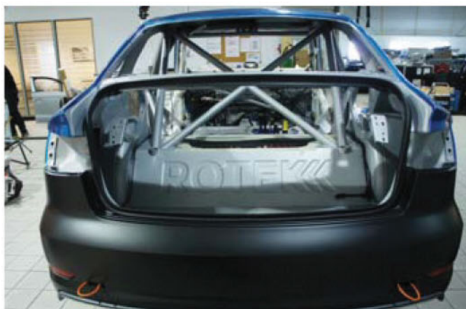
The rollcage is mated to a heavily modified production car shell, which was prepared by Willy Poole Motorsport Services
