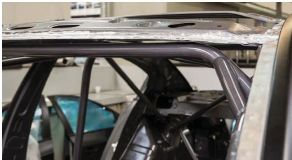
An issue with a bar across the top of the windscreen resulted in a delay to the first shakedown of the car
