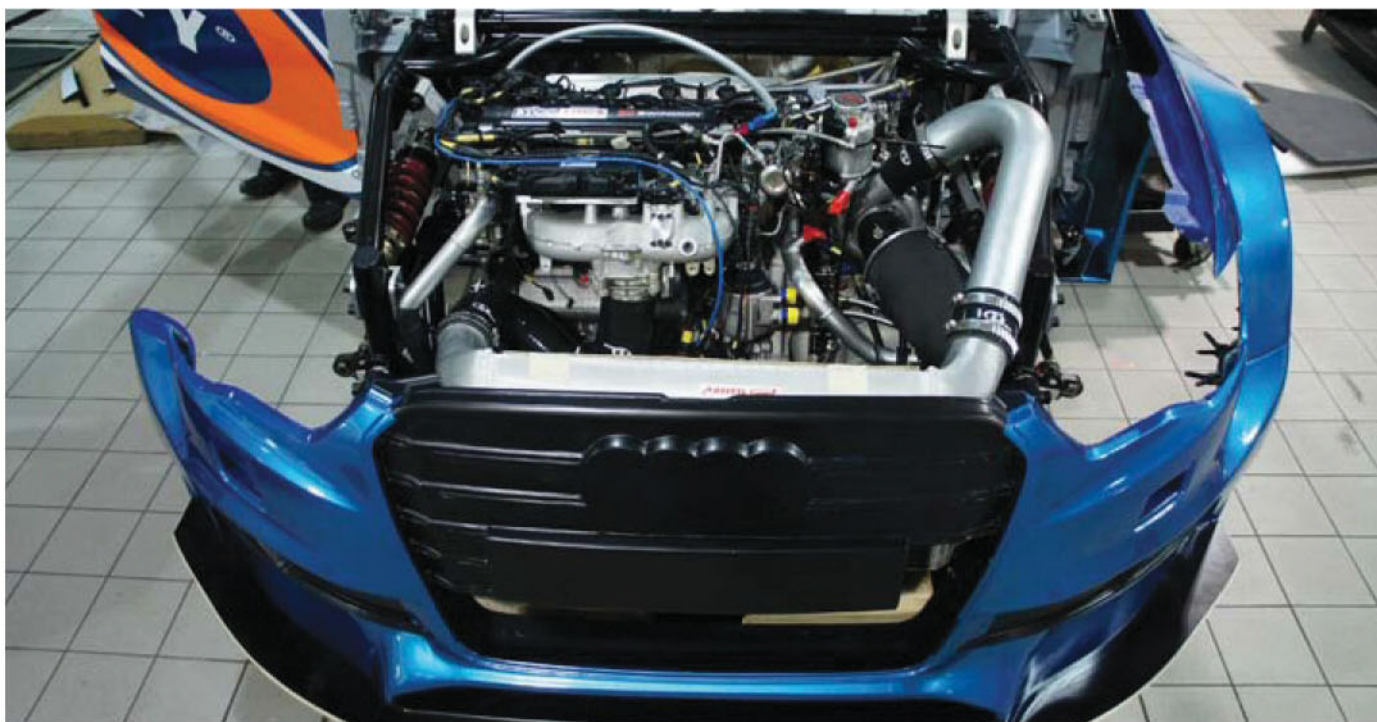
Rotek opted for the spec Vauxhall-based engine, supplied by TOCA and tuned by Swindon Racing Engines
