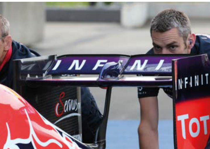
Rear wing set almost flat, Red Bull found some speed at the expense of downforce...
