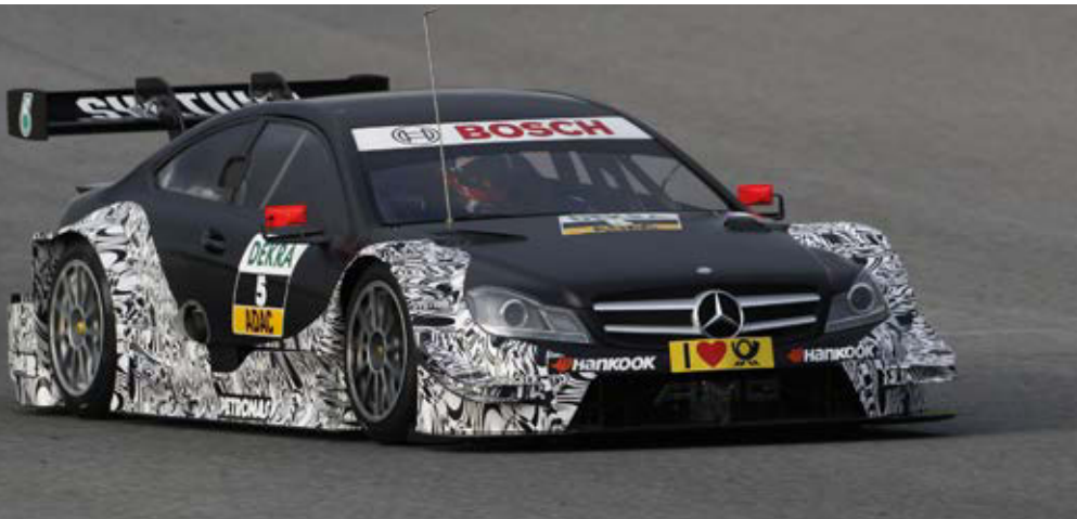
Mercedes livery in testing serves to indicate the body areas of the cars that are allowed to deviate from the base car template. Dazzle camouflage may be to deter eyeball analysis of aero elements by opposition
