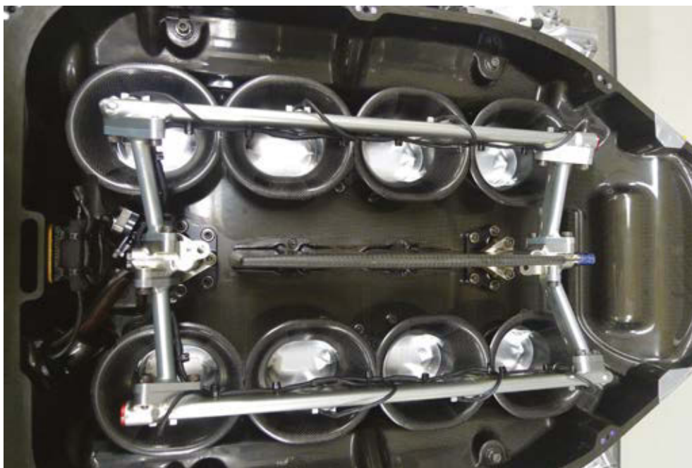
Power gains were found from creating a splitter between the left and right bank of intakes in the V8 airbox
