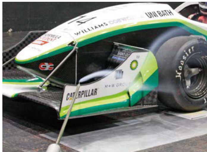
Figure 8: The front end plates also deflected air around the outside of the tyres
