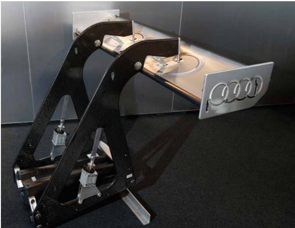
The 2014 regulations allow for DRS on the rear wing but, as currently implemented, the added cost and complexity hasn't yet delivered closer racing or more overtaking
