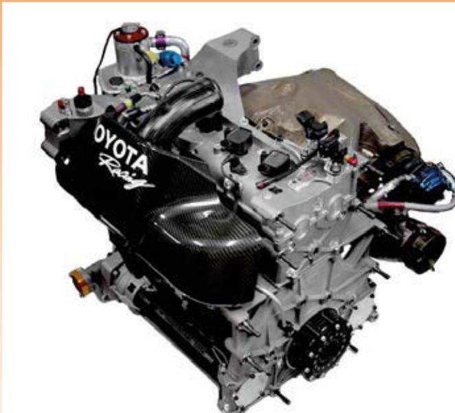
GT500 in Japan initially ran with 3.4-litre V8s but, for 2014, GTA rules demand 2.0-litre turbocharged four cylinder powerplants like this Lexus unit
