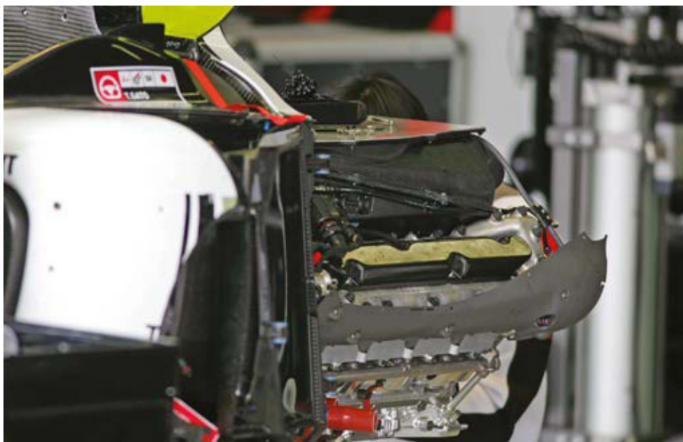
'Third Era' engines, such as this 2005 unit, were more compact and almost 50 per cent lighter than their predecessors
