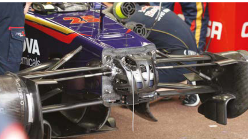
Bulkhead arrangement of the STR9 features a fairly conventional pushrod front suspension. Turning vanes and brake shroud assemblies are also visible in this shot
