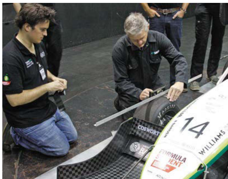
Figure 6: Setting up the trip strips on the front tyres
