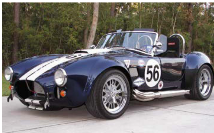
Some limitations of a live axle Cobra replica can be overcome, but resultant rear wheel movement is not identical to the IRS of the original
