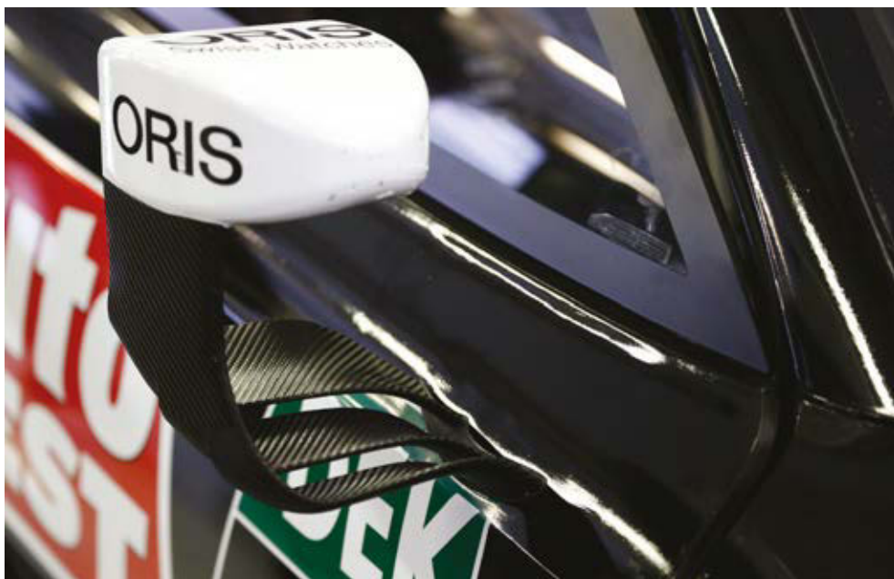
Aero door mirrors highlight a small free area in the extensive DTM regulations for the upper parts of the cars
