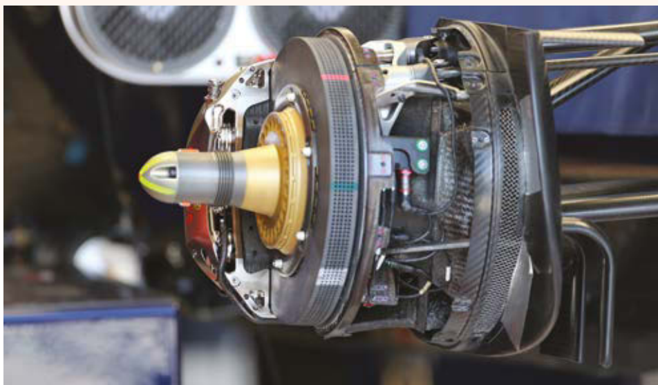
Top: Brembo componentry features in the STR9's brake by wire system. Three-row ventilation drilling visible on rears
