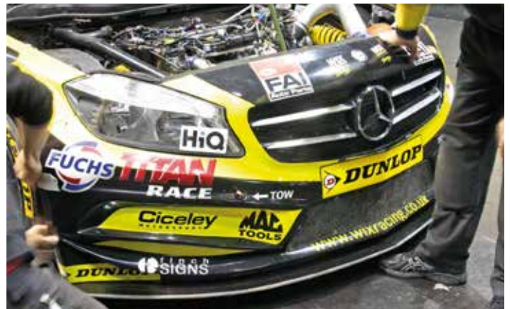
Photo 2: The original front bumper featured a horizontal recess above the splitter
