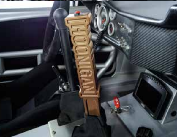
The 'Hoon Handle' is a specially developed handbrake which not only locks the rear wheels but also disconnects drive to the rear. It was originally developed for Block's rallycross Supercar. Note the traditional looking Auto Meter dials supplemented by a MoTeC digital dash
