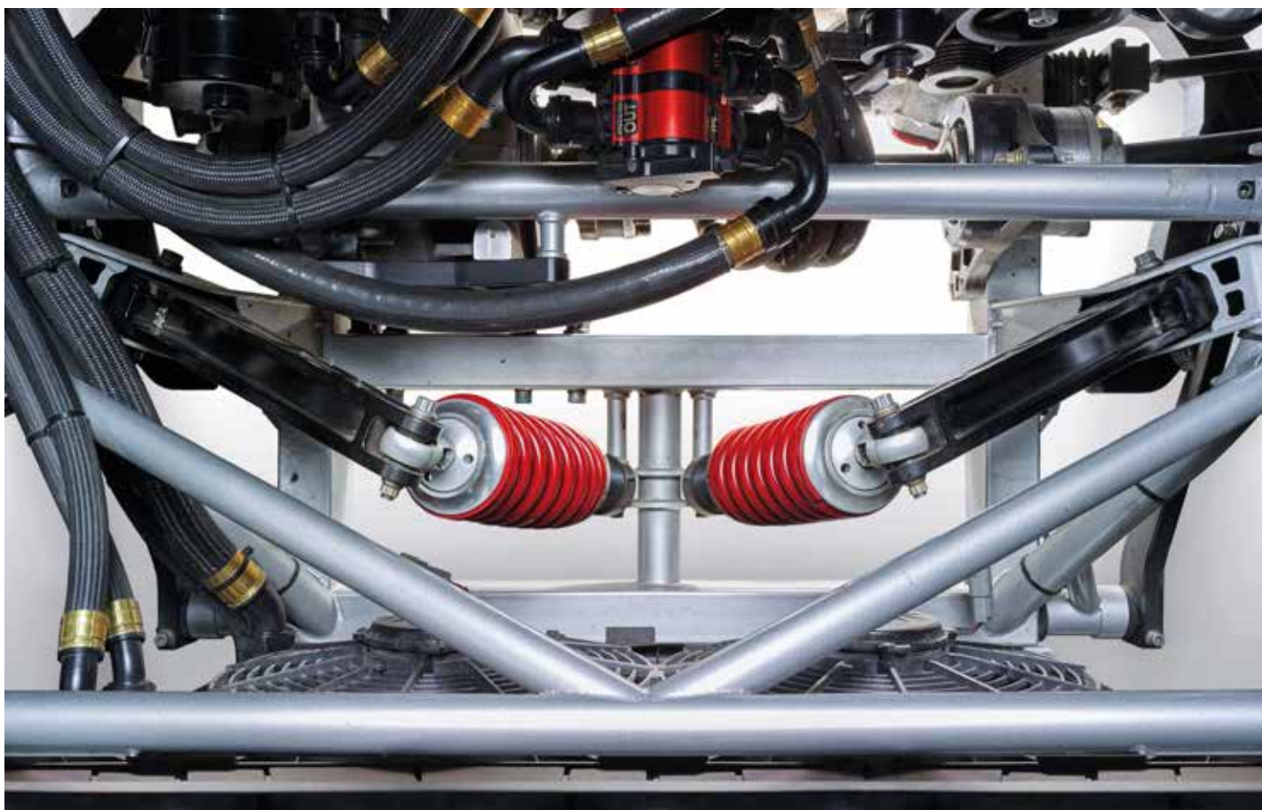
Above: The large engine and Dakar transmission saw the '65 Mustang chassis replaced with tubular steel, as is evident under the bonnet of the car. Note positioning of J/Ri dampers Left: A cantilver suspension system was fitted front and rear to meet the dual demands of Gymkhana filming and real world competition
