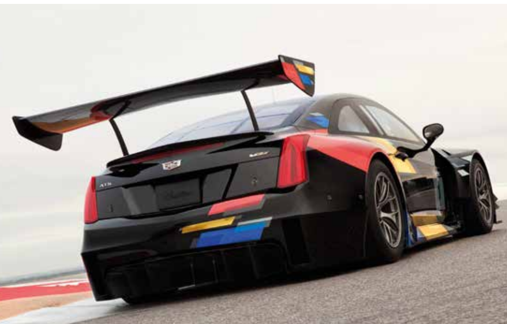
A full-length undertray directs air beneath the car to the rear diffuser, which helps create a downforce-producing effect and keeps the 18-inch racing tyres planted securely to the track
