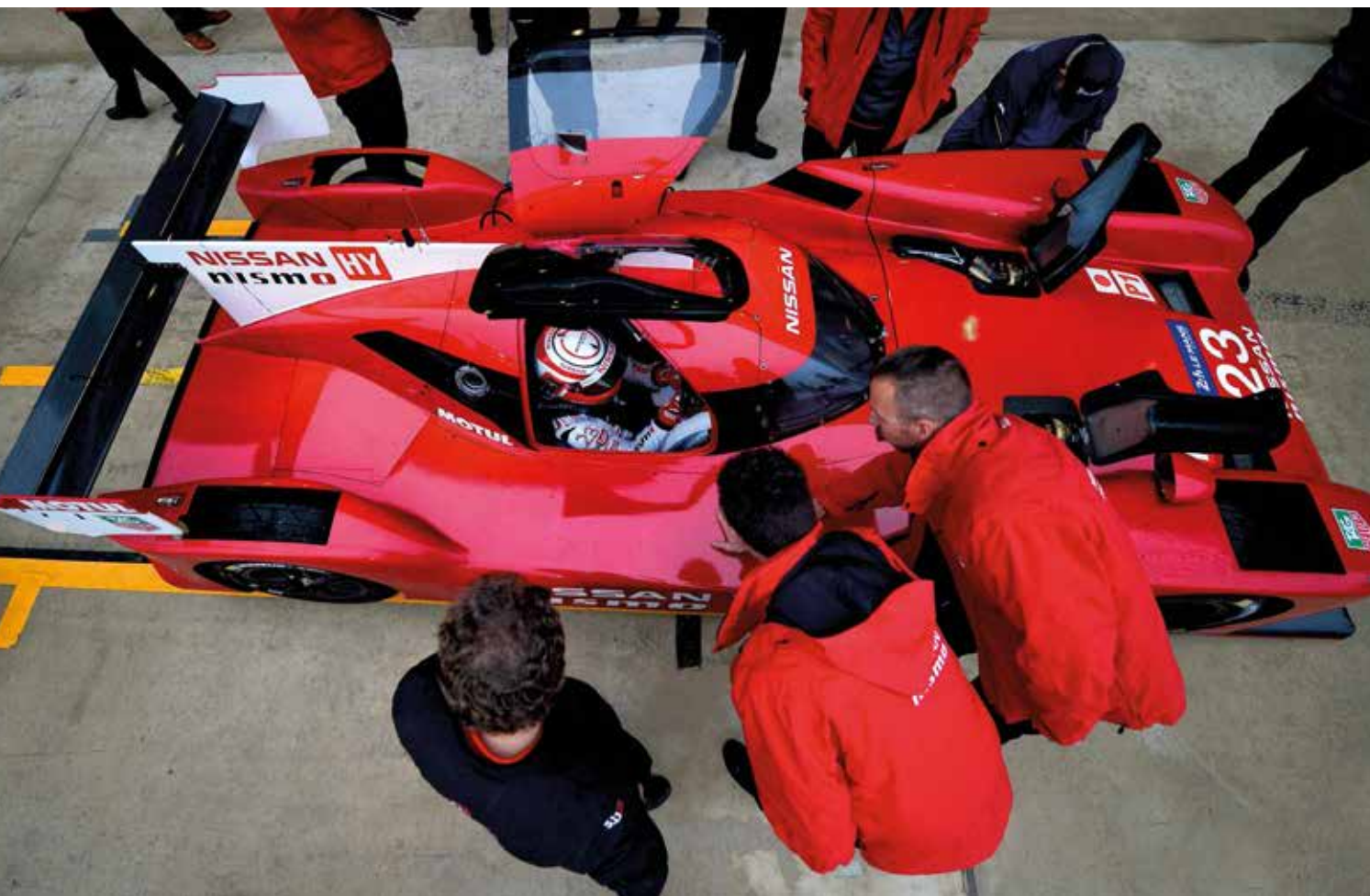
Nissan has challenged conventional thinking with a front-engine car. One of the two turbos is visible in the opening by the front wheel, confirming a twin-turbo layout
