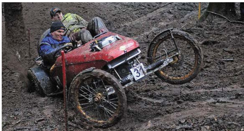
In trials the passenger can play an important role as anti-squat in boosting grip and traction when attacking hills
