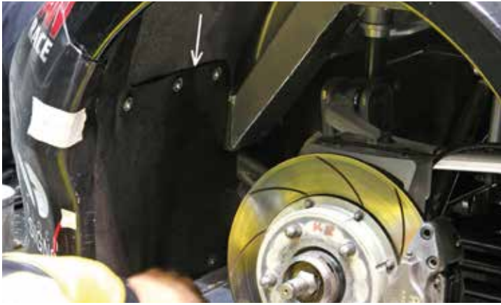
Photo 5: The panel closing off the rear bumper cavity produced the expected results
