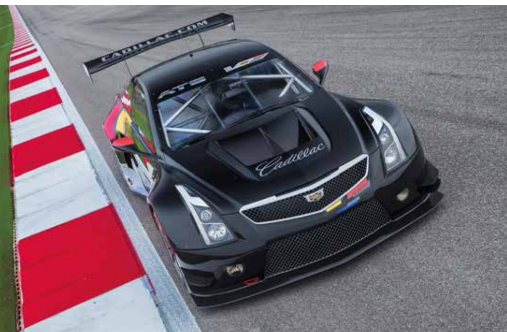
Thanks to the larger twin BorgWarner turbochargers, a direct, side-exiting exhaust system and larger capacity intercooler, the ATS-V.R’s 3.6-litre twin-turbo V6 powerplant produces up to 600bhp at 7400rpm
