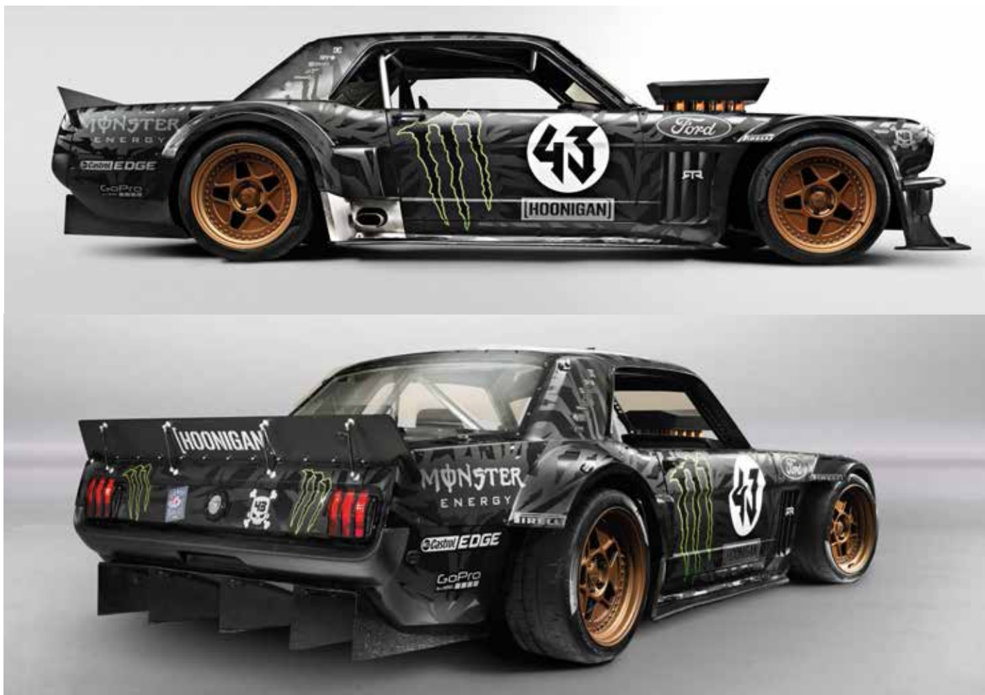
The bodywork of the 'Hoonicorn' was originally fabricated in metal before moulds were taken and made in composite materials, only a few panels of the original '65 Mustang remain. Some of the aerodynamic elements of the bodywork such as the diffuser and NASCAR style spoiler are fitted more for show, but could be reworked ahead of competition
