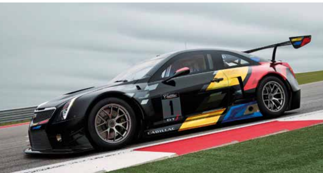
The carbon fibre aero package features an aggressive rear diffuser, a front splitter, dive planes and rear bumper cover, all of which have been designed to fit FIA-mandated tyres and wheels
