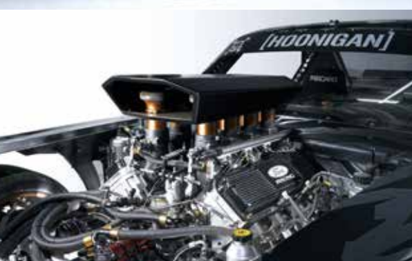
The huge Roush-Yates Sprint engine produces almost 900bhp and sits as far back as possible due to aesthetic demands rather than for vehicle dynamic reasons
