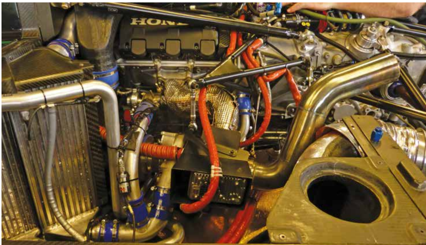
The 2.8-litre twin-turbo V6 powerplant uses more than 400 production parts for improved reliability – the technology is proven and has won multiple championships
