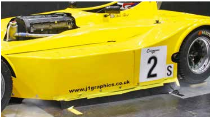
By whatever mechanisms, on this flat bottomed car with no rear diffuser, side skirts provided useful benefits with a modest increase in downforce and a decrease in drag
