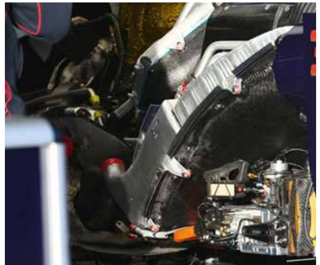
Toro Rosso has crammed the intercoolers plus the water coolers for the Renault V6 engine and its energy recovery system into its sidepod. In this picture the intercooler is clearly visible. The cooling is a central design theme with STR10
