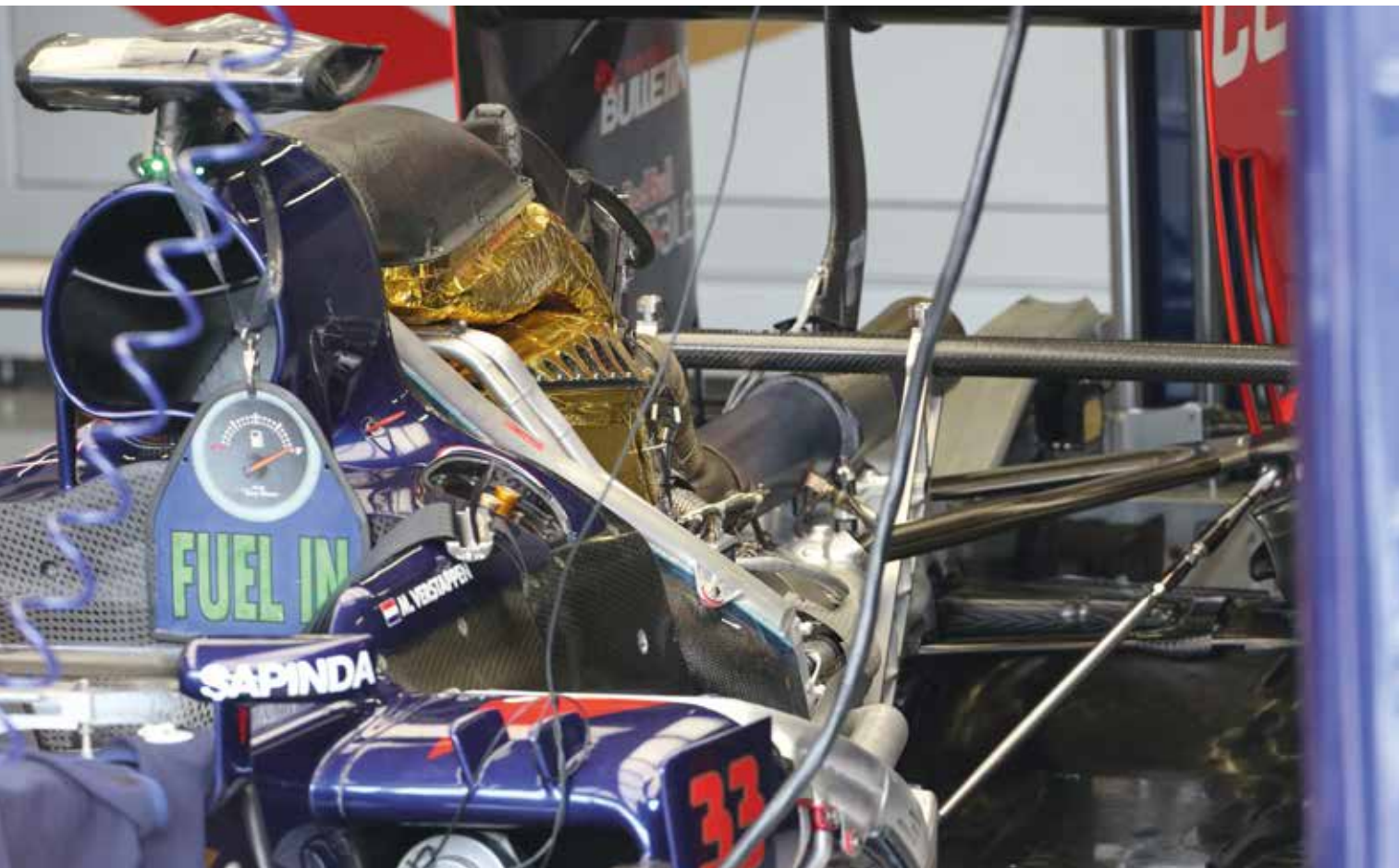
Above: The back of the car is tightly packaged and Toro Rosso is now focussing much of its development on the STR10's rear. The wing support actually passes directly through the tailpipe Below: The STR10's front bulkhead is pretty conventional as is the rest of the pointy end, featuring torsion bar front suspension. The assisted steering rack is manufactured by the team
