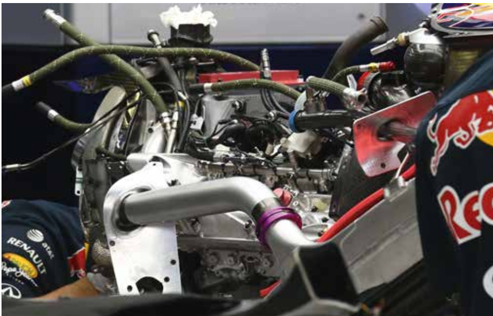
The top of the V6 power unit with the plenum removed. This year Renault switched to a variable inlet and this is one of the major differences between last year's unit and the 2015 engine – these were not allowed in Formula 1 during 2014 season
