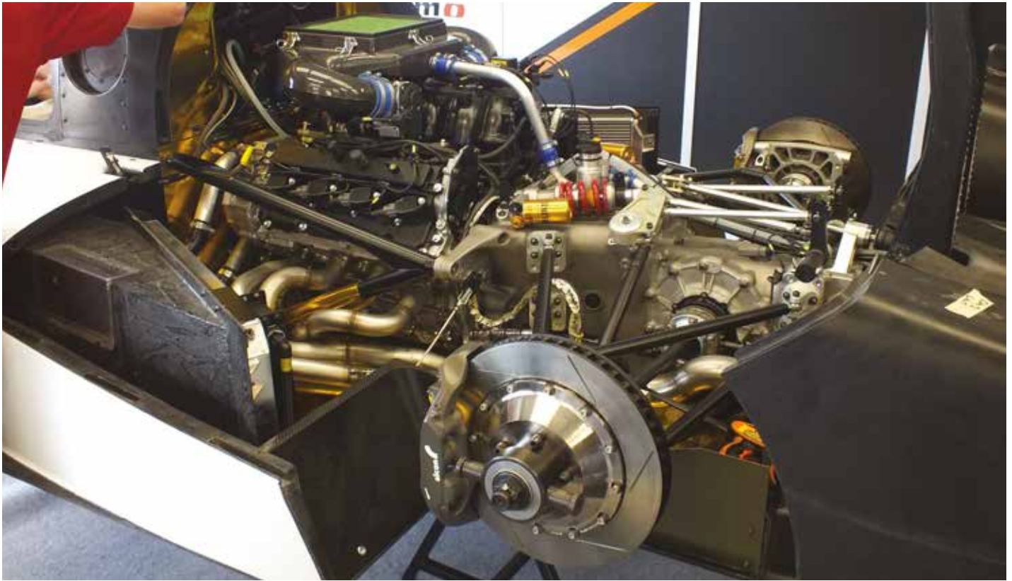
LMP3 cars must use this 420bhp normally-aspirated 5-litre Nismo Nissan V8 engine prepared and supplied by ORECA. The gearbox is a 6-speed sequential unit supplied by Xtrac
