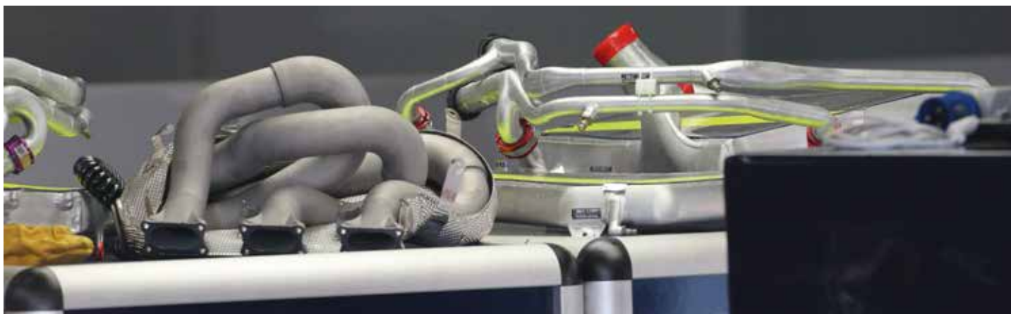
Above: The exhaust header with heat shielding removed – it appears to have been treated with a ceramic coating to further protect against heat Left: The Friday press conferences on grand prix weekends have sometimes been uncomfortable occasions for Renault boss Cyril Abiteboul this year
