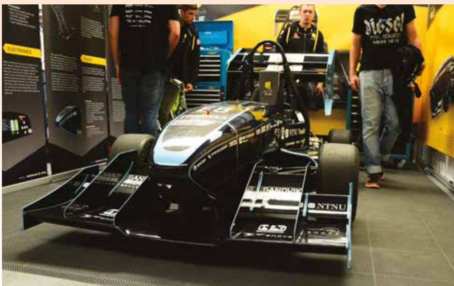
Bespoke electronics packages seem to be a growing trend in Formula Student. The NTNU car featured a team-built Battery Management System (BMS) which enabled it to monitor the current and the temperature of each cell pair
