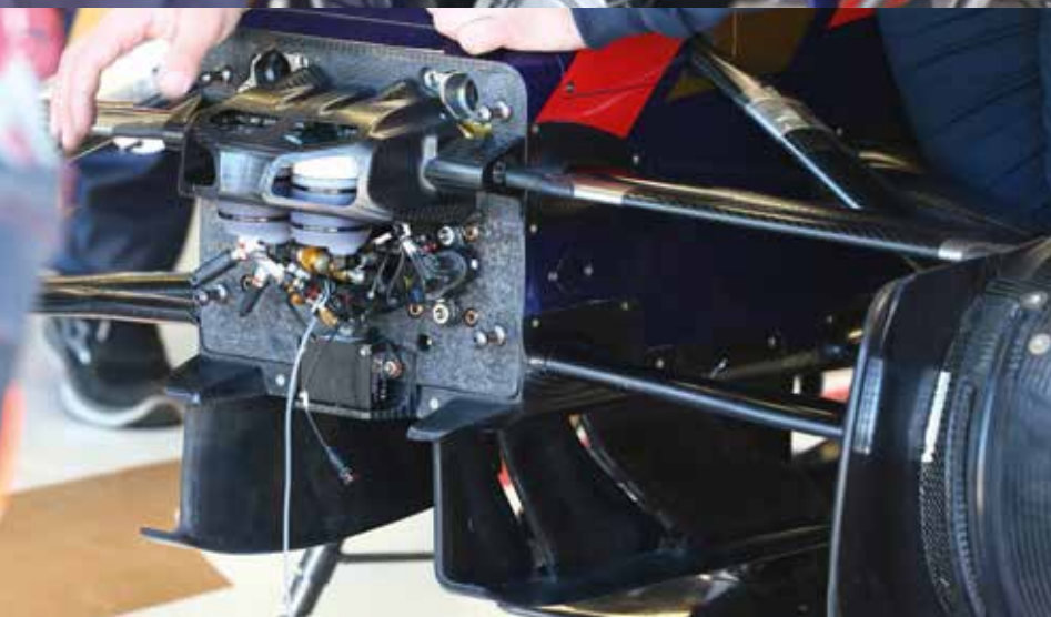
Above: The back of the car is tightly packaged and Toro Rosso is now focussing much of its development on the STR10's rear. The wing support actually passes directly through the tailpipe Below: The STR10's front bulkhead is pretty conventional as is the rest of the pointy end, featuring torsion bar front suspension. The assisted steering rack is manufactured by the team
