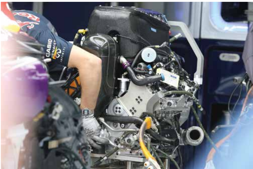
A shot of the V6 engine in its entirety. The MGU-K is visible, as is the turbine inlet and oil tank – the latter of which is a carry over from the 2014 powerplant. The engine is actually officially named the Energy F1-2015, but most call it the RS34
