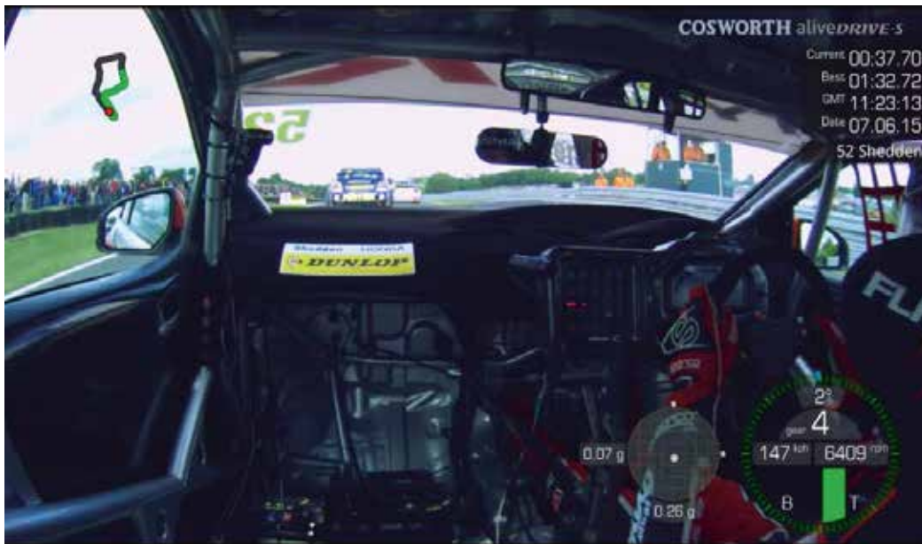
The camera needs to capture the steering inputs of the driver so it's usually mounted on one of the rollcage cross members
