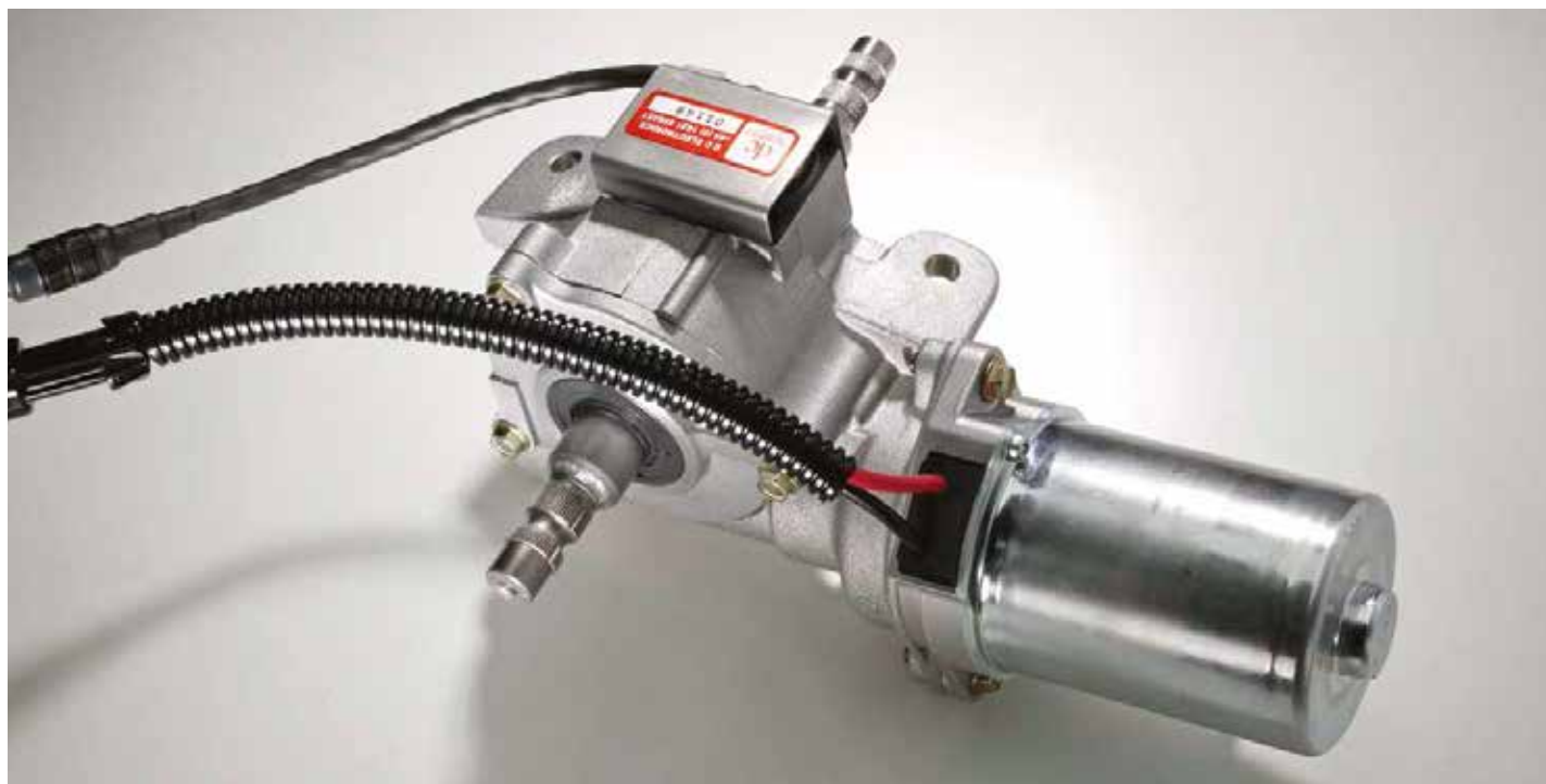
A typical column-mounted steering assist unit – the ability to mount on the column is an advantage of EPAS over hydraulic
