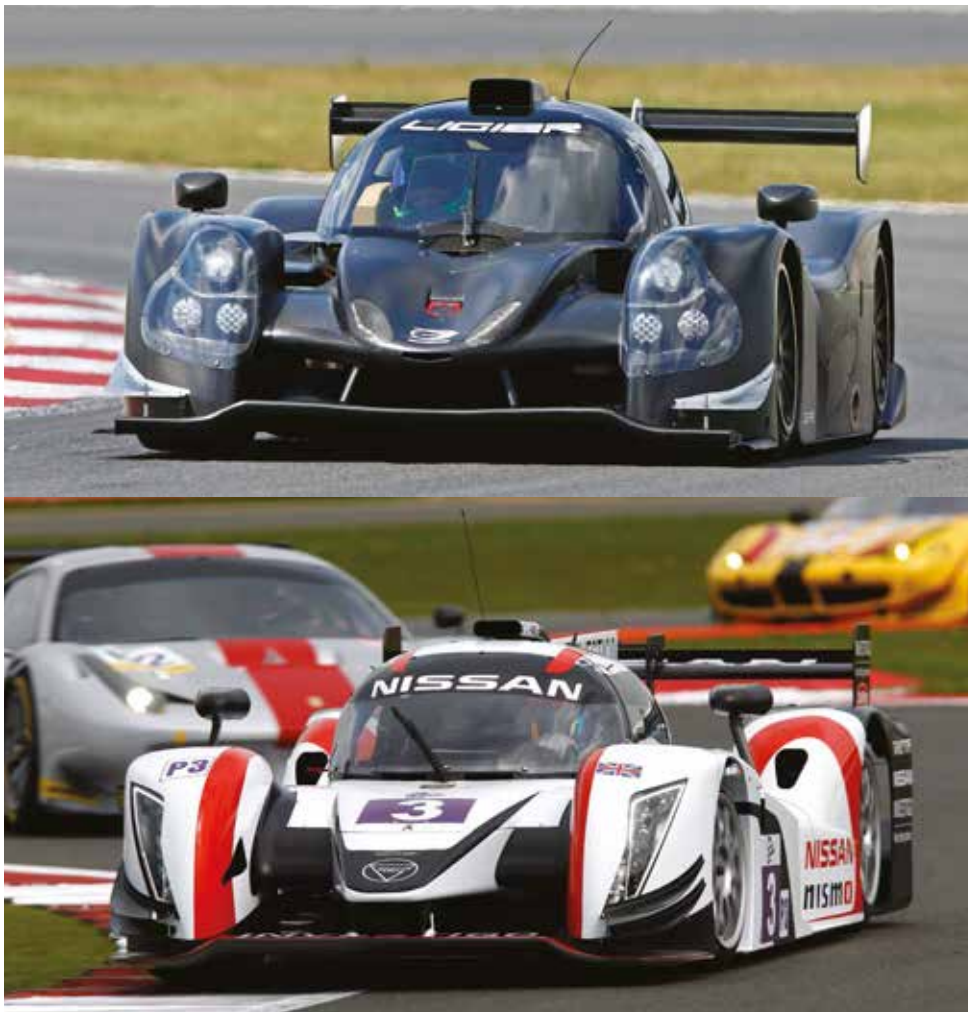
Top: Onroak used its LMP2 experience to bring the Ligier JS P3 in under the weight limit. The aerodynamics of LMP3 cars are similar to LMP2, with bodywork openings above the wheels and a single element rear wing. Above: One of the main criticisms aimed at LMP3 has been its lack of pace when compared with GTE cars. Pictured is the Ginetta-Nissan LMP3
