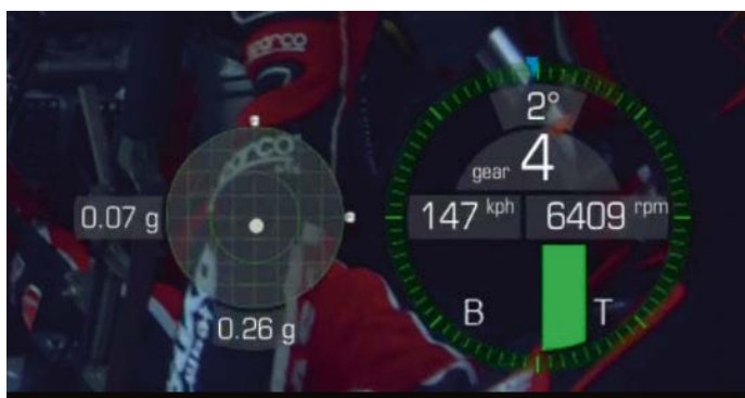
Everything the driver and car does is logged on the graphical data display, including steering angle, throttle opening, brake pressure, the car's speed, engine revs, etc.
