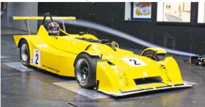
The Classic Clubmans Mallock Mk 18B sporting 'low downforce' nose with Gurneys
