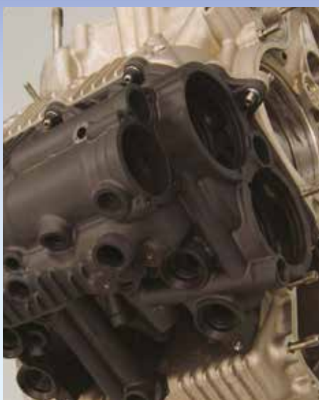
Complex shapes can be 3D printed using the Windform materials and be good enough to use as production parts
