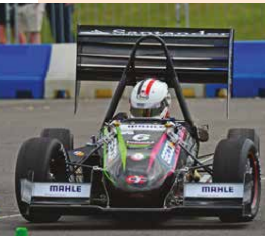
Upper cascades on the rear wing of the Oxford Brookes entry were to help balance out the front-limited racecar
