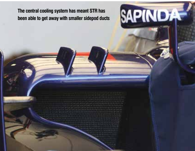
Toro Rosso has crammed the intercoolers plus the water coolers for the Renault V6 engine and its energy recovery system into its sidepod. In this picture the intercooler is clearly visible. The cooling is a central design theme with STR10
