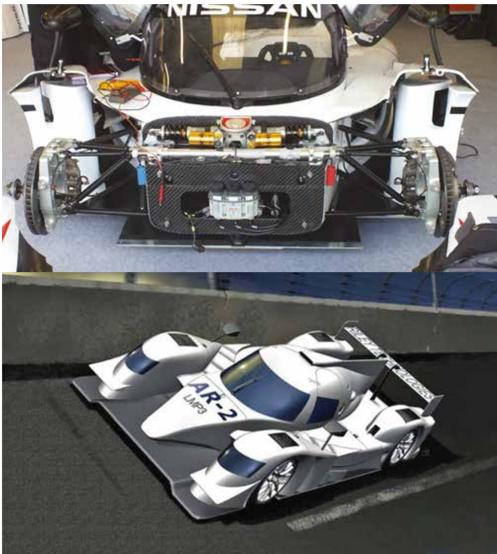
Top: The Ginetta suspension layout is based on coil springs rather than torsion bars and has been designed with ease of use and controlling costs in mind. Above: The design process for the Riley-Ave AR-2 has now finished and car build has started
