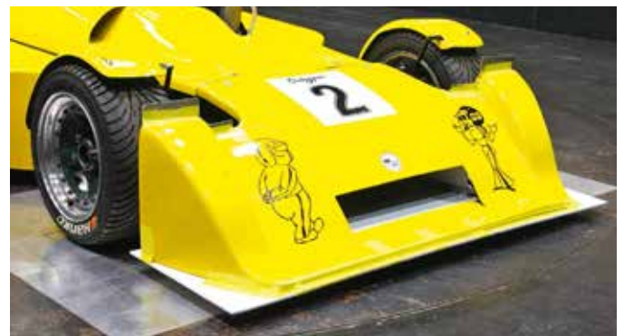
The floor panel under the nose made a significant difference to the aerodynamics
