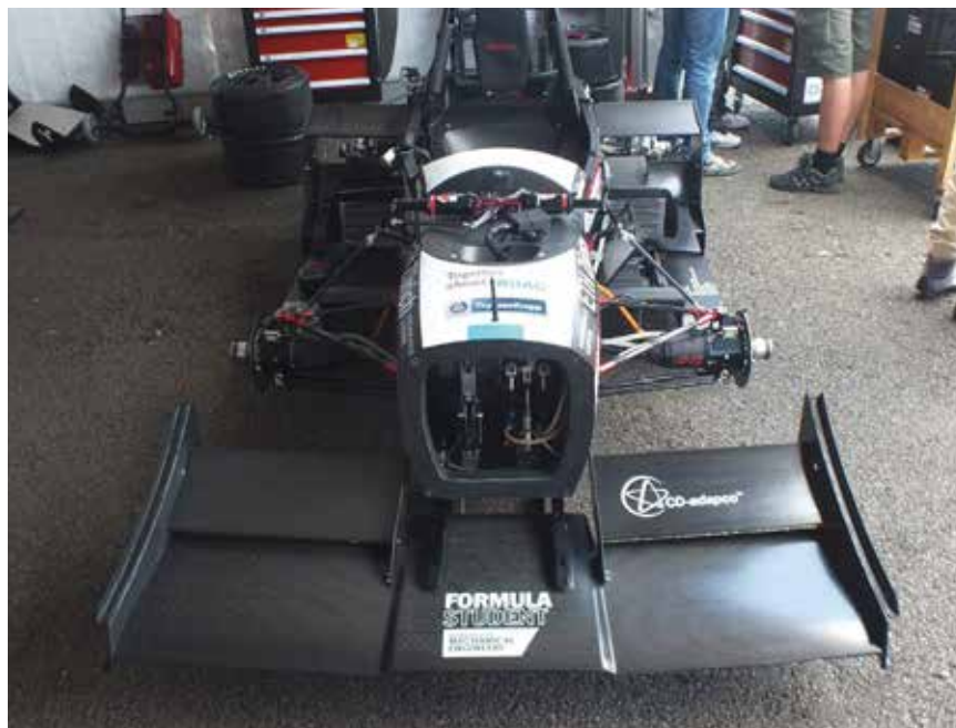
The ETH Zurich car is driven by four student-designed hub motors and boasts a neat composite monocoque
