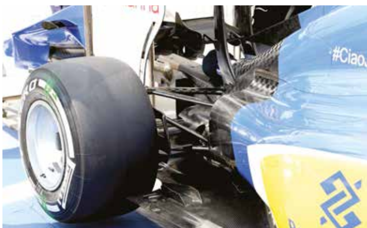
Much of the suspension work on the C34 has been focussed on improving the rear end of the car for better traction and stability. The rear wing supports pick up on the transmission casing
