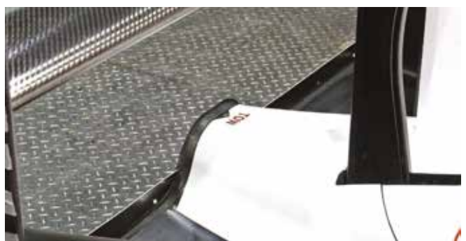
Baseline rear deck Gurney was increased in height by two 15mm increments to good effect; the first of the changes producing the largest effect in terms of balance
