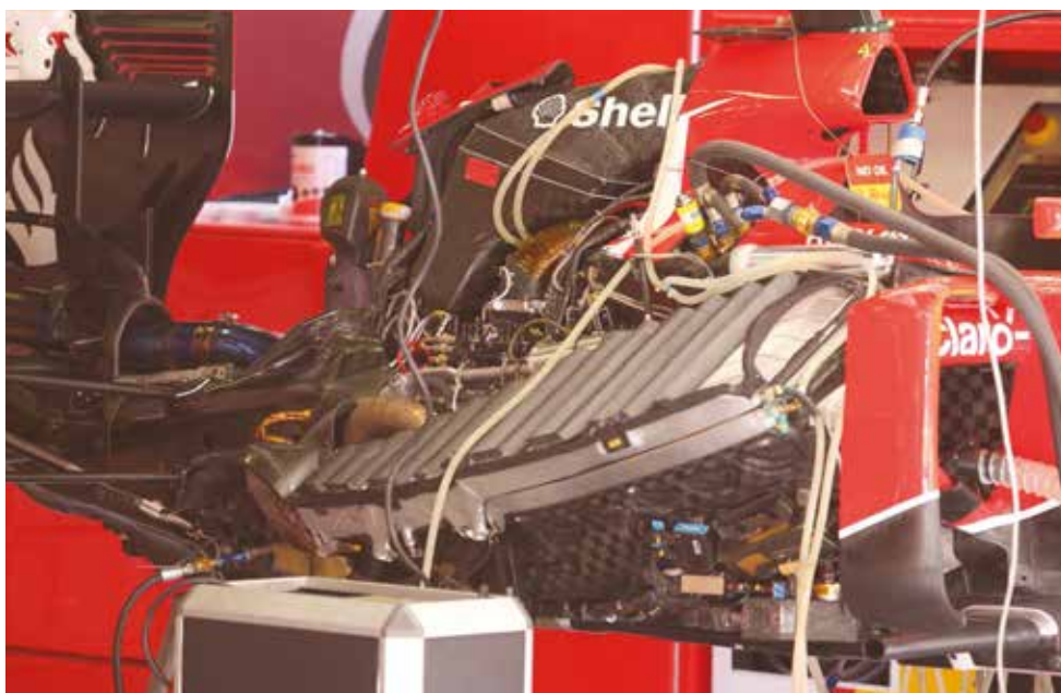
Cooling is vital with new breed of power units and Ferrari has crafted louvred coolers to help with heat efficiency on 059/4
