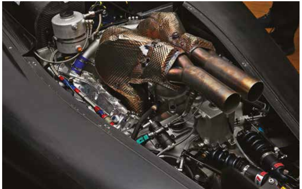
Above: Word in the paddock is that the new 3.4-litre normally-aspirated Mecachrome V6 in the GP3/16 could also power the new Formula 2 car in turbocharged form. Exhausts are mounted in the V of the engine, with the air inlets on the side
