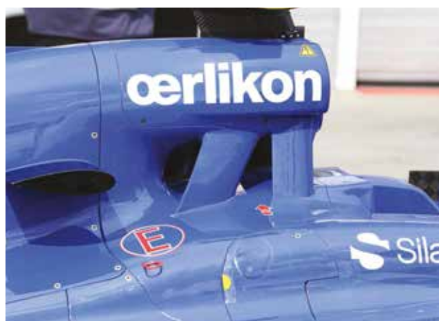
The roll hoop structure is a direct carry over from the 2014 Sauber and follows a concept first used in Formula 1 by the Force India team a number of years ago
