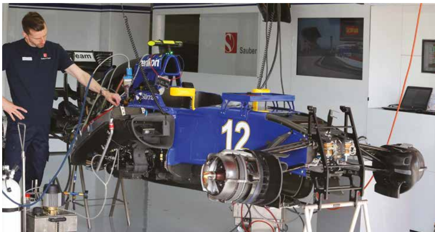
Due to the sheer amount of mechanical and electrical systems it has to pack, the modern F1 car is a long piece of kit and this has led to understeer problems, Sauber tells us
