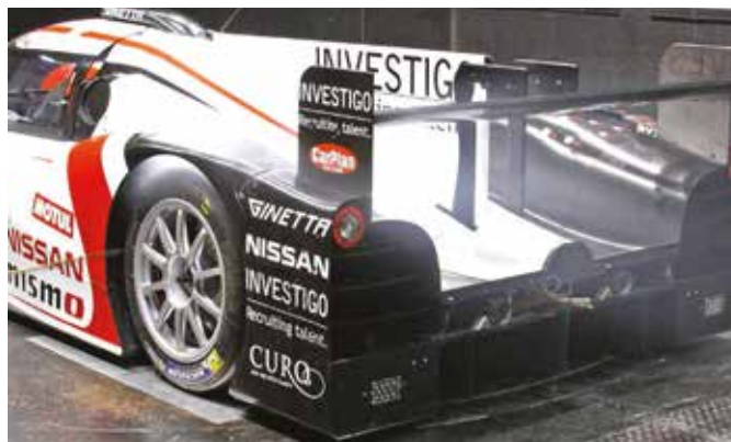
Air emerging from the rear wheel arch top apertures clearly interacts with the rear wing's flow field. The rear wing is limited to a single element of 1600mm span
