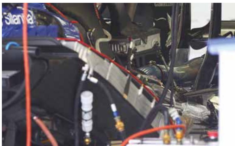
Some radical and innovative packaging solutions have been used in the C34. Sauber has also switched to horizontal mounted radiators, allowing for even tighter sidepods than nimble C33
