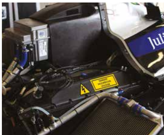
An updated spec cooling system has been fitted to the base SRT_01E car, this features a reduction in the radiator size. Teams have also been given some freedom when it comes to the cooling
