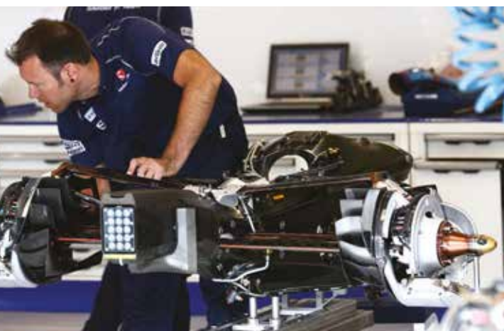
The Ferrari transmission is very different from 2014, which has meant Sauber had to mount damper elements in bellhousing and use pullrods to actuate them
