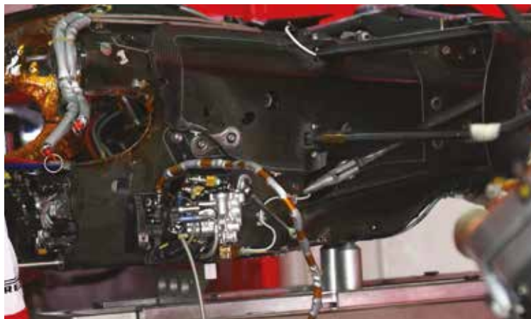
Also inside the bellhousing are a number of hydraulic components, plus dampers and torsion bars. All of these parts are exposed to very high temperatures and yet still perform as required
