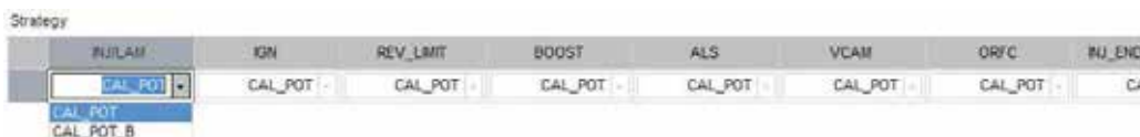
Fig 2: Defining the source to use for each strategy is critical when more than one Cal Pot is available
