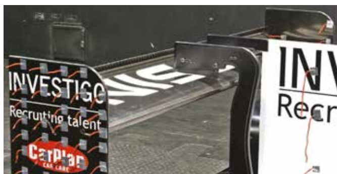
A 25mm wing Gurney in place of original 10mm item made a useful contribution
