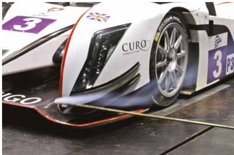
The front features an LMP2 style splitter and twin dive planes, the latter of which generated a powerful vortex when the smoke plume was put to work at MIRA
