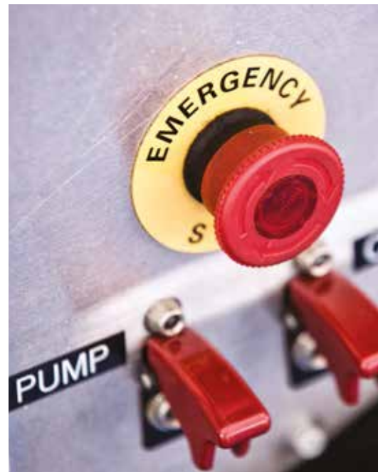
Sturdy switches are needed on record cars and the team had to make sure that everything was still switched on after each run
