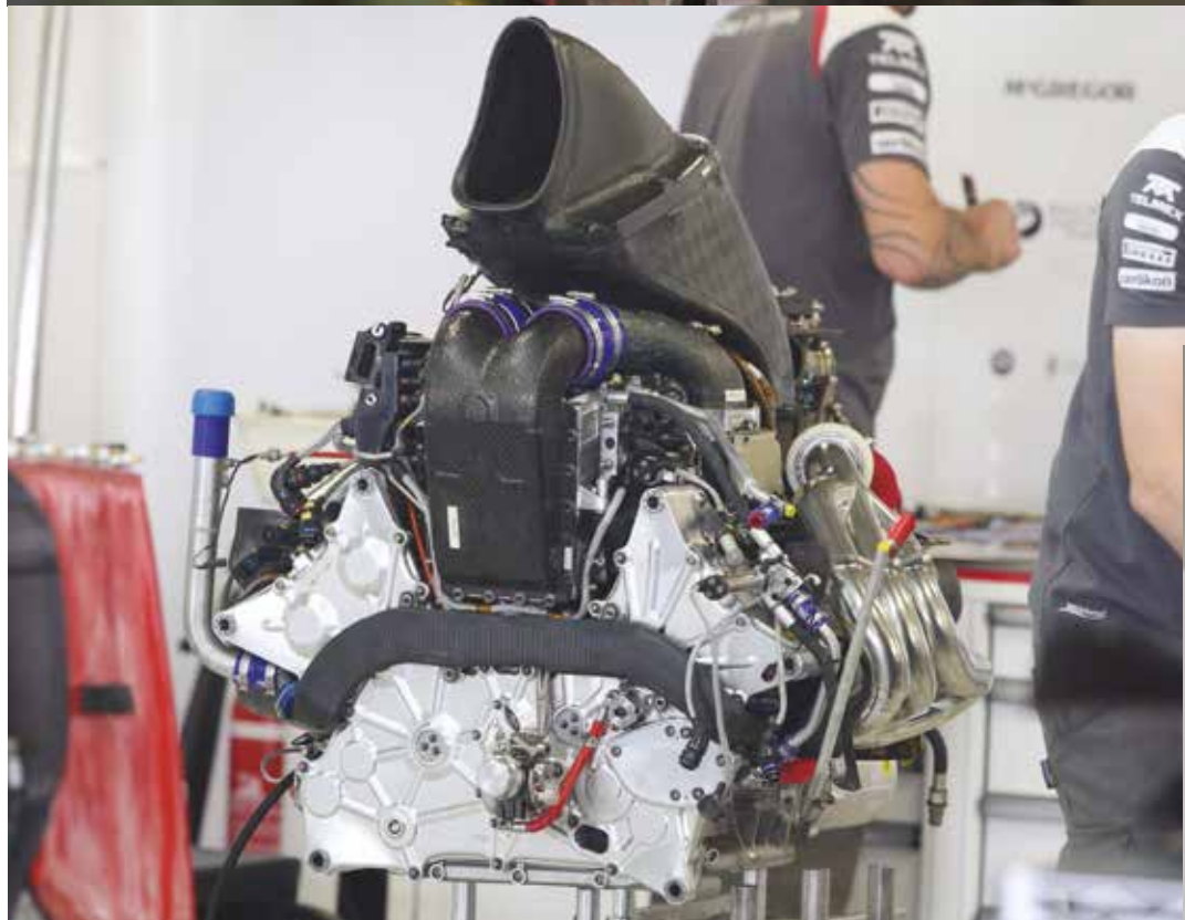
Top: 2014 power unit (the 059/3). Picture shows the exhausts swathed in thermal protection, something that Ferrari did not do for much of the season, baffling many as this meant it lost heat which reduced the recoverable energy of the MGU-H Above: Another shot of the 2014 unit; the intake and charge cooler in the V of the block can be seen here. A feature of last year's engine was the tight path taken by the exhaust manifolds, curling upwards into a three-into-one layout on each bank
