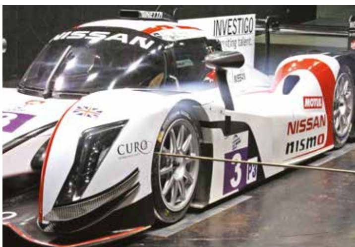
Mandatory wheel arch top apertures on front and rear of car allowed the air to escape
