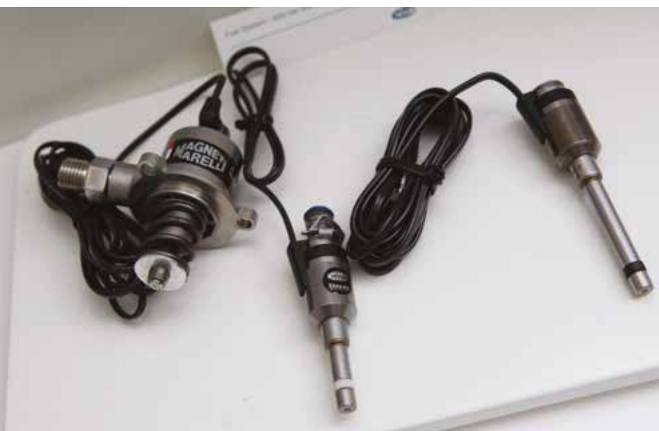
These Magneti Marelli injectors are the same as used in the 059/4, though they may differ in appearance
