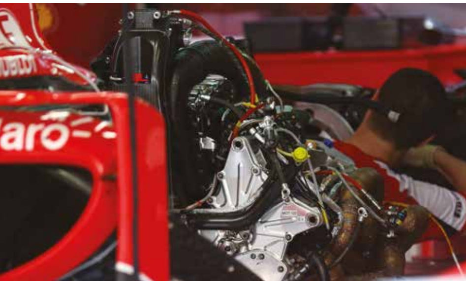
The 2015 power unit (059/4) has a relocated oil tank, now mounted at the front of the block as per convention
