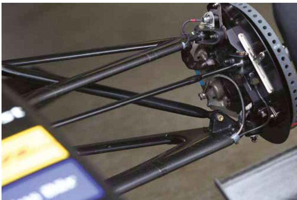
The suspension has been beefed up for season two with the addition of bulky and reinforced lower ball joints, which have been added to the front wishbone. FE made this change because of some high profile crash damage issues in season one
