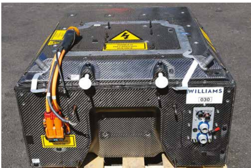
Williams Advanced Engineering-supplied batteries were originally designed for race power of 133kW but this rose to 150kW before first season and for season two it's to go up to 170kW in the races. This move has proved controversial in FE paddock
