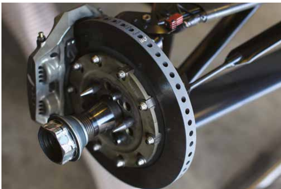
A new brake disc is among the changes to the Dallara-built SRT_01E racecar for season two of the Formula E Championship while new brake pad geometries have been introduced by the championship's brake supplier, Tamworth UK-based Alcon
