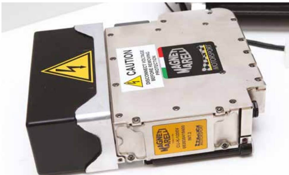
Magneti Marelli is trying to reduce the weight of the capacitors, which are housed in the black section of the inverter
