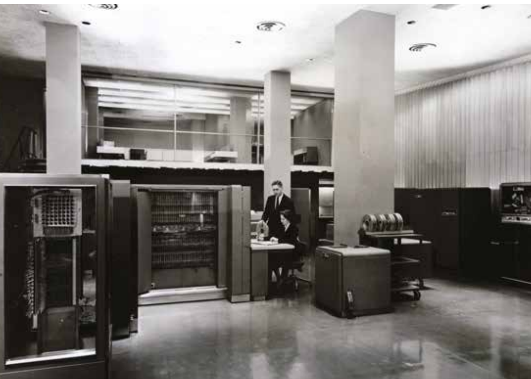
Chuck Carrig wrote a computer programme for this vacuum-tube driven IBM 704 to simulate suspension movement in 1958
