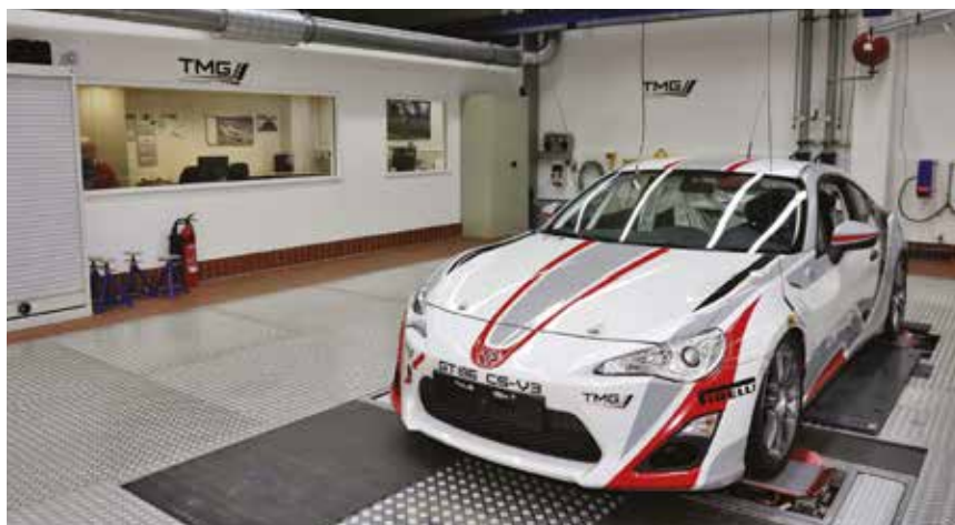
Hardware-in-the-loop (HIL) means DIL simulators are linked to test rigs in real time and this can theoretically be used in both directions; but in reality there is at present a bit too much lag with HIL to driver connections
