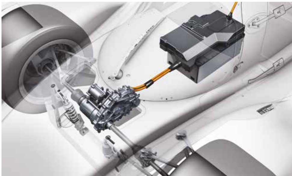
Porsche's system uses the second exhaust turbine/MGU coupled to the front axle, and is complex and expensive, Hitzinger admits. Harvested energy can only be deployed via the front axle while Toyota can share between both axles with its system
