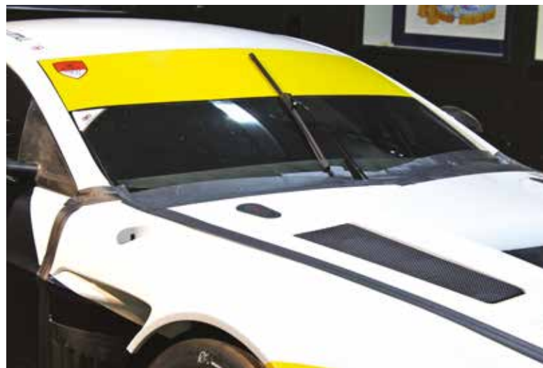
Blanking off the Aston's front scuttle and its forward door shut line was a useful exercise
