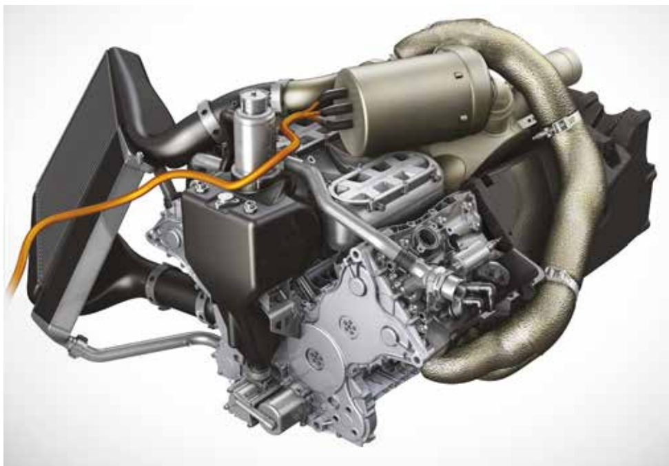
The exhaust turbine arrangement that is mated to the dinky little V4 internal combustion engine is unconventional. There are a pair of turbines involved, one of which drives the induction air compressor, while the second drives the MGU-H
