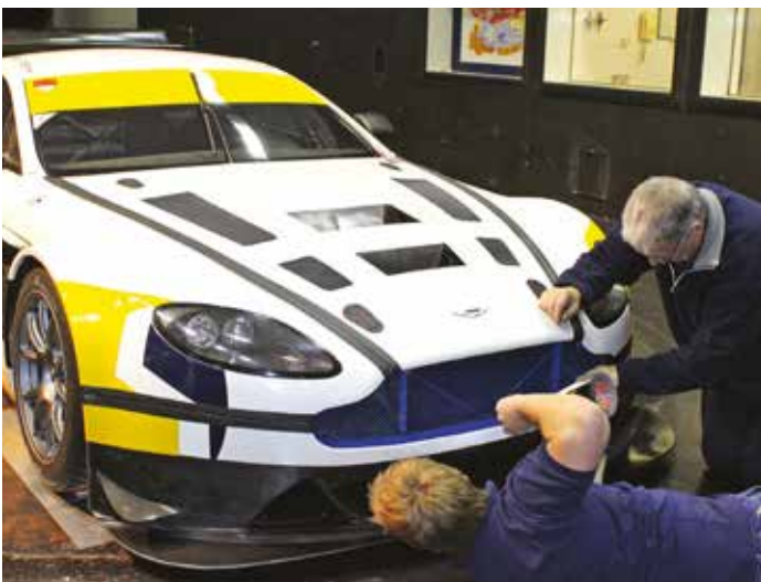
Taping over the forward panel gaps on the Aston Martin GT3 at the MIRA wind tunnel
