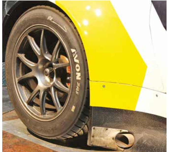
A 10mm spacer can just be seen here under the rear wheel. This additional rake produced a typical response despite the absence of a flat bottom and rear diffuser
