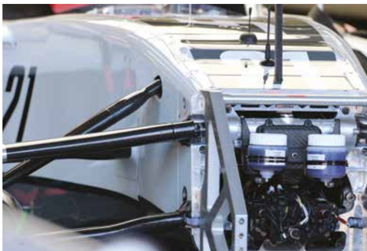
The steering rack on the Haas F1 car. One of the biggest challenges for car development with simulators has been to replicate steering feel and this has also been one of the great advances
