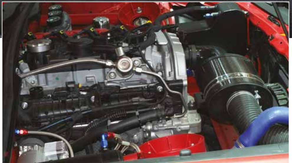
The turbocharged DOHC 1.8 direct injection 4-cylinder powerplant is called the Bialbero. It produces around 300bhp and it is actually the same engine architecture as used in the Alfa Romeo 4C. Abarth has tuned the unit for World Rally competition
