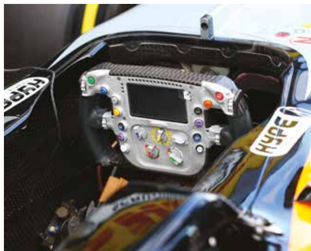
F1 steering wheel displays have been made clearer to read and more intuitive thanks to work in the simulator in response to recent pit-to-car radio restrictions
