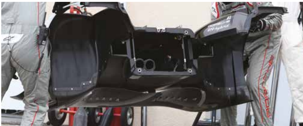
The nose of the Porsche 919 Hybrid, featuring the larger cut outs over the front wheel and strakes in the splitter under the nose. Teams are directing more air through the car as they deal with a reduction of 10MJ from the fuel allowance in 2016
