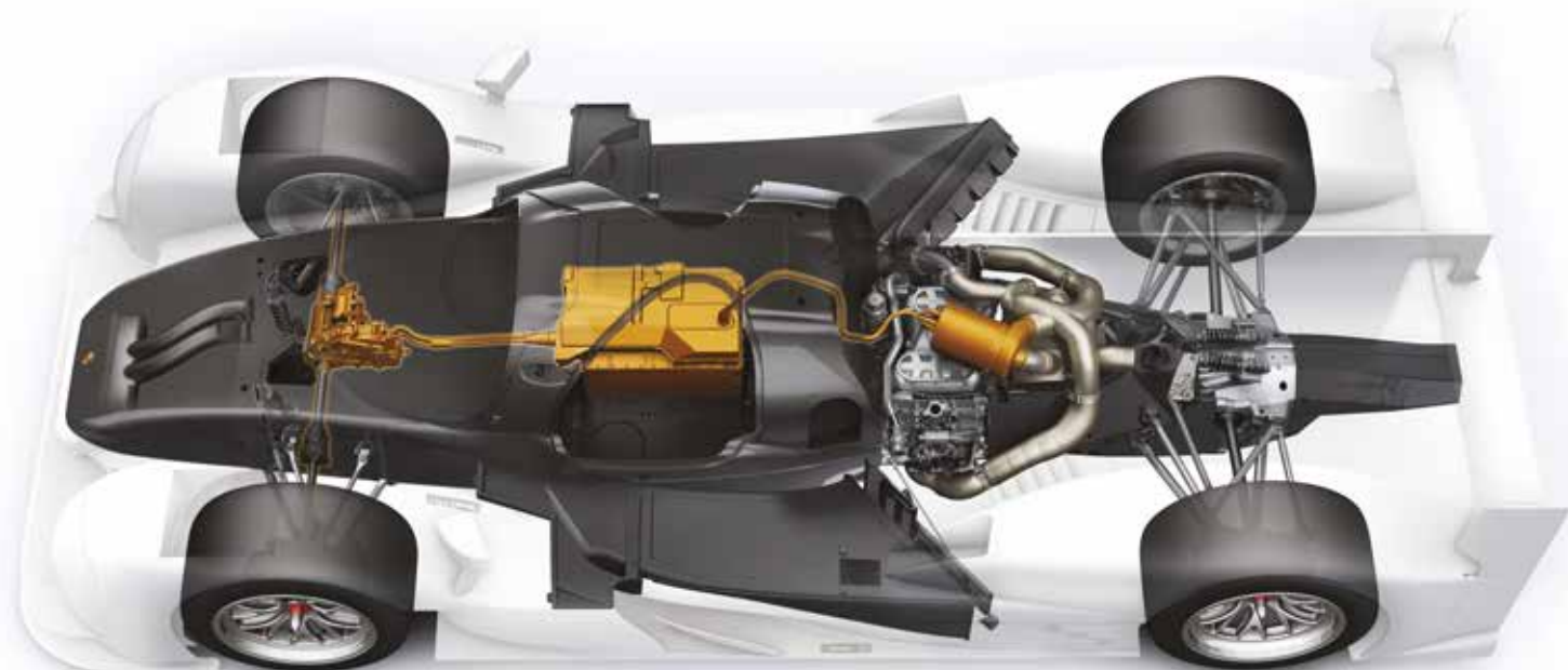
The MGU-K (front) and MGU-H (rear) in the 919, and how they connect to the battery. Front generator is operated as a single motor and drives the front wheels via a differential
