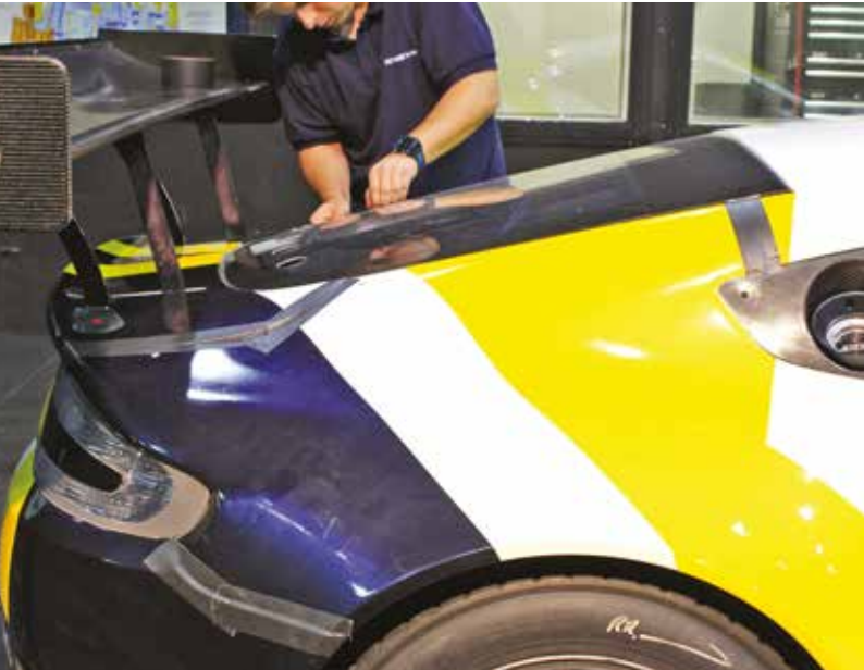
Panel gaps between the rear wheel arches and bumper; the wheel arches and the boot cover; and between the roof and rear arches were taped over. This had minimal influence
