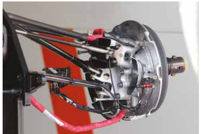
The inner face of the front upright; the red cables are the mandatory wheel tethers. Front suspension is actuated by pushrods, as it was on the MRT05's predecessor
