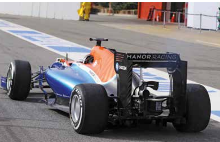
The endplates are a direct carry-over from the stillborn 115 but much of the MRT05's rear has had to be radically redesigned to house the new engine and transmission
