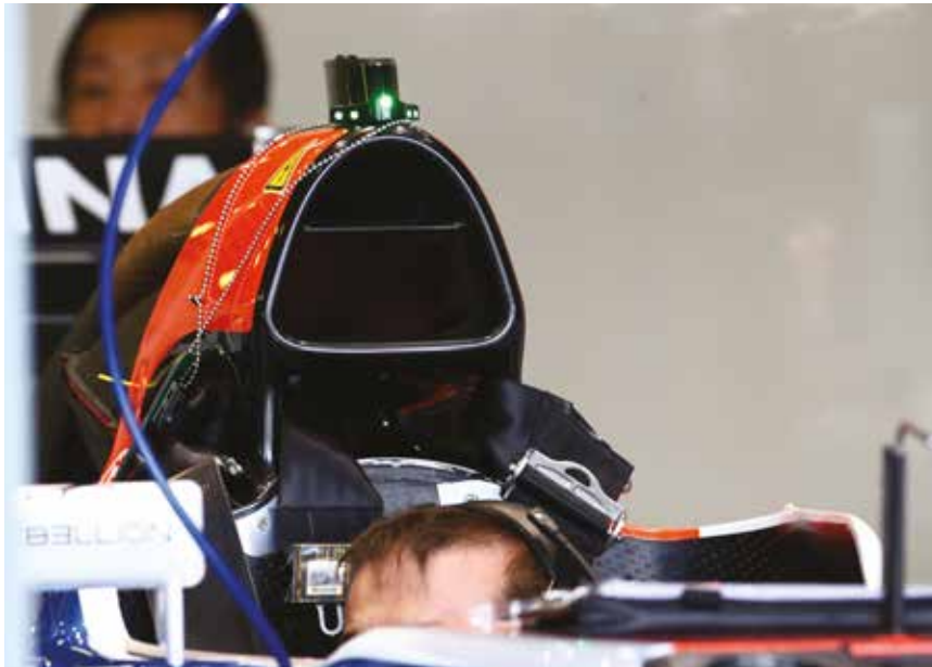
The roll hoop ducting of the MRT05 is quite different to that of the MR03 and the 115, as to install the new Mercedes power unit the coolers, which had been positioned here, had to be relocated to the car’s sidepods
