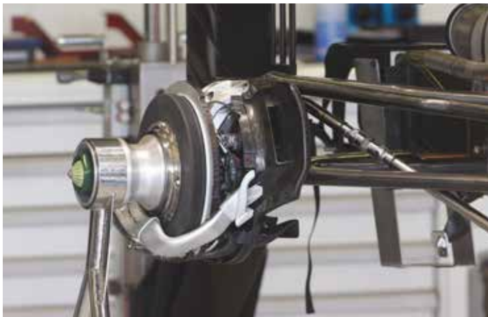
The rear brake assembly on the MRT05 has a different ducting to that on the stillborn Manor 115, but it uses the same caliper position. The rear suspension is pullrod actuated
