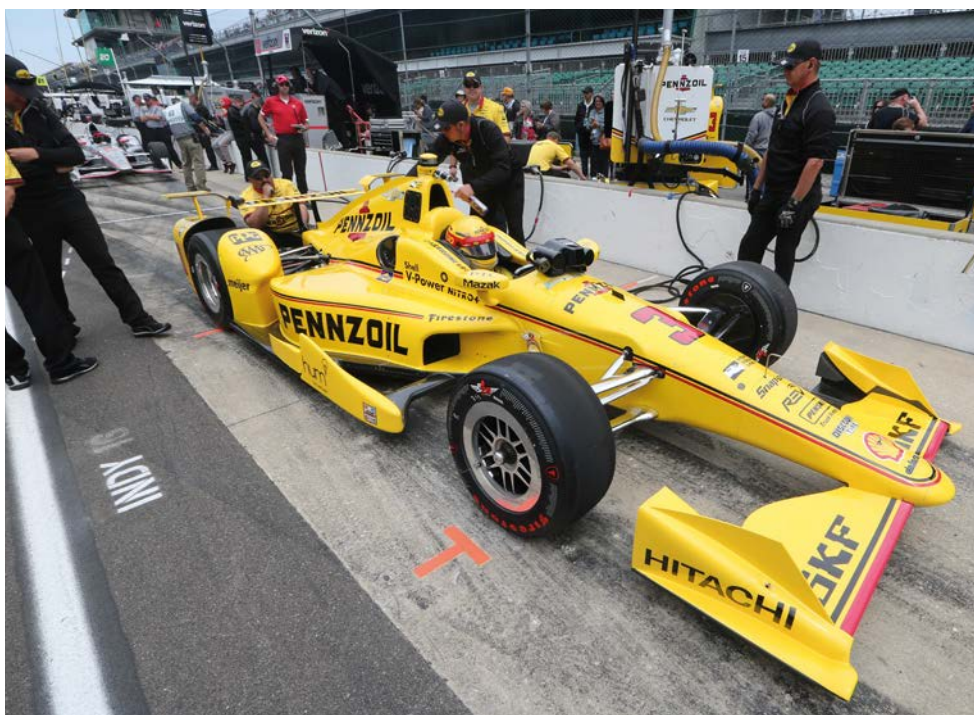
The triangular aero device ahead of the sidepod was designed to reduce air pressure in the event of a high speed spin. This year cars have been far less susceptible to flipping while the aero measures have also slowed them before they hit the wall
