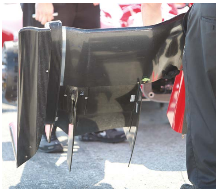
While the top surfaces of the wings became more complex IndyCar banned underwing development. The series will now look for more underwing downforce with its universal kit
