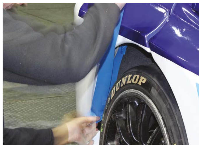
Once again we found it is slightly better to leave rear wheel arches open at the rear
