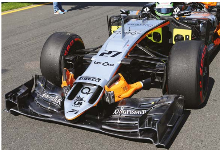
New heavily modified front wing was a part of the highly successful Barcelona upgrade, its purpose is to generate rear load. Nose still sports the distinctive nostrils introduced last year
