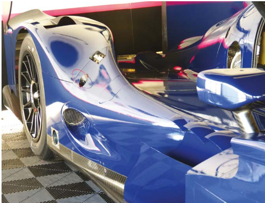
Ligier has optimised the cooling on the JS P217 by turning to Mezzo technology, as used in Formula 1 and LMP1. This meant that it could drop the size of the exchanger, make the cooler more efficient, and reduce drag
