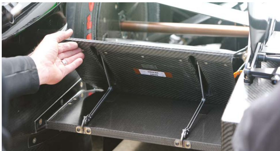
Following a spate of high profile accidents at 2015 Indianapolis 500 practice sessions the IndyCar series introduced a number of aerodynamic measures designed to slow a car and stop it becoming airborne during a high speed gyration
