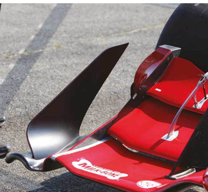
One of the by-products of the more open body kit regulations were complex road course front wing arrays which were apt to break and cause yellow flag periods
