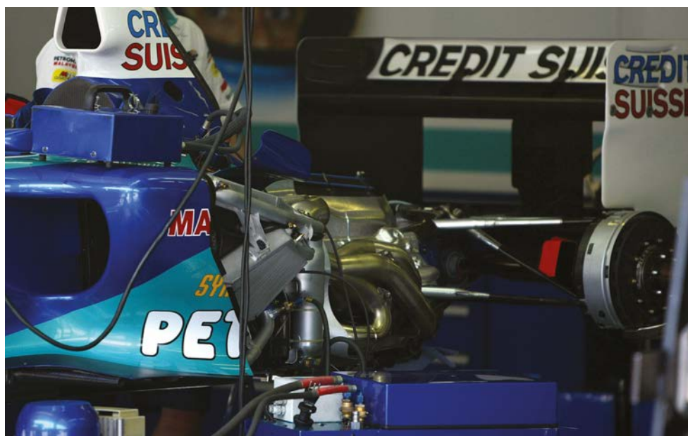
The Ferrari V10 in a Sauber in 2005. The external features of the engine were also heavily developed during this halcyon period of F1 engine design. Snorkel inlet designs were constantly optimised in order to maximise the charge air density
