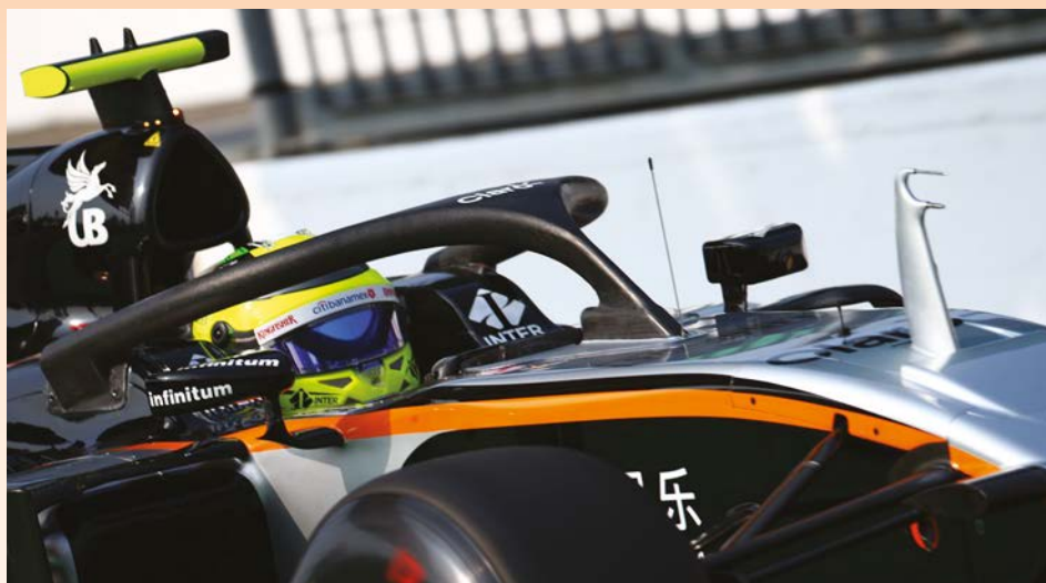
In the interests of driver safety Halo, or some other form of cockpit protection, looks set to be a part of F1 from the 2018 season onwards and many of the teams, including Force India, have run in practice sessions with such devices fitted
