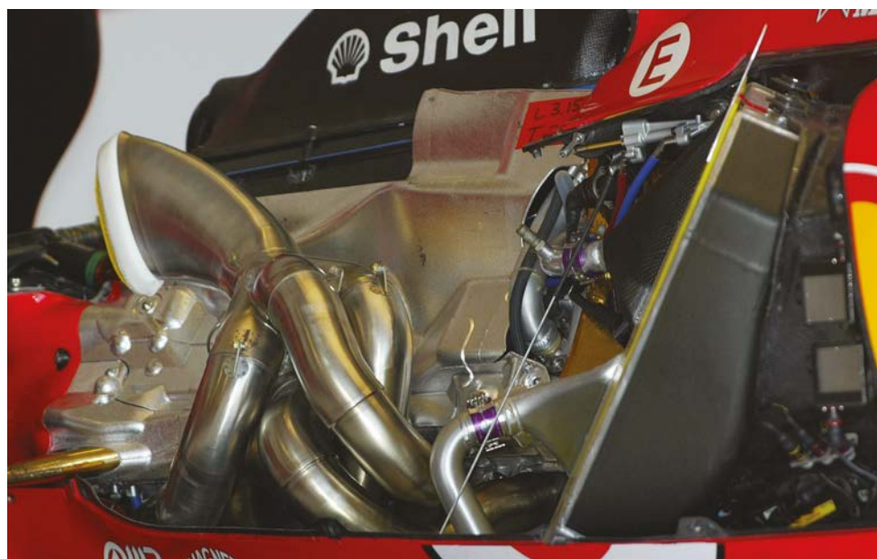
The Ferrari V10 engine pictured in 2004. During the period of free thermo-fluid engine development in the V10 era the main engine design objectives focused on maximising the engine speed to increase the air flow rate and hence fuel flow rate too
