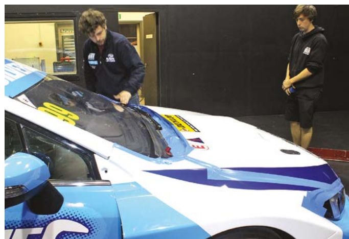
The bonnet and scuttle sealing taping exercise yielded some useful aerodynamic gains
