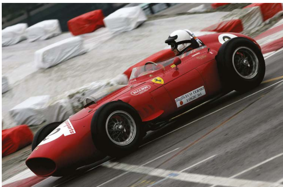
Ferrari's Dino 246 was one of the last of the front-engined GP cars – note that the powerplant sits behind the front axle line
