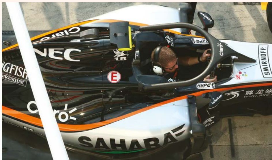
Force India's technical director Andy Green says that to fit the Halo device will require the construction of a completely new chassis, due to the loads it will have to withstand, and that Halo could not be retro-fitted to an existing monocoque
