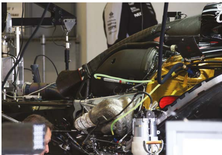
Force India's philosophy with the power unit is to run it to the very limit of the guidelines that Mercedes gives it because every extra degree cooling is downforce that's not being generated
