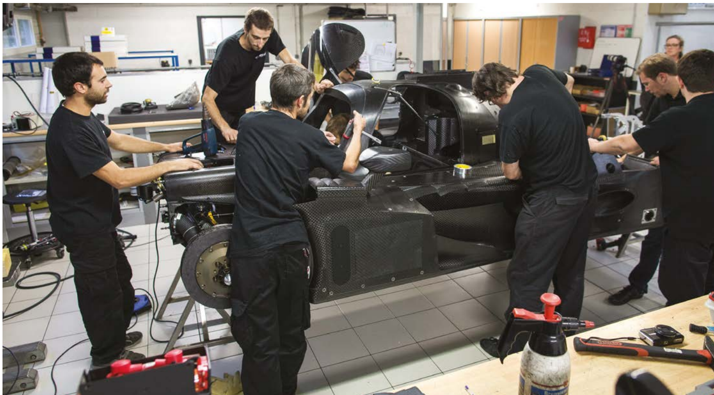
Ligier has used new materials in the JS P217 chassis, such as T1100 carbon, which has allowed it to absorb the extra weight of the Zylon panel that is part of the new rules package
