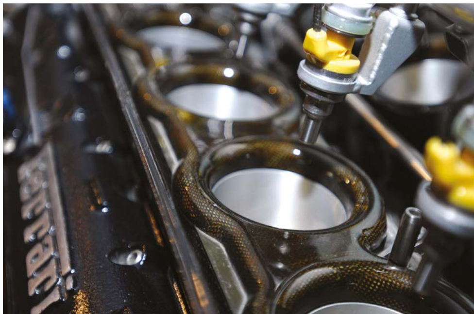
There was a concerted effort to focus on optimising inlet port flow coefficients at high lifts at Ferrari during F1's V10 era
