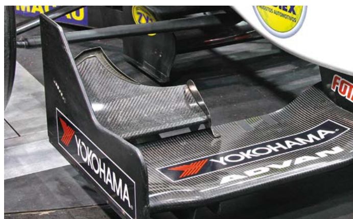
Photo 4: The inboard front flap end plate on the Dallara F308 Formula 3 car
