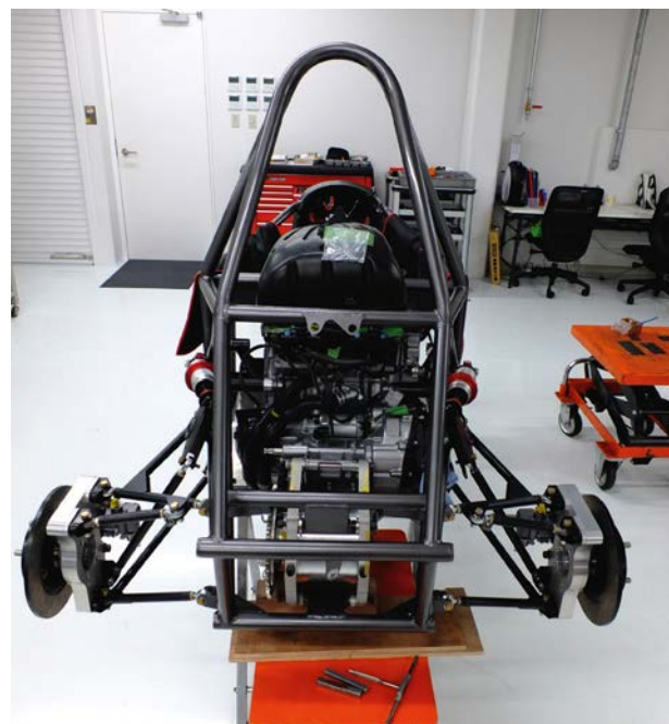
It packs a Honda 650cc engine at present, which gives around 80bhp, but Dome says it should be possible to fit a larger unit
