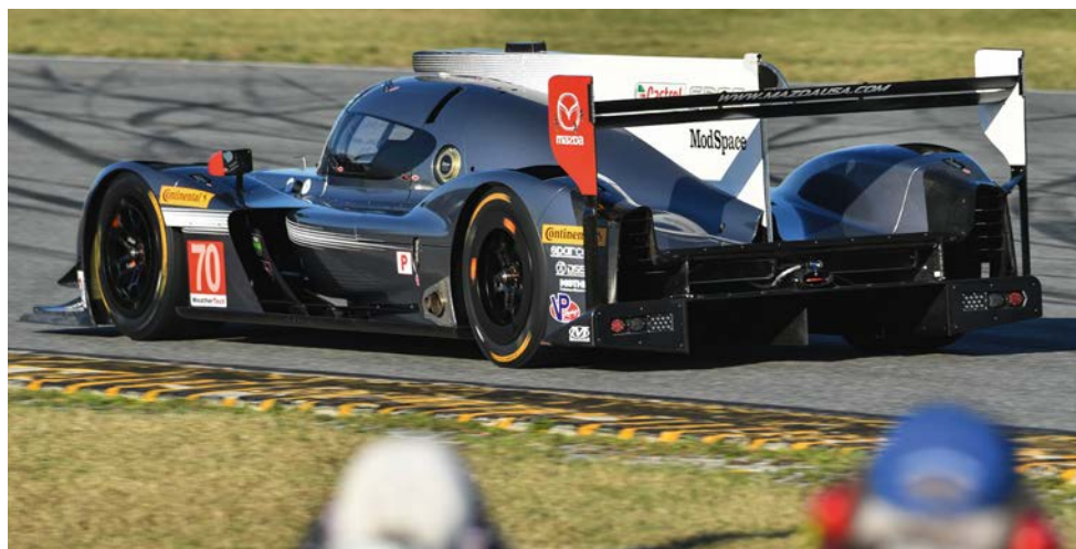
Despite the need for Mazda styling cues there are some neat aerodynamic touches such as the remote rear wing mounts
