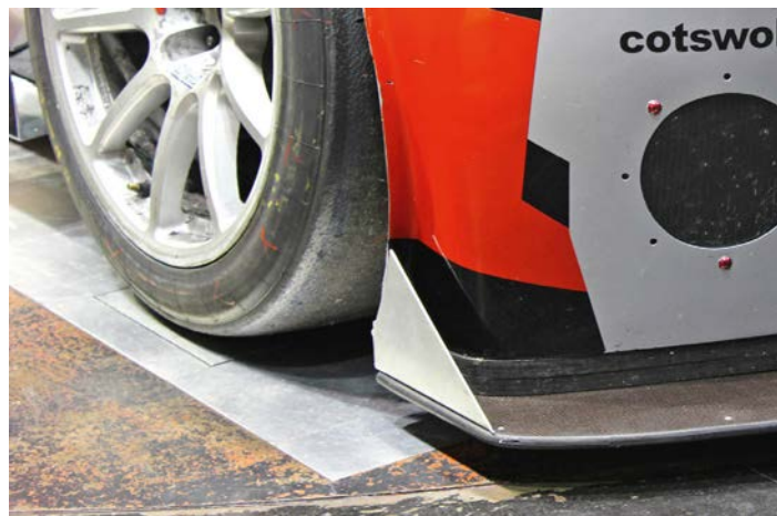
The small splitter end fences achieved good forwards balance shift
