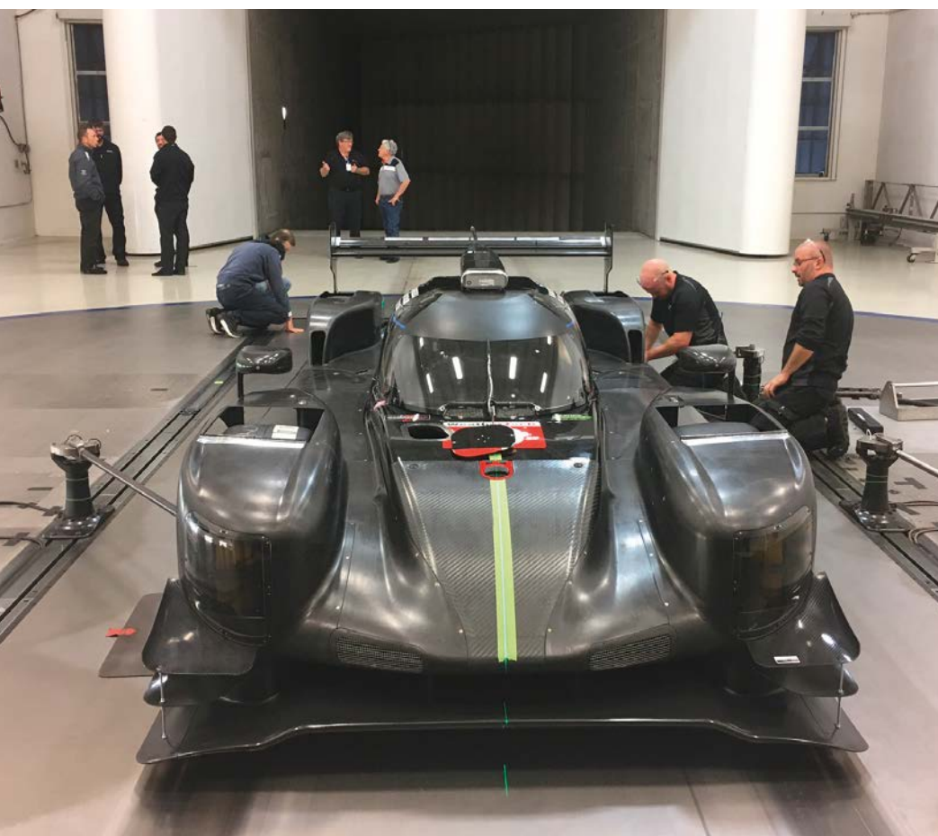
The DPi Cadillac has its bodykit put through the full scale aero tests in the impressive Windshear facility in North Carolina
