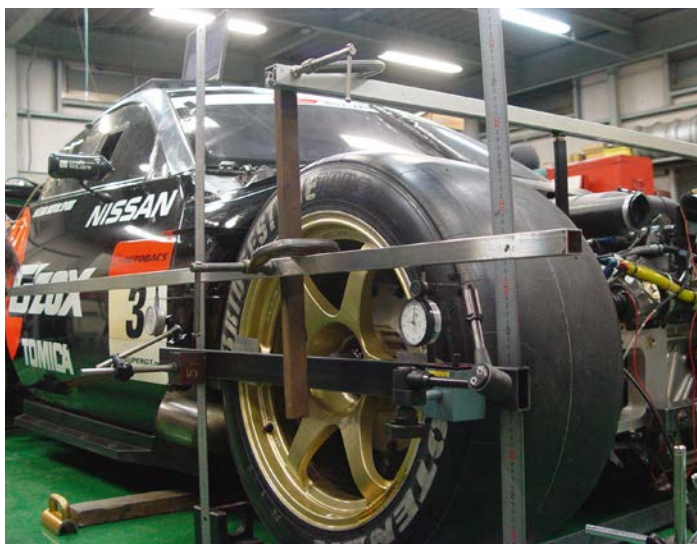
This complicated looking arrangement is the toe, caster and camber bars and the dials
