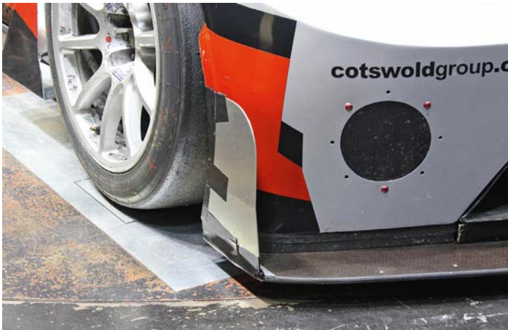
The large splitter end fences were not as successful as the smaller examples when tested
