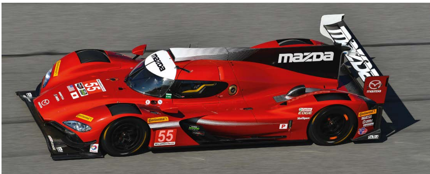
Periscope exhaust has been chosen over the side exhaust (see below). Mazda had to wait until the LMP2 version of Riley-Multimatic was finalised before detail design could start
