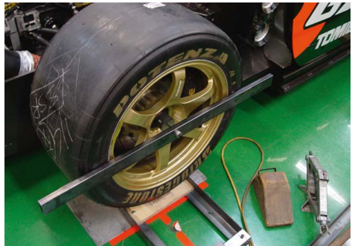
To measure the deflections you need to use a beam mounted on the wheel with clamps
