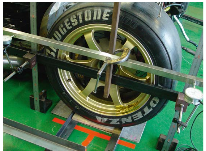
This shows the caster measurement process with the rulers fixed on to the wheel bar
