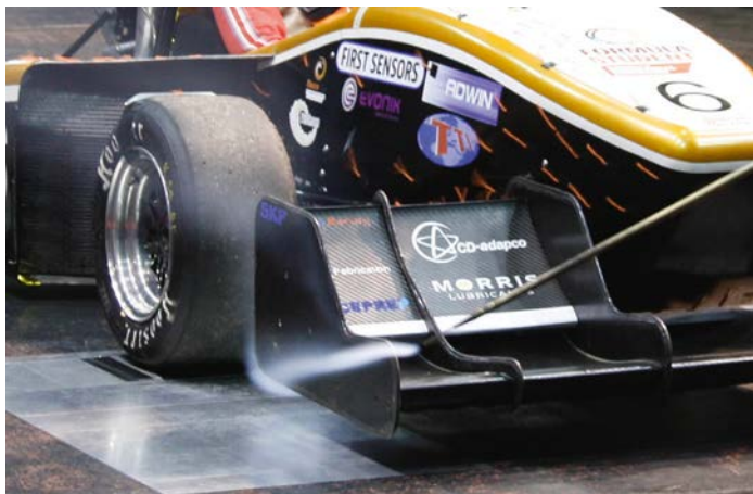
Photo 2: Lower tip vortex passes under the end plate and inboard of the front wheel
