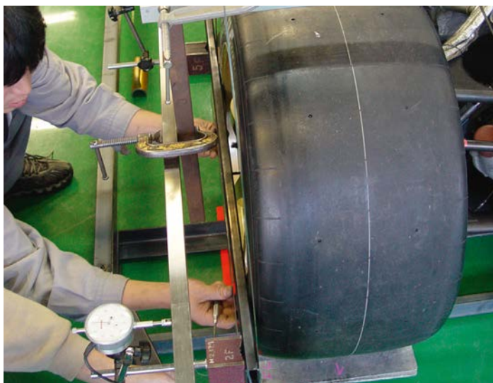
Load ratchet pulley in increments and record gauge values and compile a table of results
