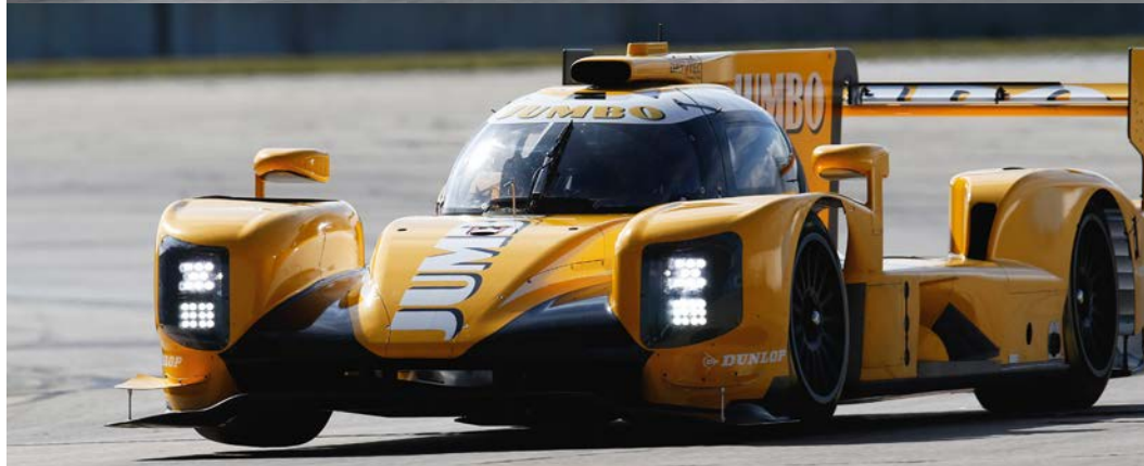
Top: Dallara Cadillac with subtle design elements; in line with new DPI regulations and the US firm's marketing ambitions Above: Dallara P2 is a more purposeful package. Note airbox design on roof, and headlight design as clear differences
