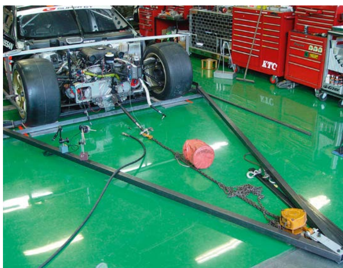
As the testing frame is actually pulling against itself it will not need to be restrained
