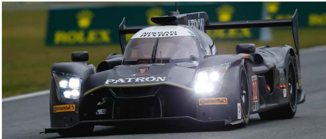
Top: Dallara Cadillac with subtle design elements; in line with new DPI regulations and the US firm's marketing ambitions Above: Dallara P2 is a more purposeful package. Note airbox design on roof, and headlight design as clear differences
