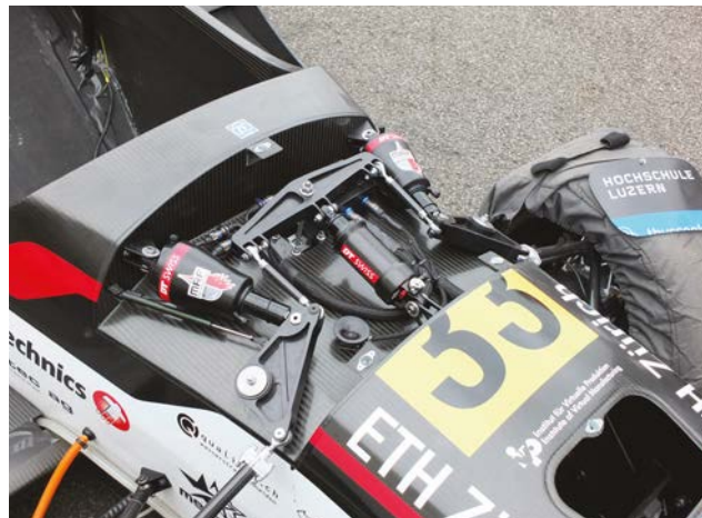
Third element suspension systems, as used on this Formula Student project, feature a heave spring to support the aerodynamic loads acting on the car
