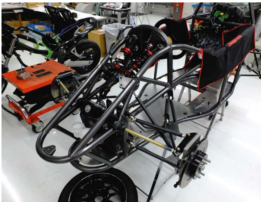
The Cheetah features double wishbone front suspension; front uprights are from the Dome F4 car. It also uses AVO dampers. The robust spaceframe is made from tubular steel and the little racecar weighs in at 320kg
