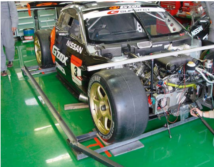
Car restrained on all four wheels with the two frames interlinked will reduce wheel loads
