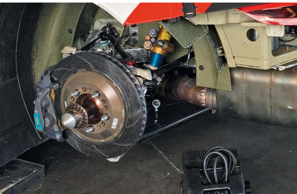
The rear brake assembly and suspension. The latter has changed to a double wishbone layout – the 2016 Porsche was multi-link. Suspension features four-way vibration dampers and twin coil spring set-up, comprising main and helper spring
