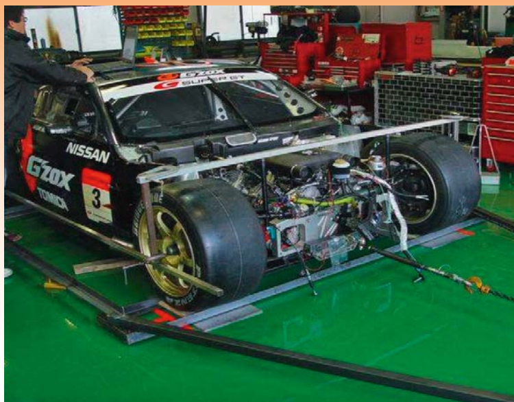
The ratchet chain pulley system is effective and much cheaper than hiring time on a K&C rig
