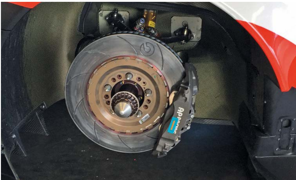
The RSR packs two independent brake circuits for the front and rear axles, both adjustable via balance bar (front brake assembly shown). Front has six-piston racing calipers and internally ventilated steel discs, four-piston calipers at the rear
