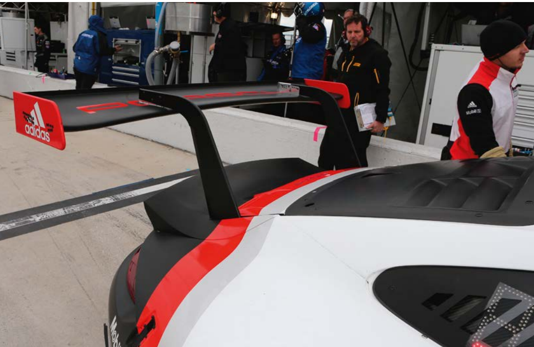
The RSR’s rear wing is mounted under the supports to clean up the airflow passing underneath it. Under the chassis Porsche has also been able to include a substantial diffuser, thanks to the positioning of the powerplant further forward in the racecar
