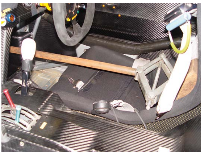
The car also needs to be restrained; here the brakes are kept on with a car jack and pole
