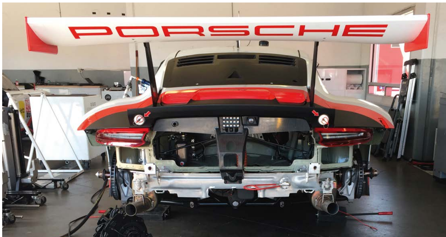
The engine position (not shown) is the main talking point with the 911 RSR – its normally aspirated unit is now located in front of the rear axle, leaving more space at the rear the car
