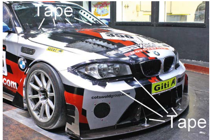
That old Aerobytes favourite, race tape, once again proved its aerodynamic value
