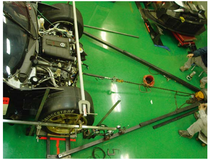
A view from above of the toe rig assembly. The car may need to be loaded with ballast
