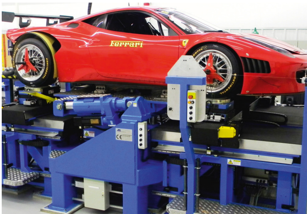
A kinematics and compliance rig is a very expensive piece of kit but there are some lower cost alternatives
