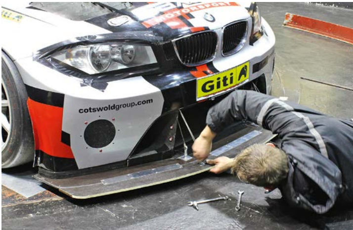
Extending the splitter worked well, effectively adding over 100 counts of front downforce
