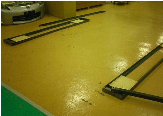
This shows the individual axle frames that are a vital part of the test rig equipment
