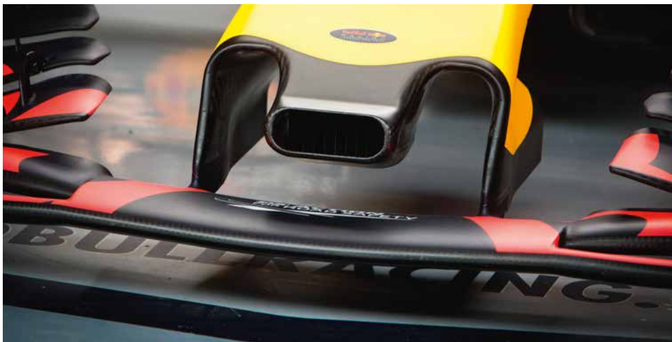
Red Bull RB13 has a duct in its nose which it claims is for driver cooling. Front wing is similar to 2016 except for delta shape
