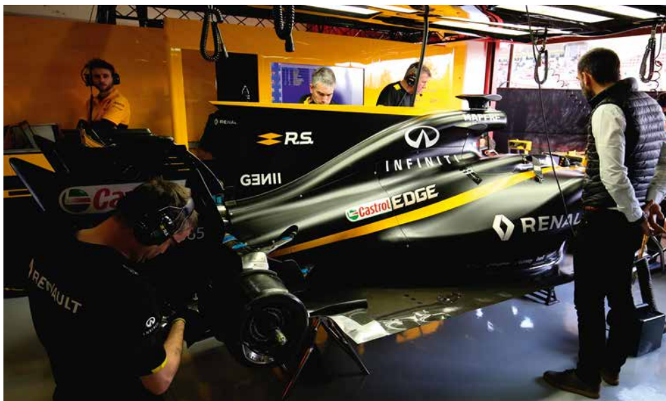
Renault's RS17 features the must-have appendage of 2017, a shark fin. Engine development has been a priority for Renault
