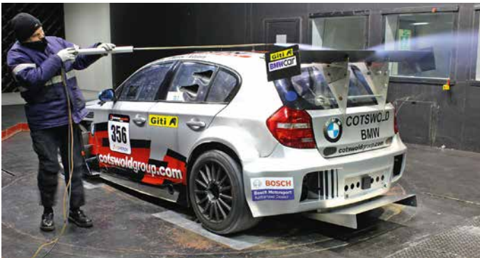
Testing rear wing modifications on the Giti/Saxon Motorsport BMW 1 Series racecar
