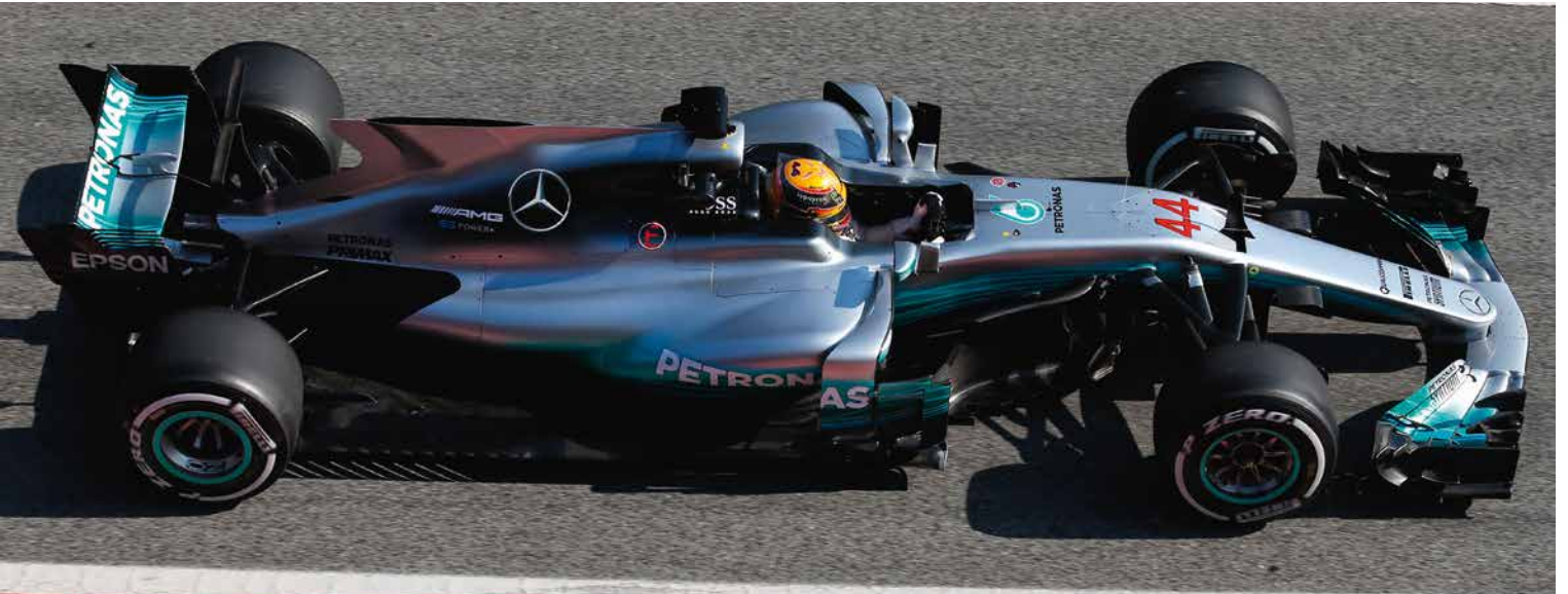
Top: The 'looking faster' philosophy of the new rules is epitomised by the swept back rear wing endplates on the new Haas VF-17 Above: Mercedes W08 is seen here fitted with a cooling outlet that is integrated into the engine cover fin. Merc also ran without a fin Left: Ferrari SF70H boasts an unconventional sidepod and underfloor leading edge treatment, plus a radical cooling concept
