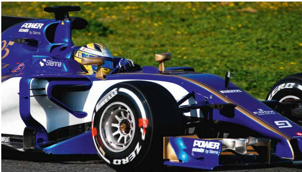
Sauber C36 has a central roll hoop structure with a split intake either side, similar to the 2009 Mercedes and 2010 Caterham
