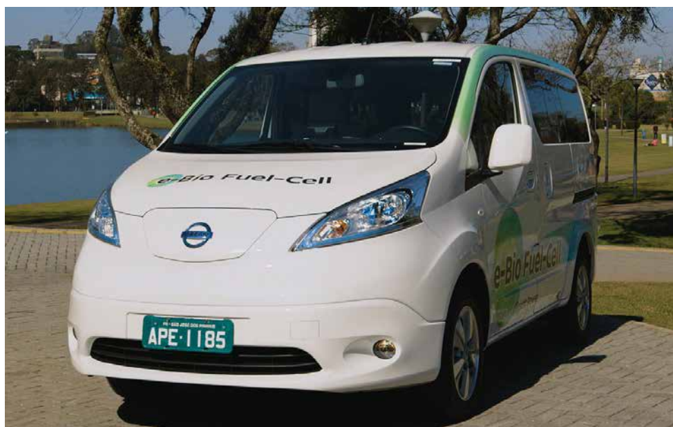
Nissan unveiled this ethanol-powered hybrid fuel cell van in Brazil last year. It has a nominal range of 600km and is already running on public roads. The Japanese car giant has plans to bring ethanol fuel cell vehicles to market in three years time
