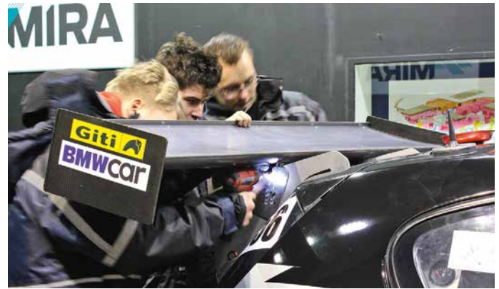
The fitting of a large Gurney had a big effect with added downforce but also added drag
