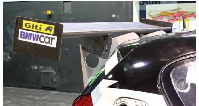
The tailgate on the BMW was changed. Standard hatch terminated with a slight flick up
