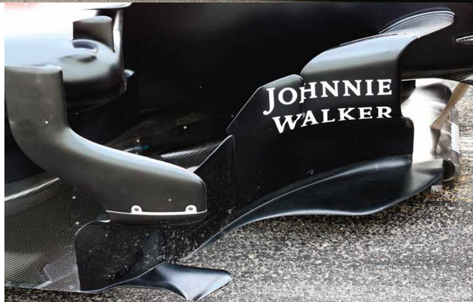
Right: The new McLaren MCL32 (note the new numbering protocol) sports an extremely complex barge board arrangement
