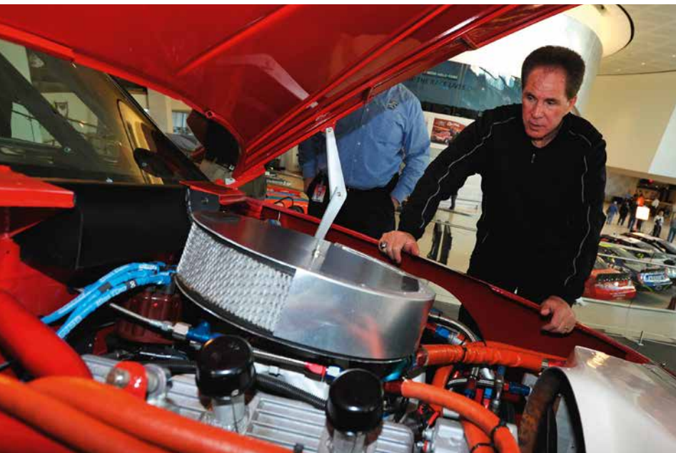
A big engine with a huge filter on it (pictured in a 1986 car in the NASCAR Hall of Fame). Lumps like this were a natural result of NASCAR's drive to have true 'stock' cars in its early days, when most US cars had big V8s
