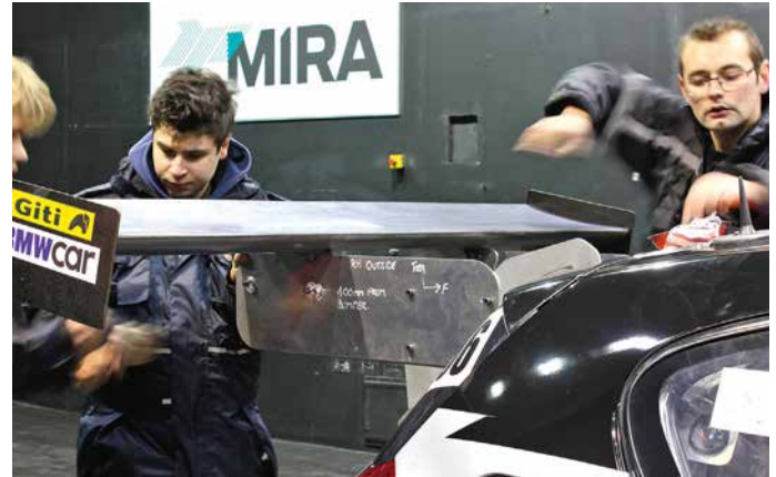
The rear wing overhangs for other race series' aero regulations were also evaluated
