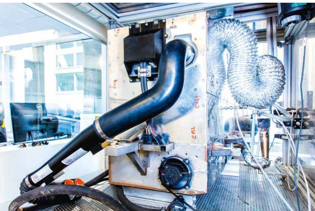
Nissan is leading the way in bio-ethanol fuel cell technology. This is its Solid Oxide Fuel Cell (SOFC) powered system. It's a fuel cell which makes use of the reaction of fuels, including ethanol and natural gas, with oxygen to produce electricity
