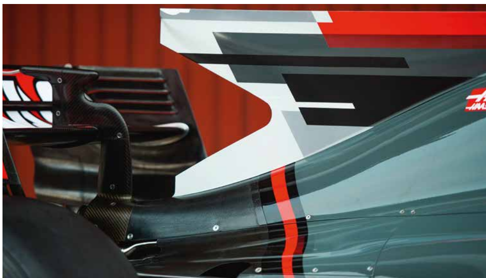
Haas also sports a fin, with an undercut in its trailing edge. Rear wing is conventional for 2017; note louvres on endplates
