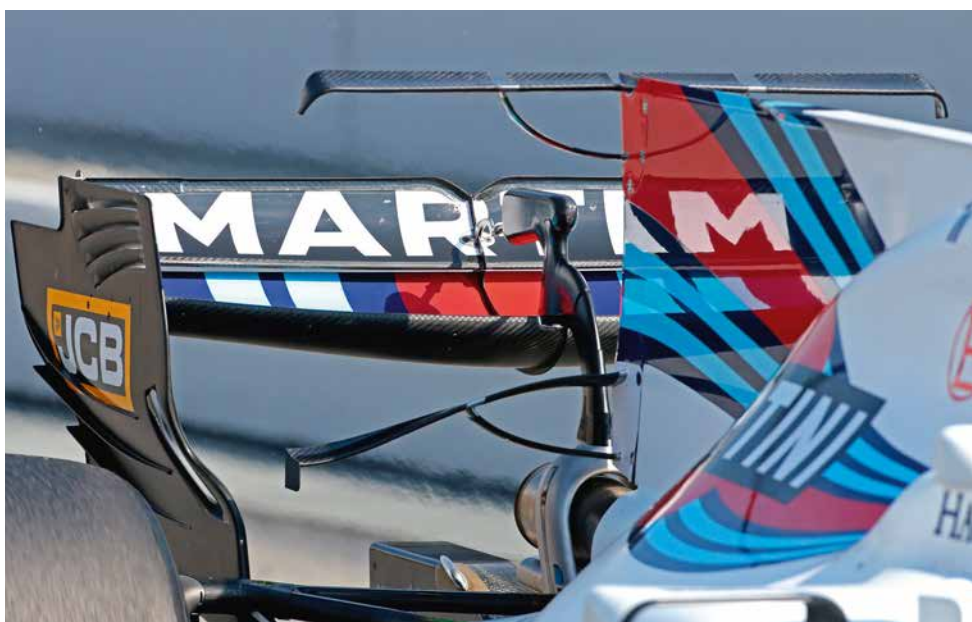
First seen on the Mercedes the T bars (here on the Williams FW40) are thought to help clean up the airflow to the rear wing
