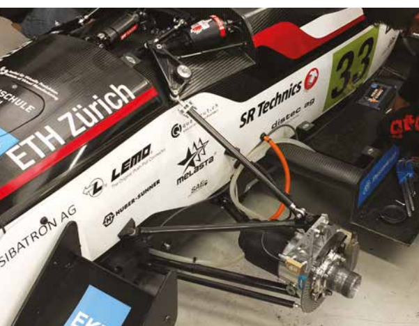
It's best to keep the uprights above the bottom of the wheel rims at all times, even if the tub dips lower than this. All the suspension pieces should clear the ground when the tyre is flat
