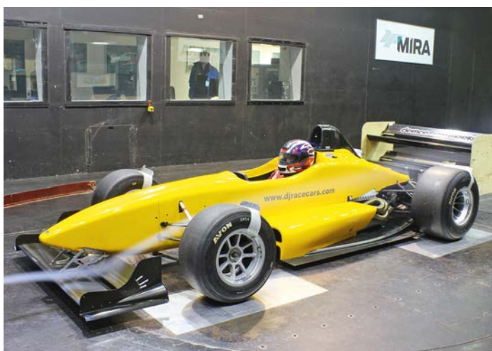
The 2.5-litre V6 motivated DJ Firestorm hillclimber being tested in the MIRA wind tunnel
