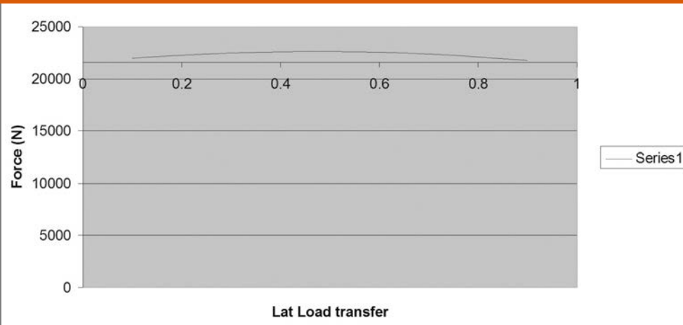
Figure 4: This shows how you can plot the total car grip as a function of lateral load transfer at the front of the racecar
