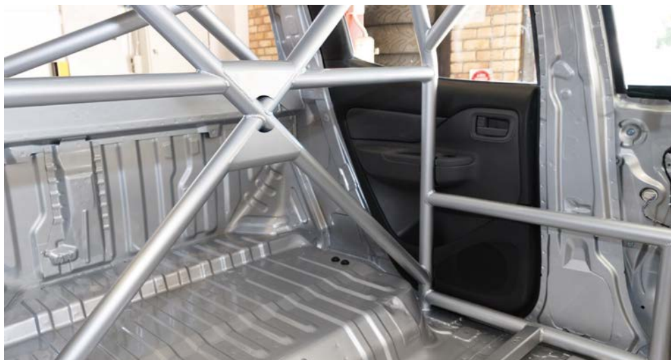
The rollcage is a standard component and stretches back in to the dual-cab space. The full parts kit will cost $60,000 AUD
