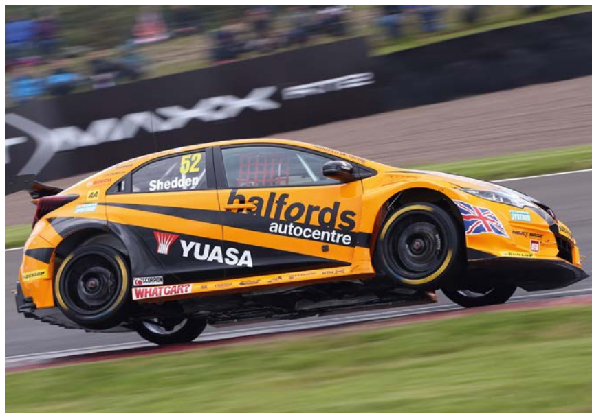
Touring car wheels need to be strong enough to cope with cars twice the weight of single seaters, while they will often get a bit more abuse too. Kerb strikes can impact the high stress areas around the end of the spokes
