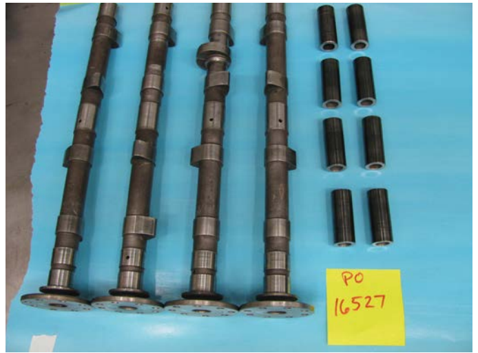
P3 camshafts. As the head is symmetrical each port could serve as exhaust or intake. These were switched from the 8C 2300 spec, with intake moved from the right to left
