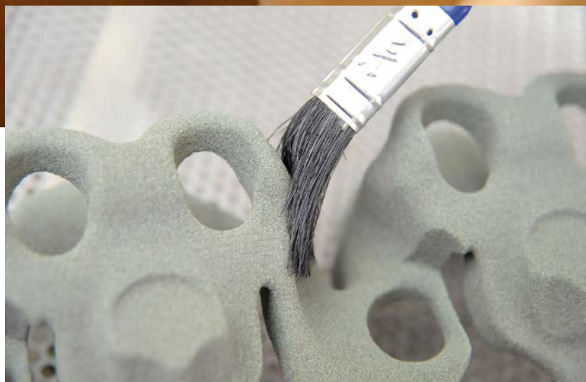
Main pic and above: sand printing has allowed the manufacture of the intricate shapes needed for modern race engines while maintaining the strength for the sand cores to survive 700degC of molten aluminium
