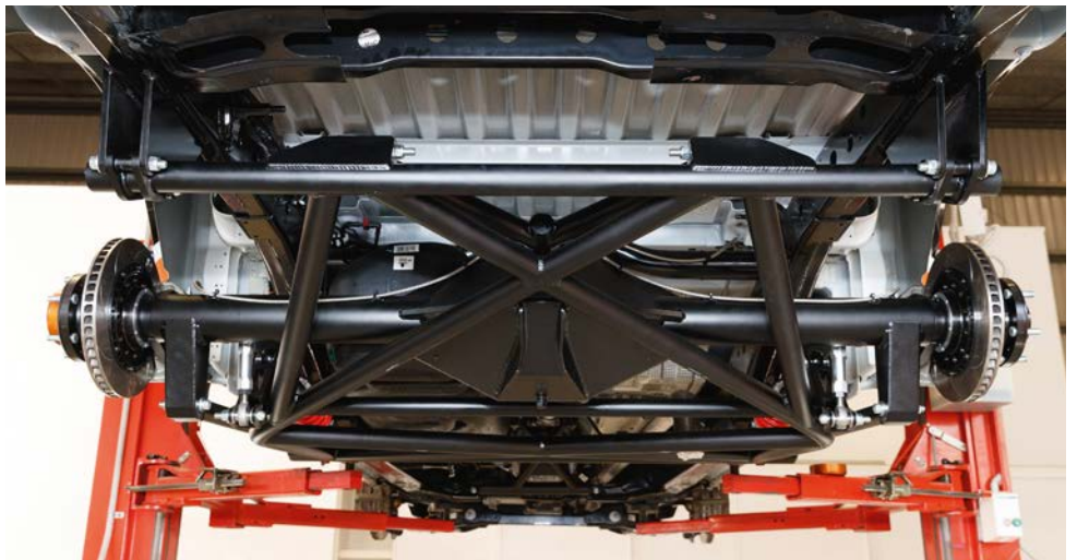
Supercars series preparation specialist Pace Innovation has designed and produced a spec rear axle housing as part of the SuperUtes package. It incorporates the damper mounts and the rear anti-rollbar while the mounting is common as well
