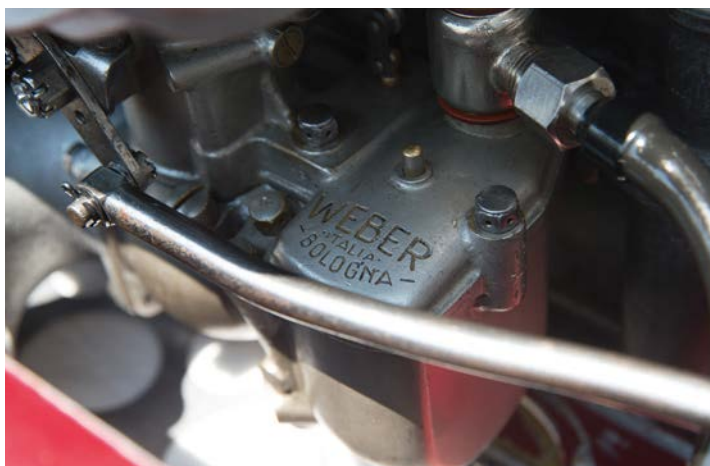
Weber carbs are fitted above superchargers, feeding petrol from a 140-litre fuel tank that is fitted in the tail of the car. There is also a 20-litre oil tank for the dry-sump lubrication
