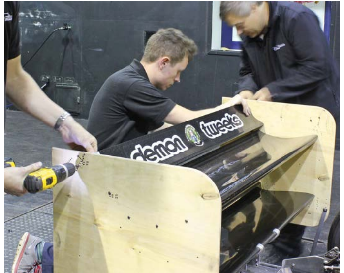
The new Firestorm's upper rear wing tier had a higher downforce main element than the original car's baseline set-up. It makes use of the legal maximum span of 1400mm
