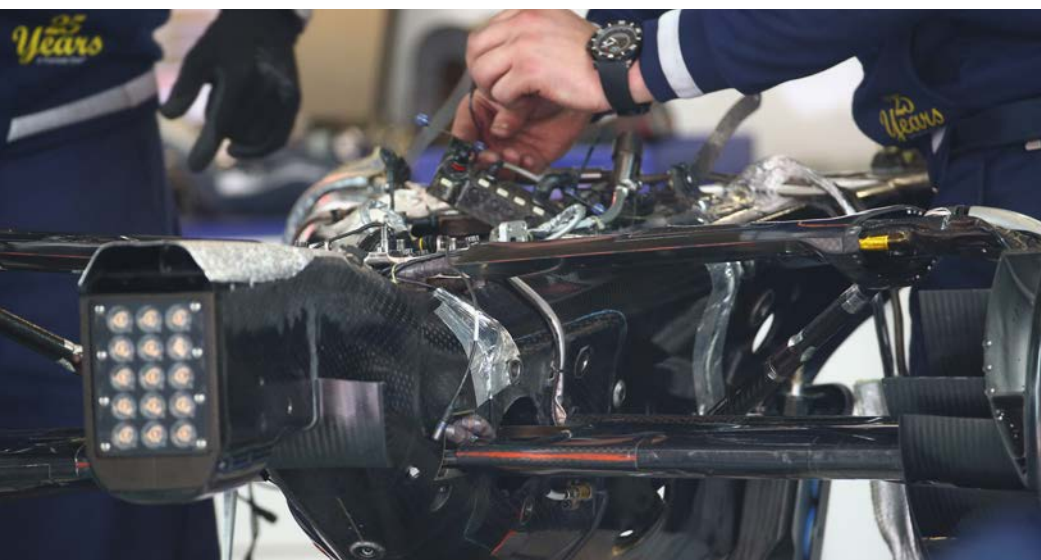
The C36 also uses the 2016 Ferrari transmission, though in this case modifications did have to be made to cope with loads
