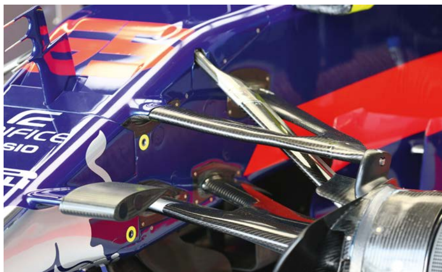
Front suspension members had to be significantly stronger than in 2016, resulting in a larger cross section
