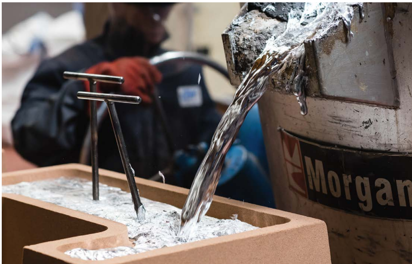
The molten aluminium needs to avoid exposure to air as much as possible and this is why the flow of the metal in the mould is controlled through some very complex gating systems
