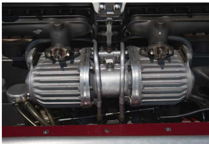
The Roots-type superchargers, each feeding four of the eight cylinders, are mounted laterally on the intake side of the powerplant and are also driven by the central gears
