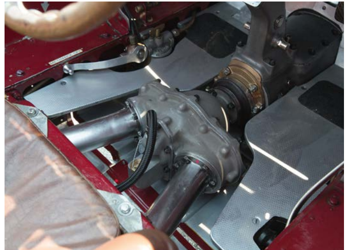
The 4-speed 'box sits between the legs of the driver with the stick protruding from it. The differential is bolted directly to the gearbox and is also situated in the P3's cockpit
