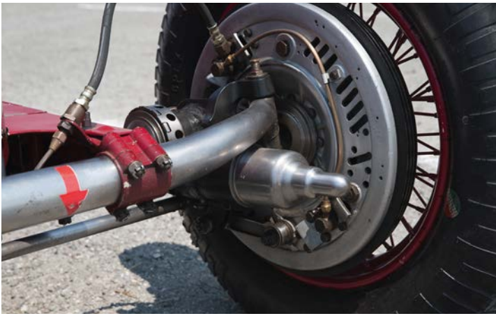
Dubonnet type front suspension consists of a rigid mounted beam axle with short trailing arms connected to the axle through kingpins, plus internally mounted spring and damper
