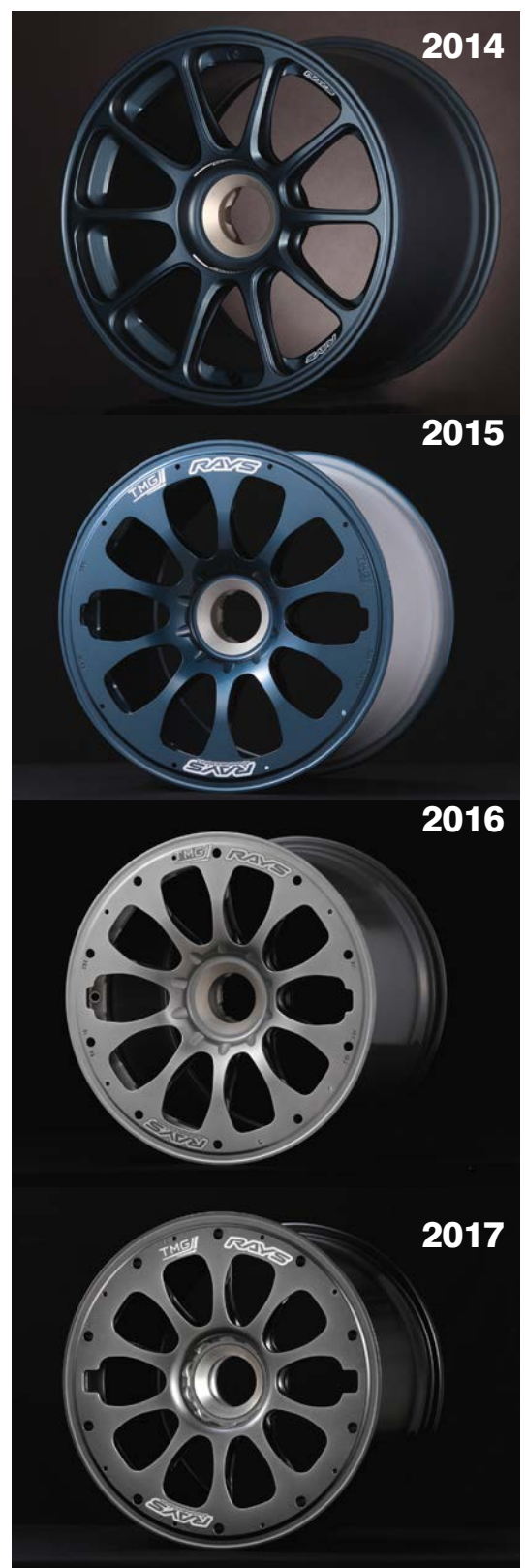
The Toyota LMP1 wheels have been developed by Rays and over the last three and a half years have gone through over 30 iterations. This year's features the widest fairing yet, which is designed to aid the attachment of the airflow around the wheel
