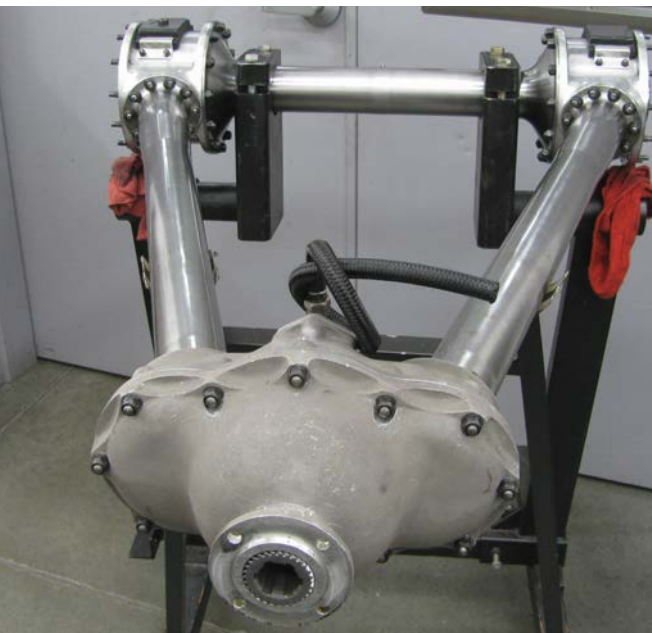
The bifurcated drive system removed from the racecar. This consists of a pair of propshafts connected to a centrally mounted differential
