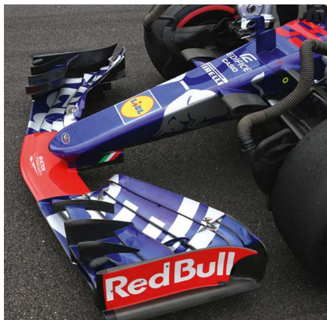
Nose is very similar in concept to the Mercedes, though STR12 uses an array of NACA ducts on the underside while the W08 uses a large scoop
