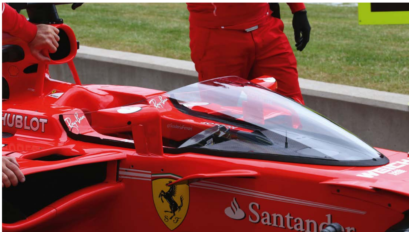
Questions were raised about driver egress from the tight cockpit opening created by the sloping sides of the Shield. Two different shaped versions of the device have been produced
