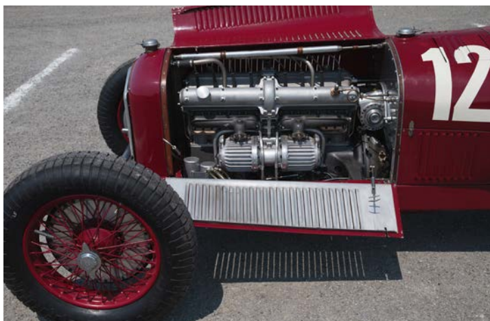
The quite beautiful twin-cam 8-cylinder powerplant was bored out from 2.9-litre to 3.8-litre during 1935 season. It was then delivering an impressive, for the time, 330bhp at 5400rpm
