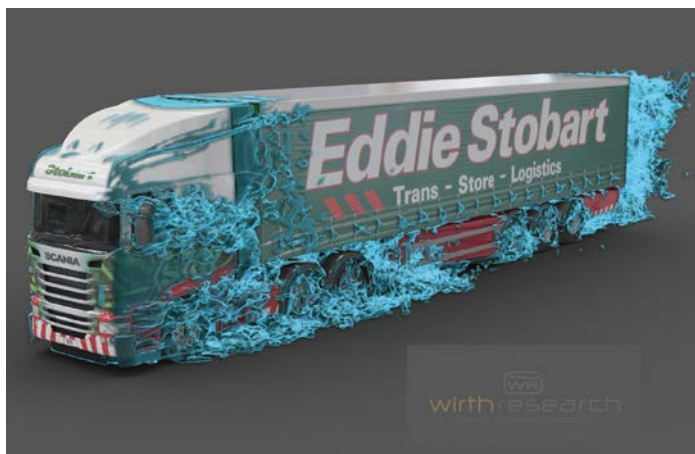
Steady and unsteady CFD simulations provided CO2 emission reductions and economy improvements for Eddie Stobart, and over 400 of its trucks now sport WR's aero kits
