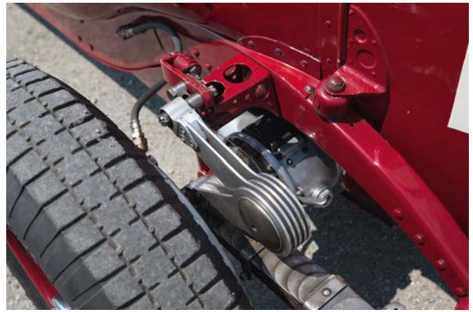
At the rear quarter-elliptic leaf springs were fitted by Ferrari and one of the friction dampers was substituted with a hydraulic shock. The drum brakes are also hydraulic
