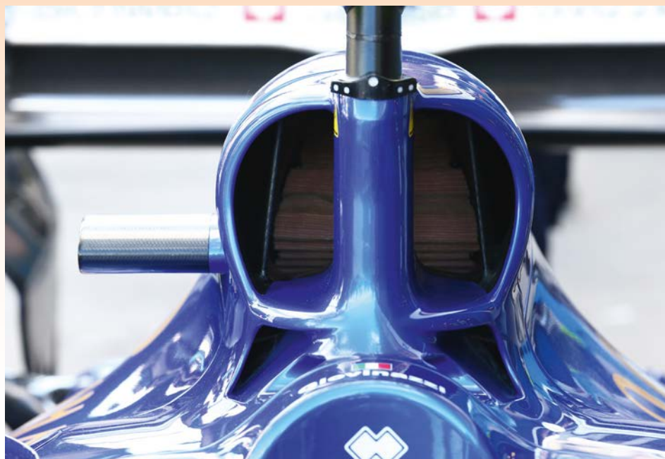
A single upright blade helps divide the air through ducts that feed in to the Ferrari V6 ICE and to the Sauber C36 coolers
