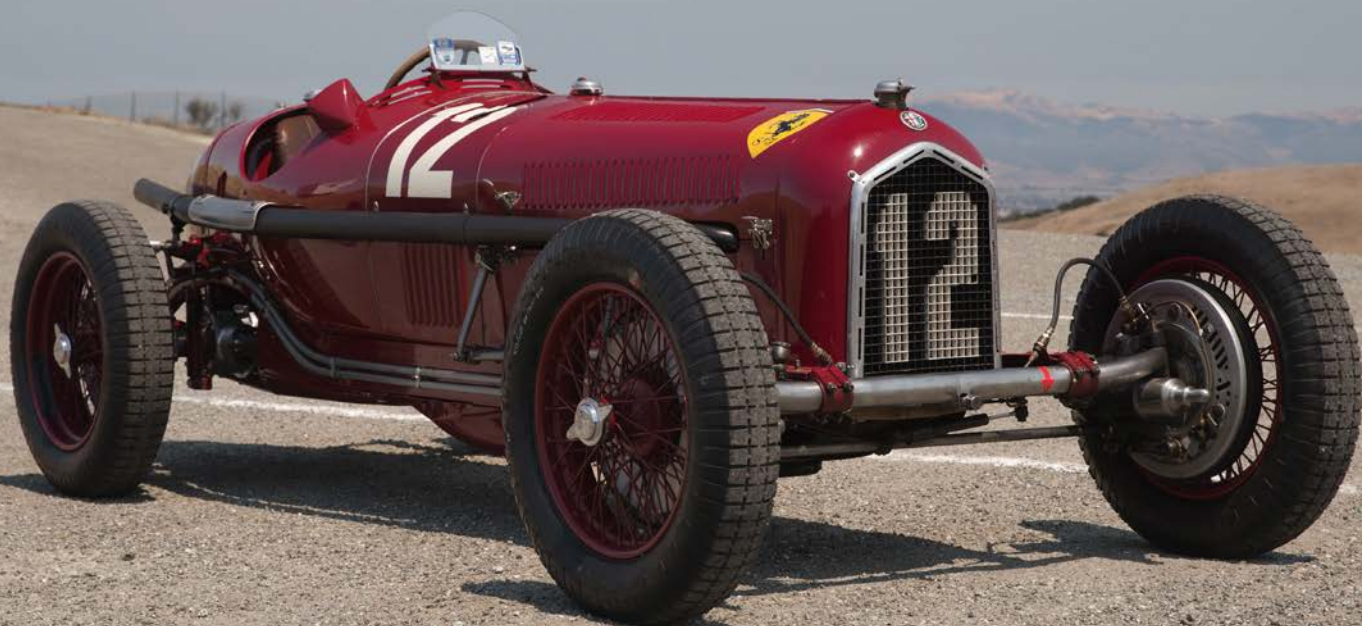
The aluminium body was tightly wrapped around the car's running gear. The P3 was widened to meet the new grand prix racing regulations that came into force for the 1934 season
