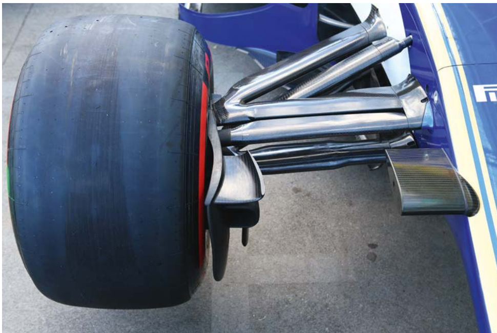
Higher 2017 loads mean beefier wishbones. Making sure the tyres are in the right operating window has been a challenge
