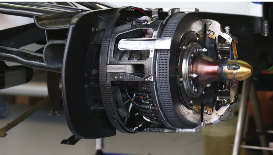
Front brake. Stopping is courtesy of Brembo carbon pads and Carbon Industries discs. Brembo also supplies the calipers
