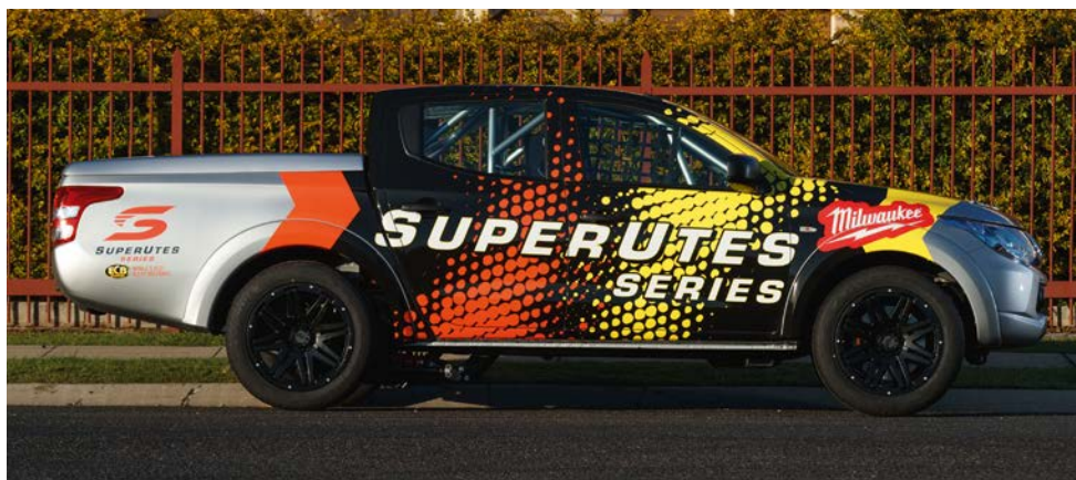
Ride height of these trucks is going to be huge, even in race trim there’s 80mm between top of the wheel and inner guard
