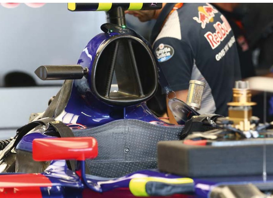
Roll hoop showing the segments in air intake. The central part is for combustion air to the Renault V6 while the side sections are for cooling. Toro Rosso introduced centreline cooling to Formula 1 in 2014
