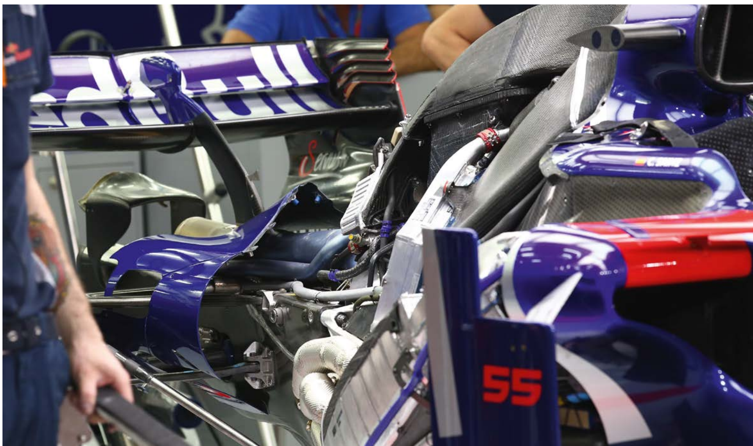
Bodywork removed to show the charge air cooler in the sidepod. Other coolers in centre of car allows it to run with smaller sidepods, with the aim of improving the aero performance
