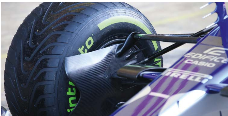
STR12 uses an unconventional front wishbone attachment. The wishbone actually ends slightly short of the upright and an extension then reaches outwards and rearwards to meet it. It is reminiscent of the Lotus 49 suspension layout from the '60s
