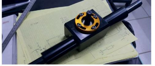
The new steering rack was tested on the older FVee cars at the race circuit to validate the design, as was the gear linkage
