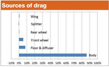
Figure 5: The splitter's contribution to the drag on our GT aero model was minimal
