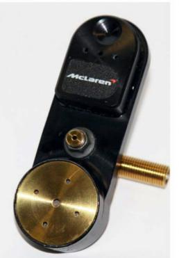
The TPMS sensor is located on the rim where the tyre bead seats. These not only measure tyre pressure but now also include IR elements to measure the temperature of the tyre carcass
