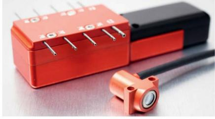
An example of an eight-channel aerodynamic wireless 8xPDIFF-WS sensor (back) together with the high temp INF-V4 sensor (front) from Texys. Wireless tech looks set to be the next big thing in the world of sensors
