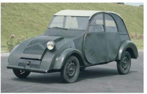
The first iteration of the 2CV was minimalistic in the extreme; note the single headlamp. Body steel was corrugated for extra stiffness
