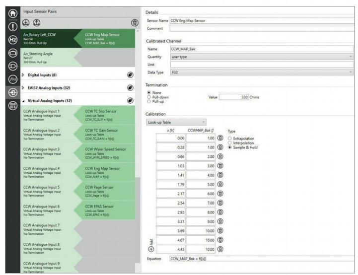
This is an example of how a direct output from the CCW is calibrated in a Cosworth system. Note also the CAN based signal used as a virtual analogue input, which can be calibrated in the exact same way. This would allow a redundant system to be created should an issue arise with either CAN or with direct wiring
