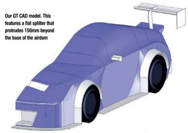
plitters feature on many different types of racecars, usually on closed wheelers although variations on the splitter and devices that function in a similar way can also be found on open wheel racecars. Typically, though, we see them on saloons/ sedans, sports racers and GT cars, protruding forwards from the bottom of the front airdam/bumper.
