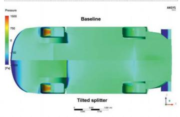
Figure 7: Tilting splitter generated more front downforce and helped rear underbody too
