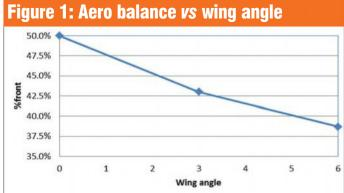
Wing angle versus per cent front shows how the wing altered the aerodynamic balance
