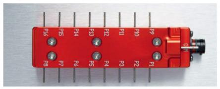
Wireless sensor with 16 channels. These work in synergy with custom designed tri-band auto-tuning systems
