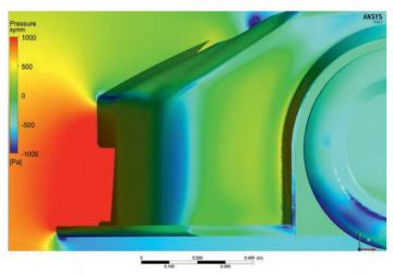
Figure 4: Pressures on the symmetry plane show the differential between top and bottom surfaces of the splitter, further illustrating how a splitter creates downforce
