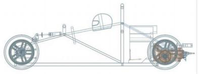
The initial layout drawing with all the major items placed. The new Formula Vee has been designed with robustness and ease of use in mind as it's also to be employed as a school car
