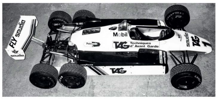
While the concept was all about drag reduction FW08B was able to find good ground effect downforce from this layout and it might have been raced without both front and rear wings
