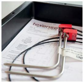
Pitot tubes are more visible than most sensors. They are usually mounted on the nose of the racecar and they measure the airflow
