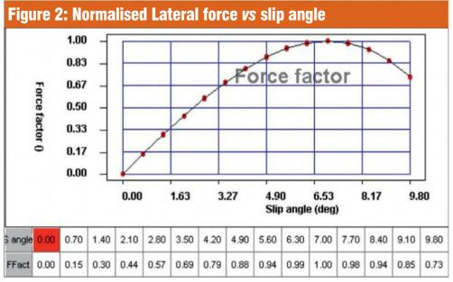
The second component is the lateral/longitudinal force vs slip angle/slip ratio, which is used with the traction circle radius
