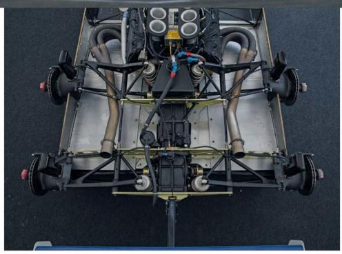
Main picture: The Williams six-wheel experiment began with the FW07D, on to which the four-wheel rear end was grafted. This retained the bodywork of the FW07C. The team then developed a six-wheel version of the FW08, called the FW08B Above: The gearbox was the key component. It featured a single input shaft at the front while the secondary shaft was connected on either end to the two LSDs. Twin rear axles also meant Williams could mount the rear wing further back
