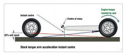
intersect to a vertical line drawn through the centre of the front tyre. If that point is below the centre of gravity that is your percentage of anti-squat, but if that point is above the centre of gravity I assume that it becomes lift?
