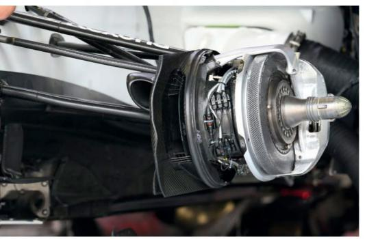
Brakes are AP Racing 6-piston front (above) and 4-piston rear calipers with carbon discs and pads. Wishbones are beefier this year to cope with the higher loads while cornering, which are a result of new-for-2017 aero regulations and wider tyres
