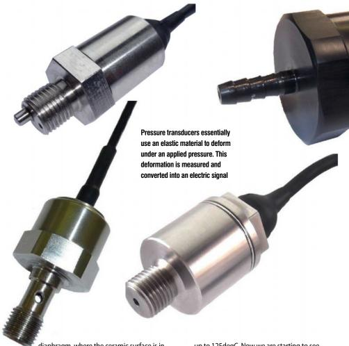
diaphragm, where the ceramic surface is in contact with the pressure media and on the back is a capacitive or resistive sensing element. We then have thin-film technology which uses a stainless steel diaphragm with a strain gauge embedded inside. Finally, our most accurate solution uses a silicon sensing element together with a stainless steel diaphragm.'
