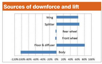
Figure 6: The splitter contributed downforce that was comparable to that of the wing
