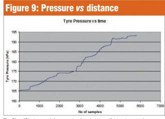
The ChassiSim tyre model can use track replay to predict tyre temp and pressures
