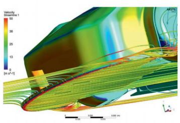
Figure 2: Air accelerating under the splitter generates most of the downforce
