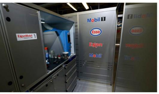
Red Bull garage lab has spectrographic analyser that picks up light signals from oil components and from metals in the oil
