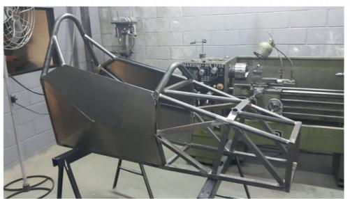
Main bulkheads were of rectangular section and perpendicular to chassis base, making for easier manufacture and jigging
