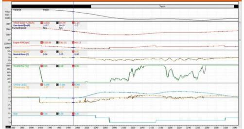
The extra detail is clear to see here. Note the near 1km/h differential on turn in and the 0.03s variation in the compare time
