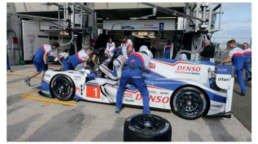
Toyota practices changing the FFM, located behind driver's door on LMP1 cars. Flow meters measure average flow in WEC
