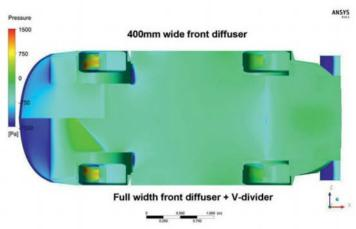
Figure 9: Full width front diffuser created yet more splitter downforce, but tradeoffs meant there was no overall improvement over the 400mm wide diffuser
