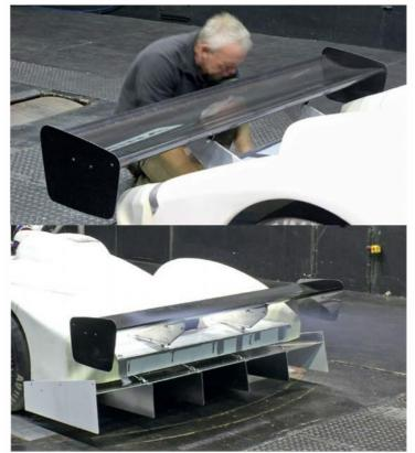
**Top and above:** The Sabre's new single element rear wing was mounted low and well back and it overlaps the trailing edge of the racecar's extended bodywork and the rear diffuser
