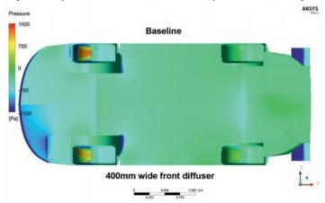
Figure 8: This clearly shows that front diffusers added significant splitter downforce
