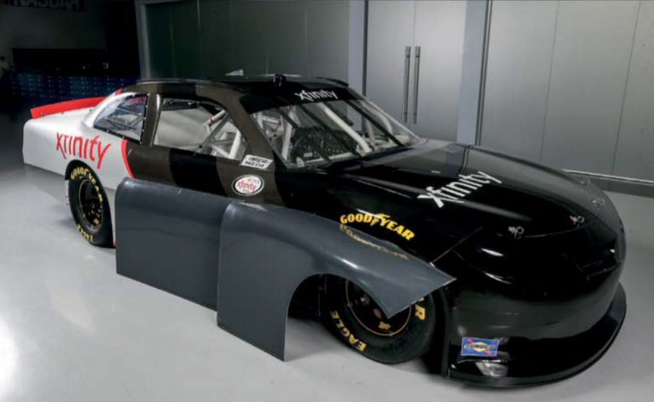
Above: The new inspection system is capable of scanning the entire body and determining camber and toe within 90 seconds Left: The ongoing switch to composite bodies in the Xfinity Series is a major change. Two of the 11 flange panels are shown here
