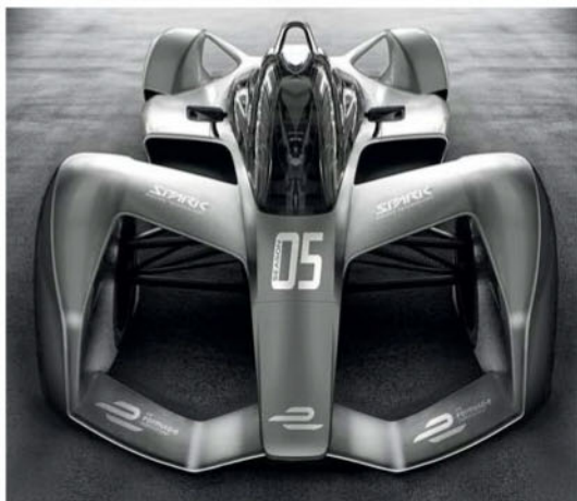
Conceptual rendition of season five car. While it may not look quite like this, it will have a large venturi at the rear rather than a conventional rear wing, plus a one-piece frontal bodywork section
