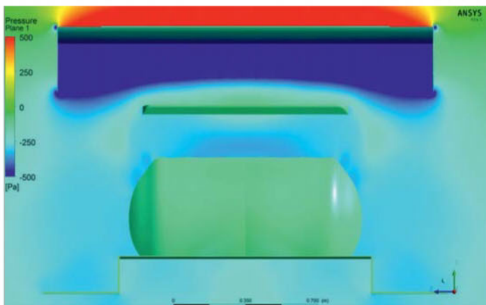
Figure 19: The diffuser footplate also saw lower static pressure above it than below it
