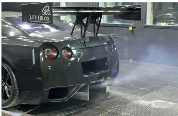
The smoke plume shows organised energetic flow from the centre of this diffuser ...
