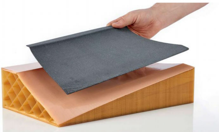
FDM technology can create the tools to help manufacture composite parts within a few days, rather than a few weeks
