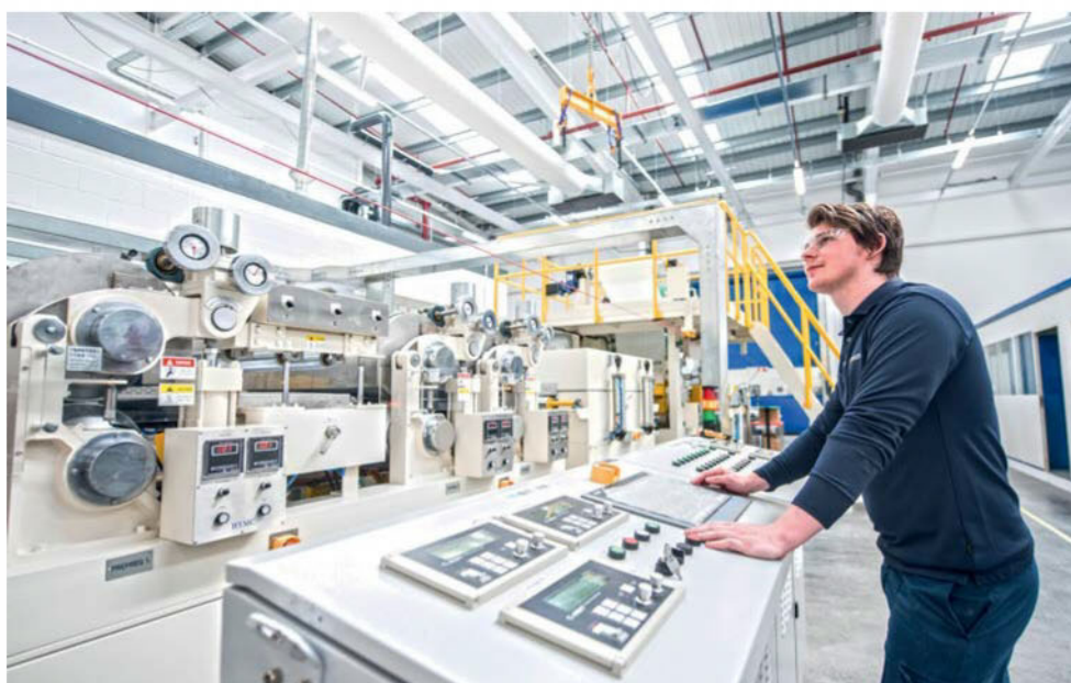
A uni-directional prepreg machine. This material is ideal in applications where strength is only required in the load direction
