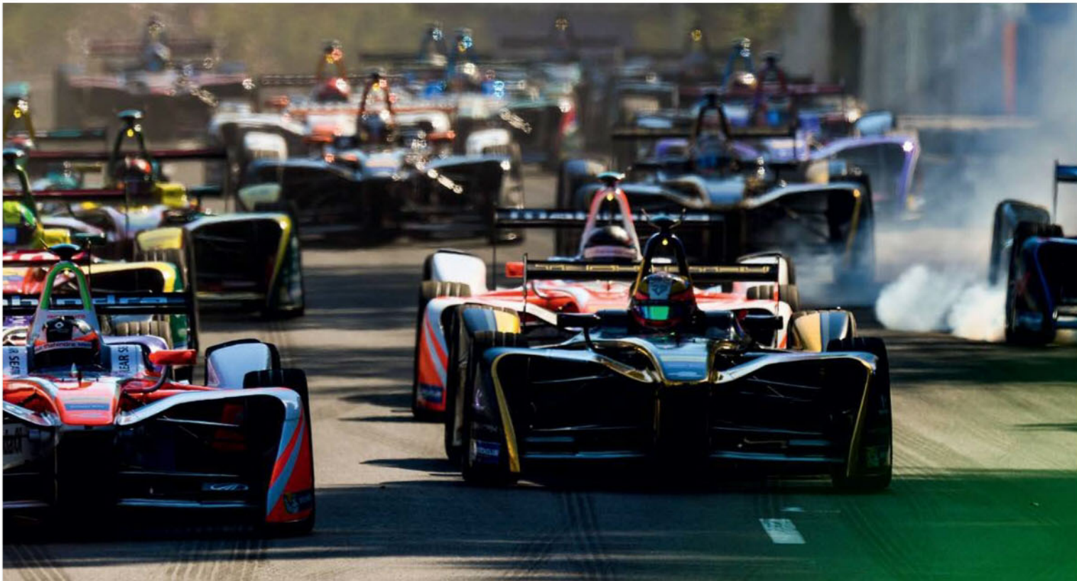
Lower downforce in Formula E compared to Formula 1 results in less drag and therefore a smaller wake, so the racecars can follow each other closely, which can mean better racing
