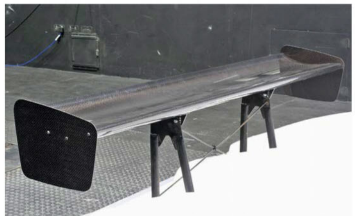
Higher location restored balance but not efficiency, and lost interaction with underbody
