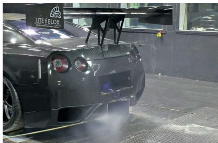
... and then a disorganised and even a reverse flow of smoke behind the outer diffuser
