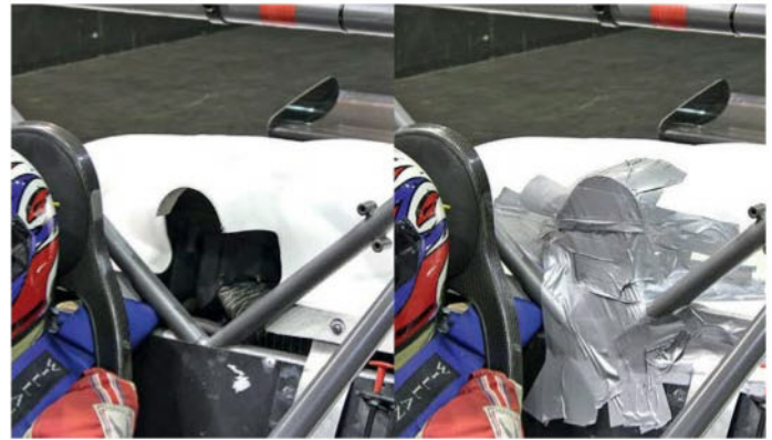
Redundant inlet duct cowl (left) was cut off and taped over (right) with modest gains
