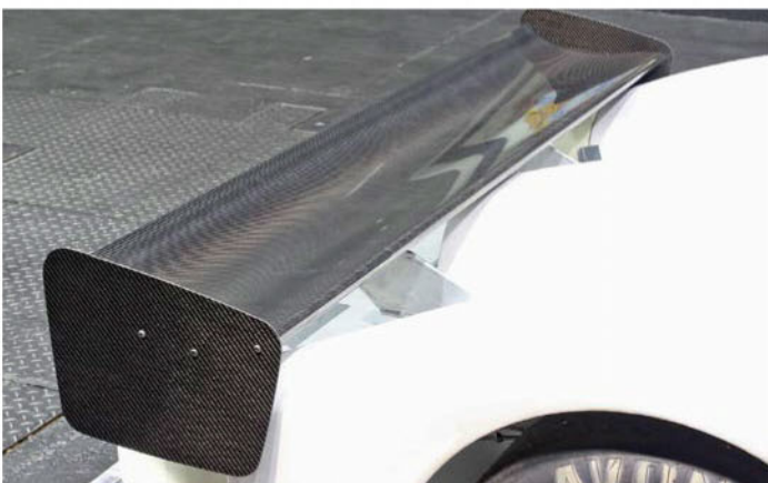
Moving wing 170mm forwards had resulted in a 37 per cent reduction in rear downforce
