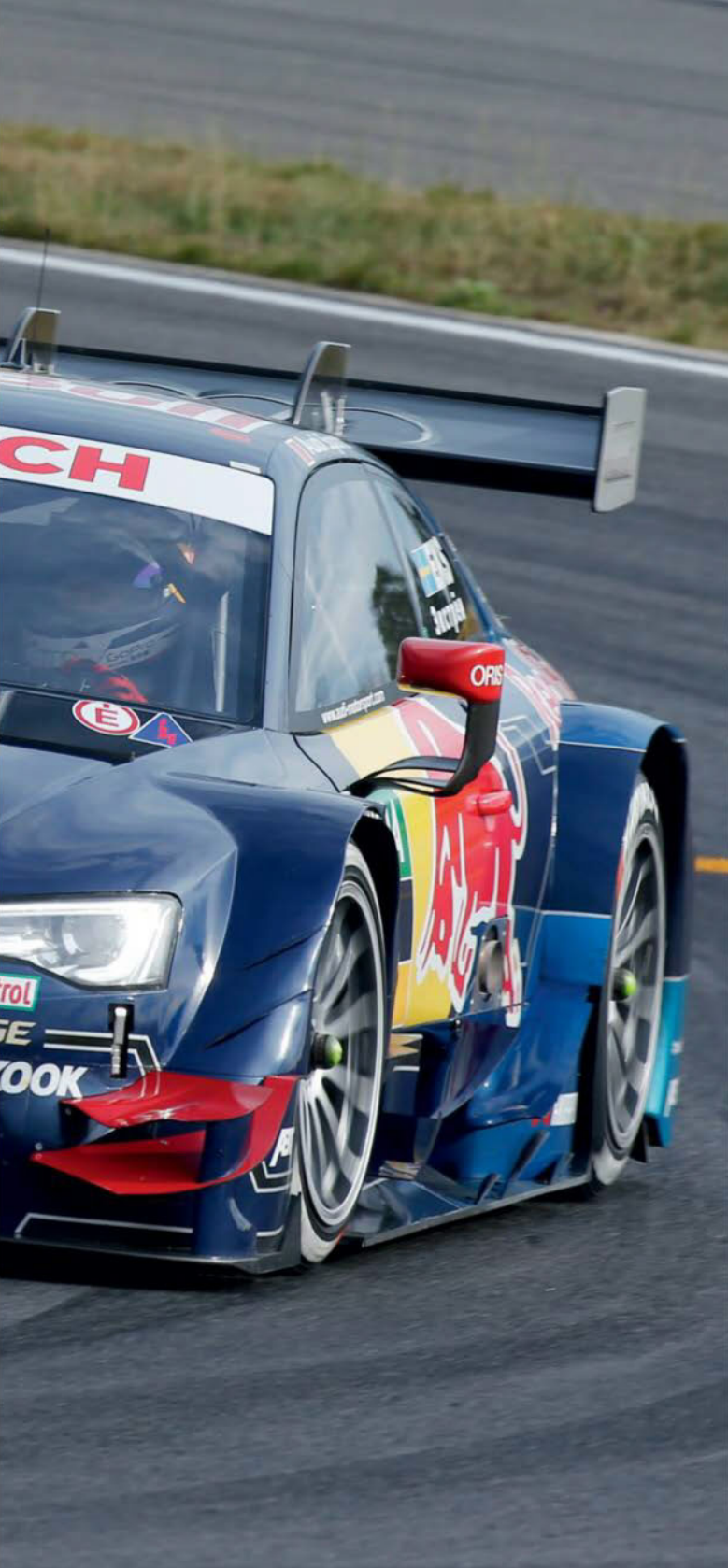
Mattias Ekstrom in his office. Unlike the headrests on F1 cars the DTM device is further away from the driver, allowing more kinetic energy to build up before the head hits it
