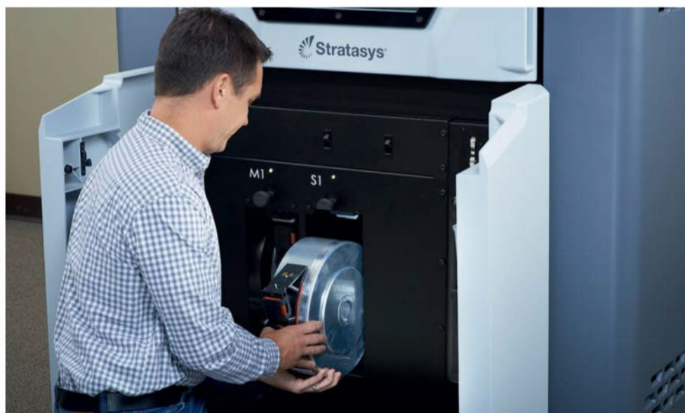
The filament used in FDM is supplied in cassettes, such as the support material cassette S1 that’s shown here. Stratasys machines can now simultaneously print different materials and colours, requiring the use of a number of these cassettes
