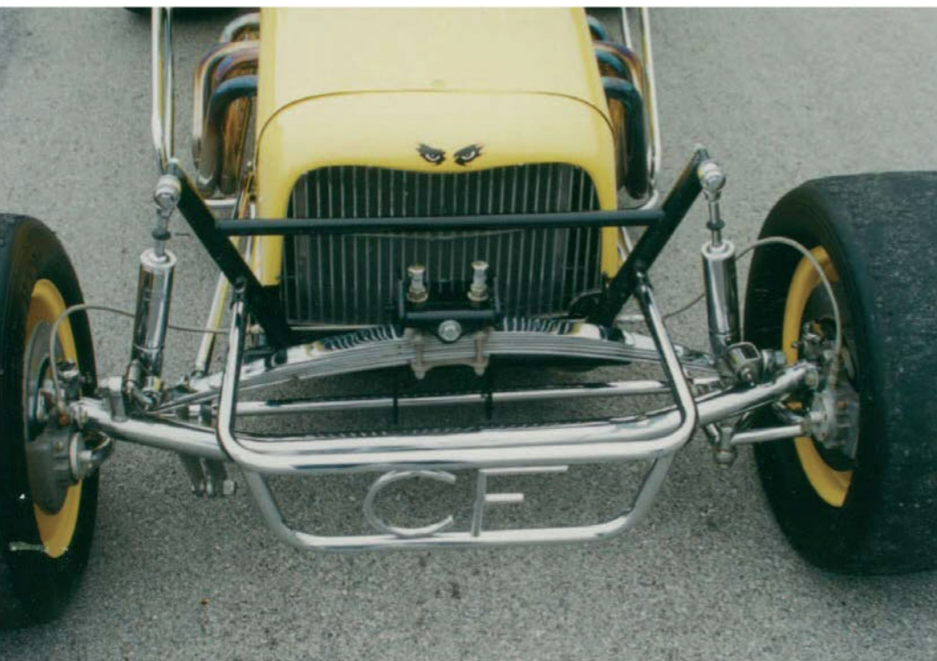
This crazy car has a beam axle on three longitudinal links and also a transverse leaf spring with a shackle on one end, then just an eye on the other. The question concerns the pros and cons of four-link and three-link suspension set-ups
