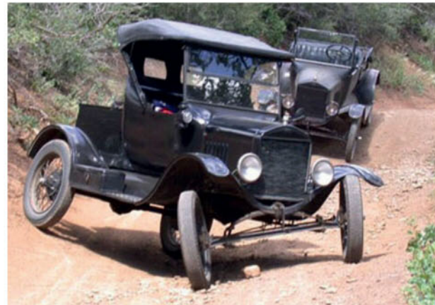
A Model T Ford in a condition of extreme warp displacement. Front roll centre is a little bit below the top of the leaf spring
