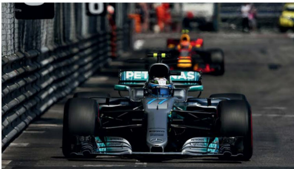
F1 aero development has led to complicated wings and flaps, in stark contrast to the cleaner lines of the Formula E racecar
