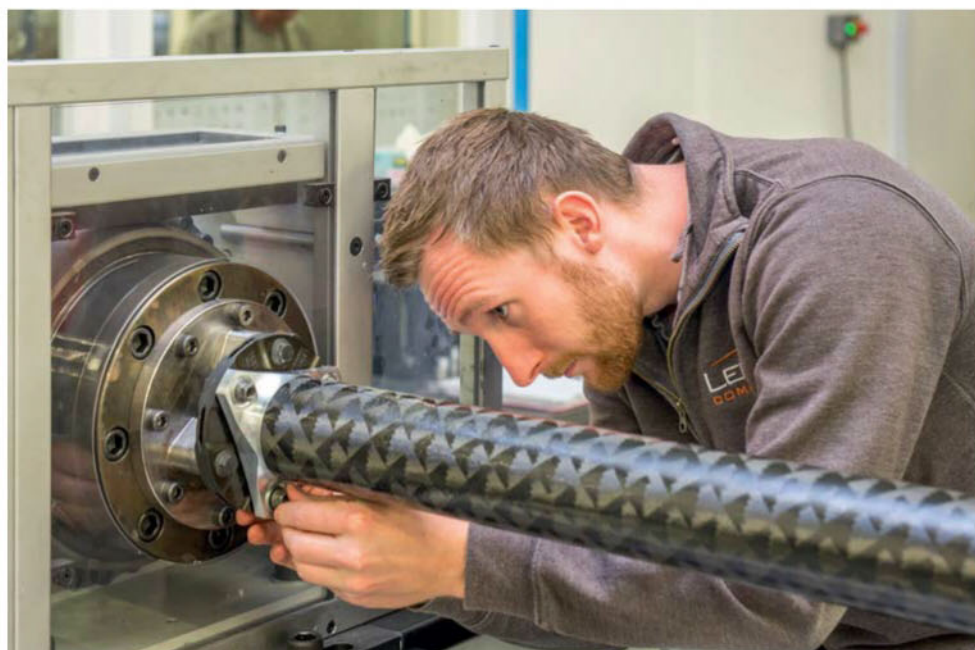
Composites are used for a wide range of components. This is a torque test for a thermoset composite transmission shaft
