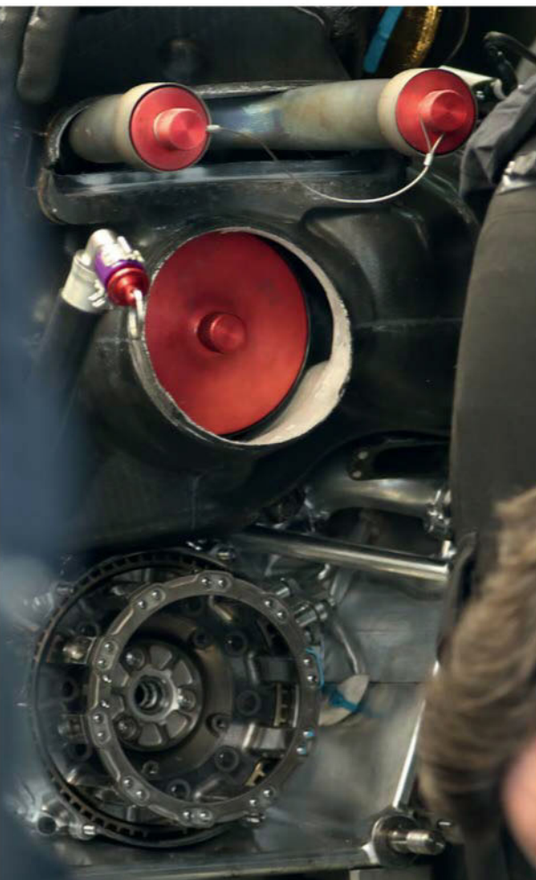
Exhaust exit from turbine with its red bung; clutch basket below it
