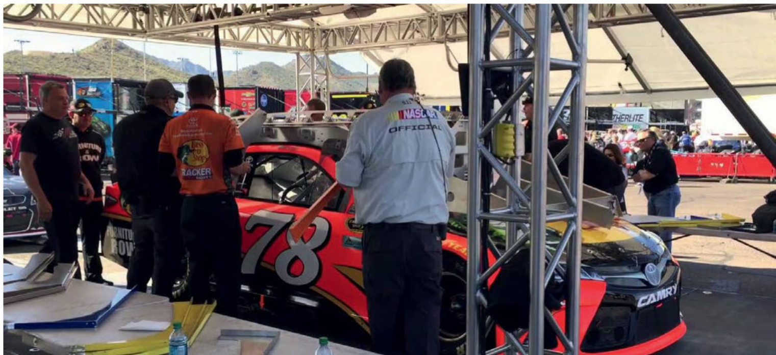
Above: NASCAR template inspection. Despite new advances in technology templates will still be used to check critical details Right: A wheel gun development war has prompted NASCAR to introduce a spec item with monitored line pressure and lug torque
