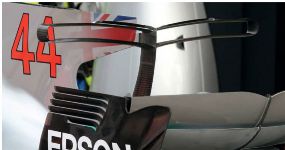
Mercedes was the first team to run the controversial T-wing. With the new aero rules there was scope for design creativity
