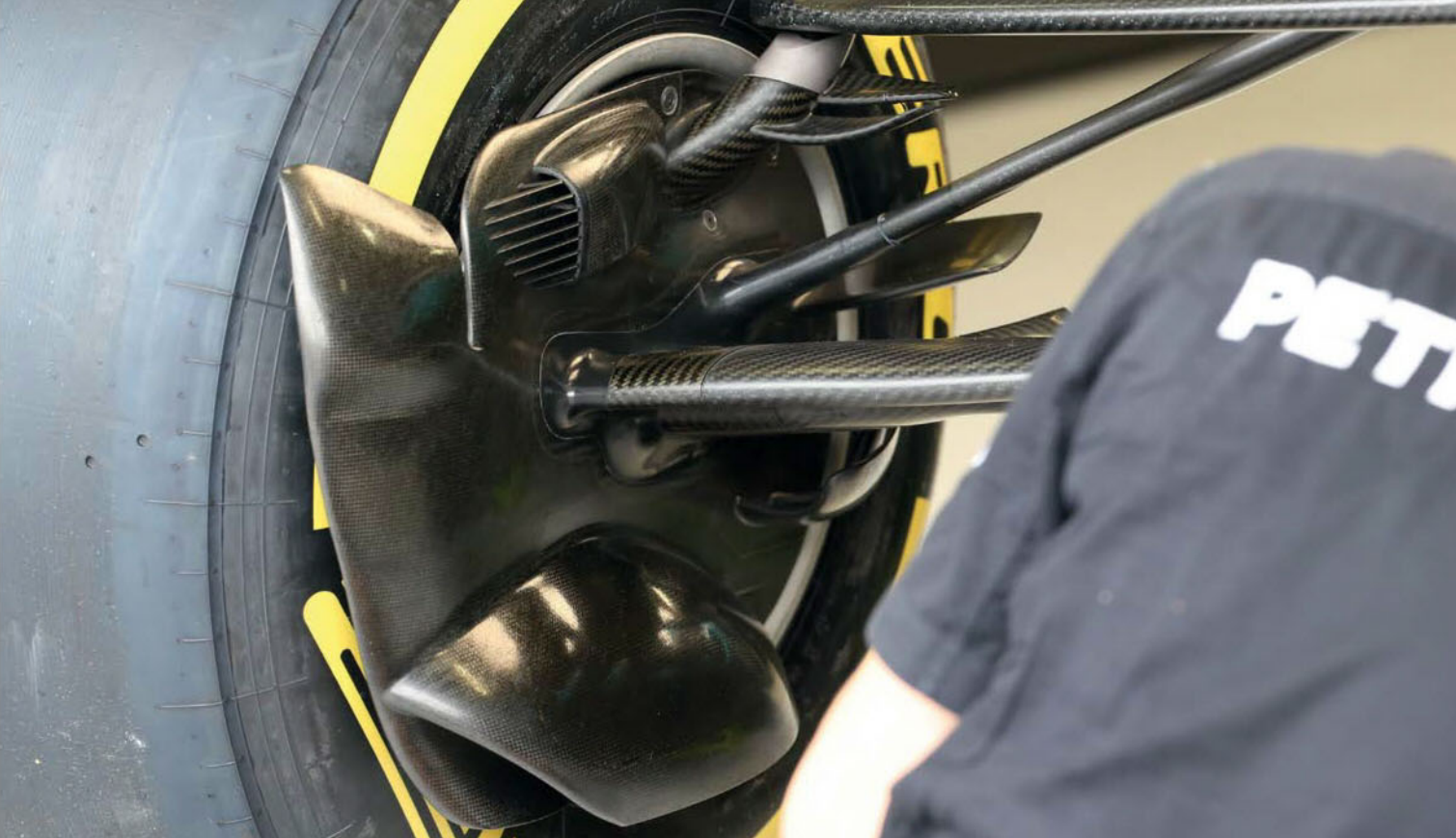
Above: The striking front upper wishbone treatment sees the pickup some way rearwards and inboard of the more usual location. Mercedes tells us this was not an aero development
