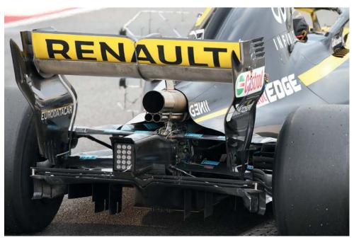
Renault is using its exhaust position to direct the plume so that it interacts with the underside of the rear wing main-plane
