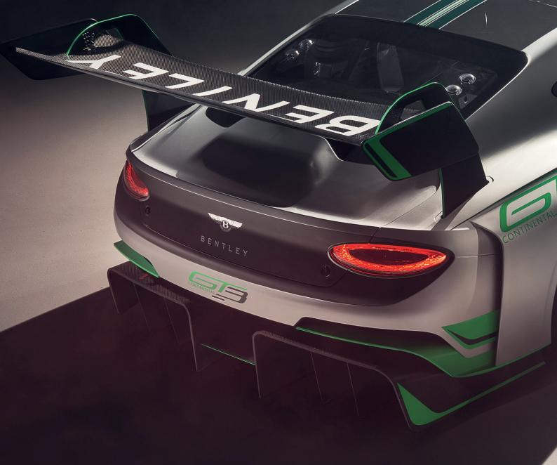
The GT3 looks imposing from any angle. Rear aero includes a new twisted rear wing and aggressive looking diffuser; actually less effective than older version because of position of new transmission
