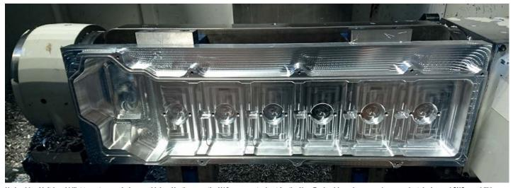
Underside of left-hand billet tappet cover during machining. Hartley sees the V12 as a great advert for the New Zealand-based company's powerplant design and CNC capabilities
