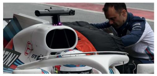
Williams uses centreline cooling. The 'A' of the roll-over structure is clear to see here. The outer segments of the intake feed air to coolers over the bellhousing, while the centre portion is for the air to the internal combustion element of the power unit
