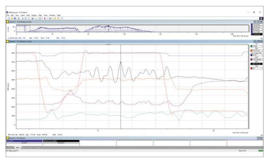
Figure 3: From this you would have to conclude that it's not sparking correctly and that this is the cause of the misfire
