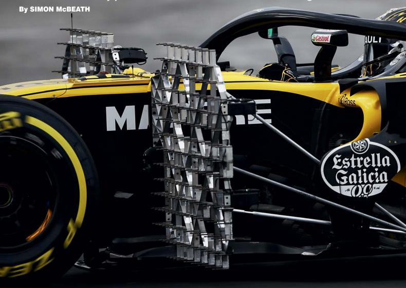
hotographs of pre-season and pre-race testing often show top race teams, especially in F1, measuring aerodynamic pressures around their cars. The most obvious manifestation of this is the pressure sensor array, like a two-dimensional rake with pressure sensors arranged over the area of the rake, positioned on the raceccar in key areas where what might be described as partial plane pressure plots can be logged and recorded.
