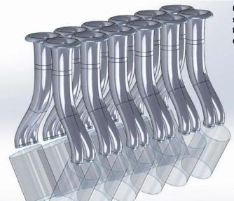
**CAD** rendering showing the inlet tracts relative to the cylinder positions
