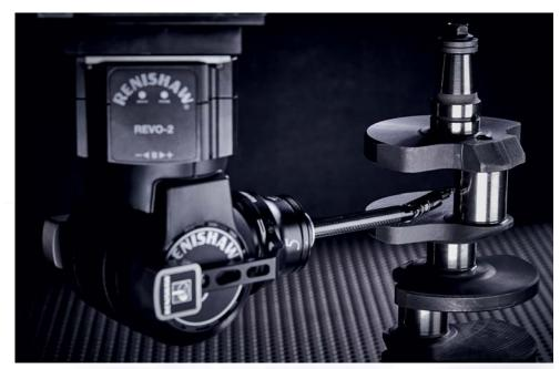
Measuring surface roughness has traditionally been seen as a black art but with Renishaw's SFP2 probe the roughness of a surface can now be measured in a controlled way, ensuring the smooth surfaces essential for engine components
