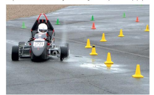
Competing in the wet is about more than simply considering the reduced grip - for instance, brake fluid is hygroscopic and so this needs to be flushed out and replaced after the racecar is taken out in the rain
