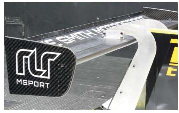
Wing angle is adjusted by fitting different brackets between swan neck plates and wing
