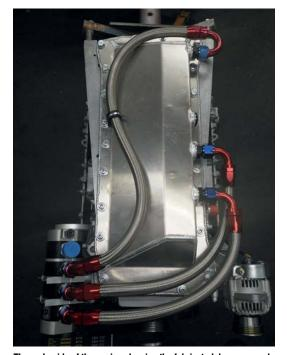
The underside of the engine showing the fabricated dry sump and the oil pump feed and return. All the work is high-end specification
