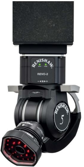
Vision probes can also be used on 5-axis coordinate measurement machines. These are non-contact, allowing the measurement of 0.5mm diameter holes, for example. A 1.3 mega-pixel global shutter CMOS sensor and digital signal processor are used and then the grey-scales of the images translate into spatial data
