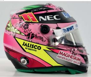
An F1-spec crash helmet weighs just 1.25kg and fits precisely, thanks to the 3D scanning of the driver's head before it's made
