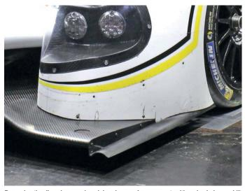
Removing the dive planes reduced drag by over four per cent, with a nice balance shift
