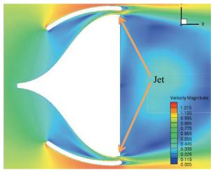
Above: Greg Woyczynski has suggested in an academic paper that the use of a duct on the leading edge of the wing mirror housing might be a good way to cut drag Right: These CFD images show the difference the internal shapes within the mirror's housing can make on the airflow
