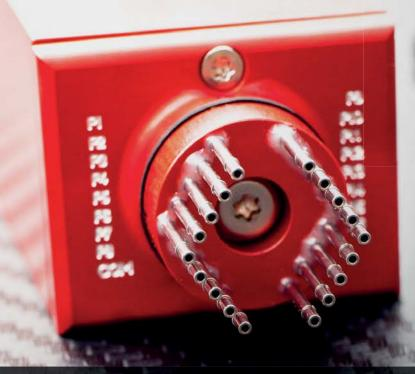
"Our aerodynamics sensors measure air speed by integrating dynamic and static pressures. This measurement combined with load measurement from our strain gauge bonding & XN4 series of amplifiers enables vehicle aerodynamics to be enhanced"
