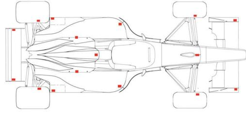
Figure 2: A distributed pressure sensor system vastly reduces the length and complexity of the tubing and installation. It puts local scanners at the point of measurement, with the tubing installation then connecting via a single CANBus cable to the nearest node
