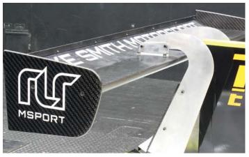
Steeper wing angle. It was possible to shave drag from the car with wing adjustments
