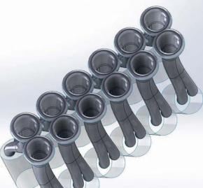
Top: The engine itself is based on a 5-litre Toyota 1GZ-FE. This powered the Toyota Century limousine from 1997 to 2016 Above: CAD rendering showing the top view of the inlet tracts relative to the cylinder positions. Hartley uses Solidworks CAD
