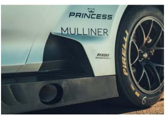
New sills increase the floor's width and are also designed to help brake cooling
