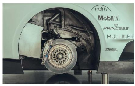
New body means the suspension pick up points are different and this has impacted on the car's kinematics
