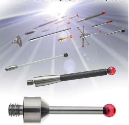
There are many different stylus combinations to suit any application or component. The stems are often made from carbon fibre while tips are usually ruby balls, as this is one of the hardest materials. Ceramic or tungsten carbide tips are also used
