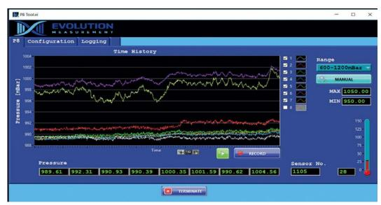
Figure 3: Screenshot of EvoScann GUI. Device has an onboard integral microprocessor so the output is in engineering units of pressure
