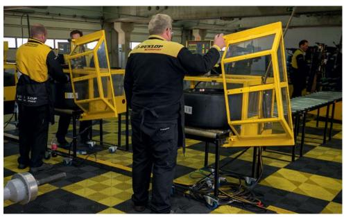
Once the new tyres have been fitted to the wheel rim they are then pumped up to pressure in these special safety cages
