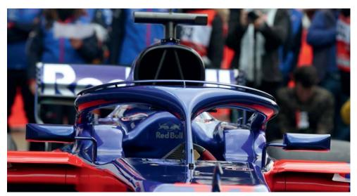
Toro Rosso introduced the centreline layout. It's clear from this image that the Halo could have an impact on a car's cooling
