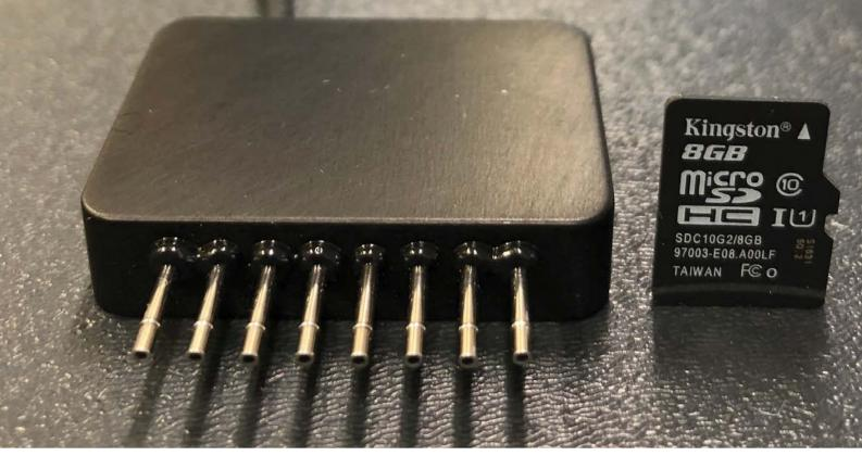
FS-PR8 is the smallest 8 channel absolute pressure scanner available for motorsport Its super light weight compact rugged design allows it to be mounted and used in harsh motorsport environments.
