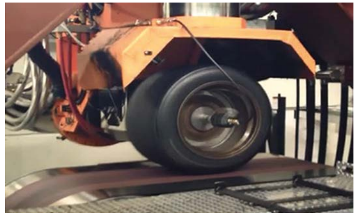
Figure 4: The test; the tyre is steered to a given slip angle then held there
