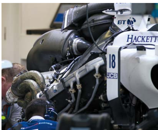
The FW41 uses the centreline cooling philosophy which is a feature of all the Mercedes powered Formula 1 cars this year
