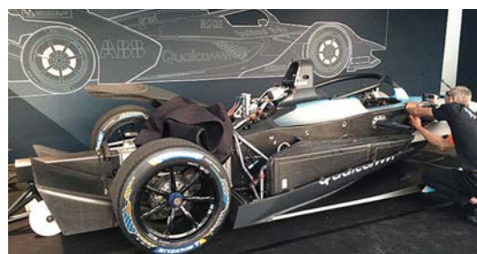
The Gen2 car weighs in at 900kg, which is an increase of 100kg over its predecessor, while it also has a higher centre of gravity
