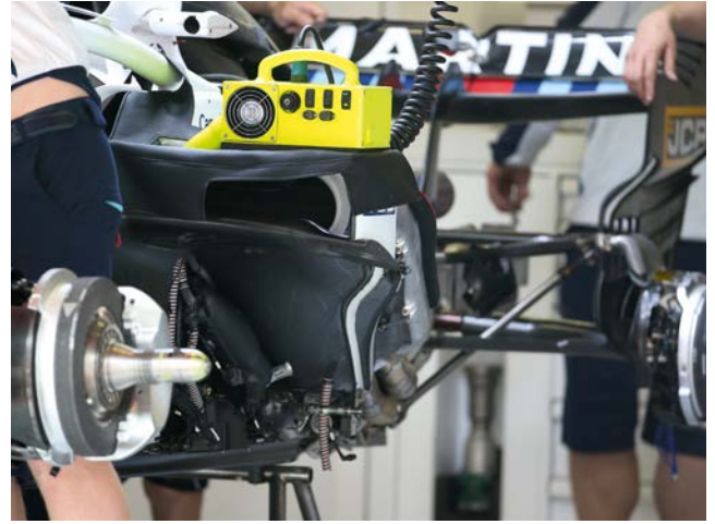
The undercut sidepods shown with the bodywork removed; note the low position of the side impact structure. The FW41 has the largest undercuts in Formula 1
