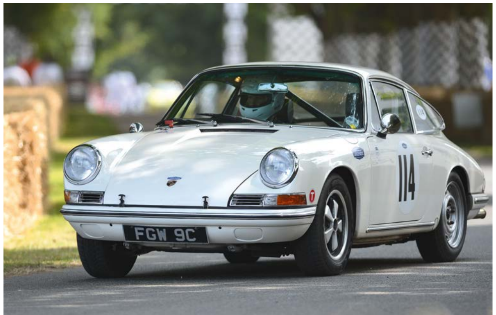
With older rear engine cars it is necessary to have a disproportionately large share of the lateral load transfer at the front end
