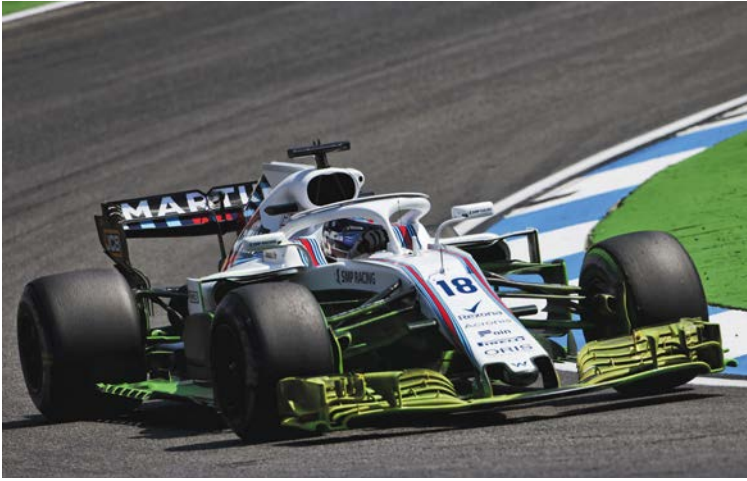
FW41 has often been seen covered with bright splashes of flow visualisation paint as the team tries to understand its aero issue. This mainly involves the floor stalling in an unpredictable way
