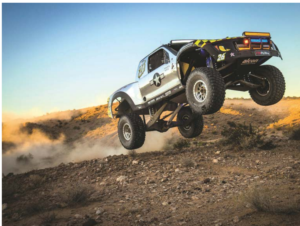
While 180cpm or even greater will suit racecars with proper downforce, off-road applications require much lower frequencies
