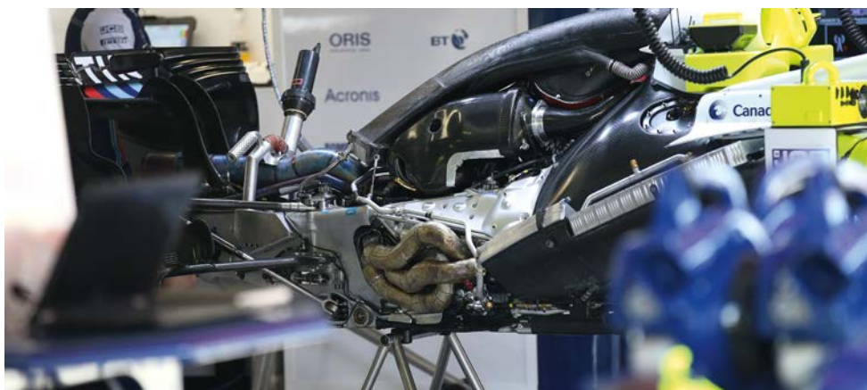
Mercedes power unit installation in the FW41. Paddy Lowe says there is more to be gained with aero than PUs this season
