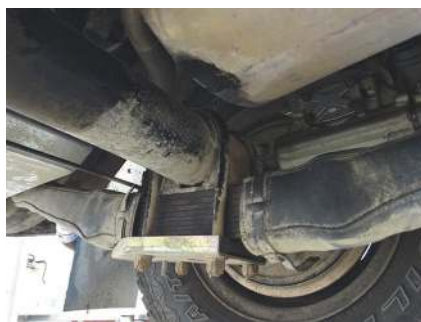
The car sits higher than standard, aided by heavy-duty rear leaf springs
