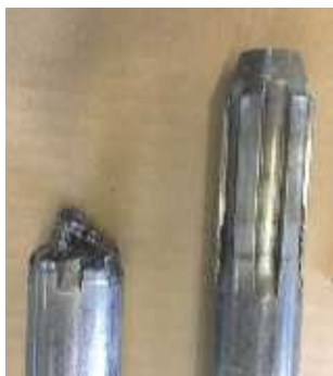
The offending broken driveshaft and stronger replacement part.
