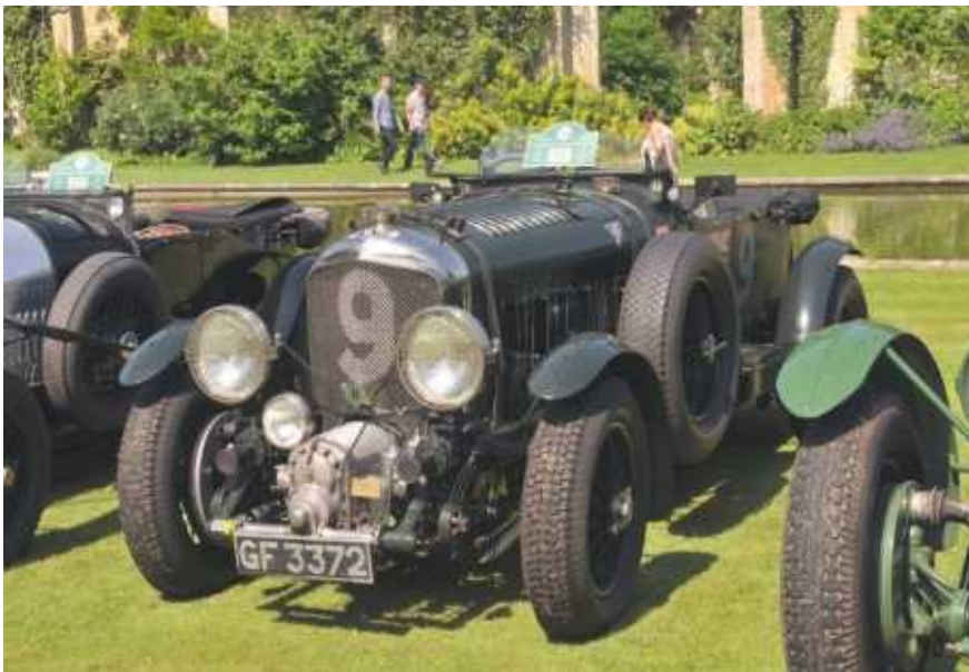
Ron Warmington's 1929 'Birkin Blower' is the real deal, with its Amherst Villiers supercharger.
