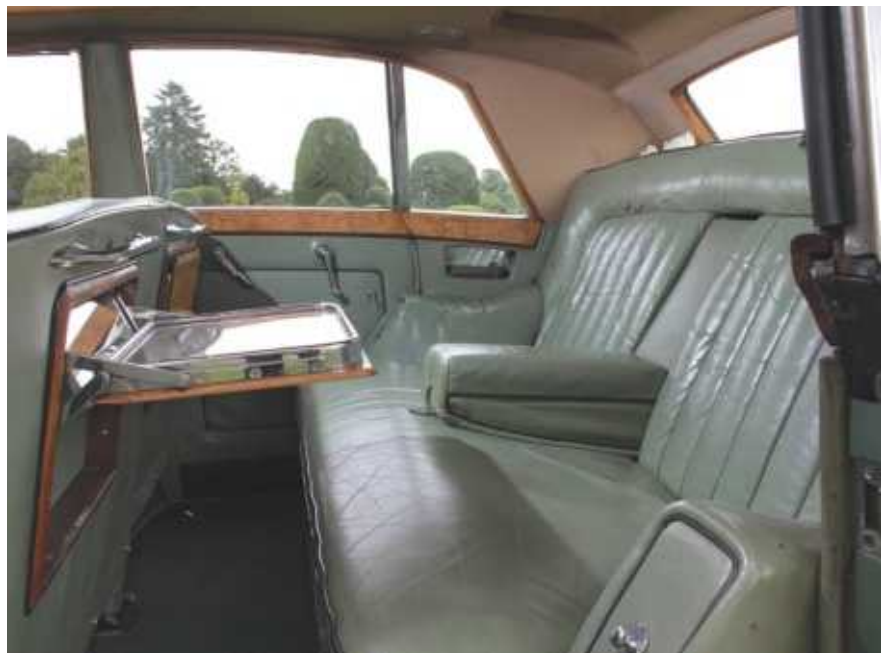
The rear seating area was designed to accommodate the chauffeur-driven super rich. Centre armrest can be lifted up to seat three in the back. Rear picnic tables include a vanity mirror. Note the driver's seat back is separate and has rake adjustment.
