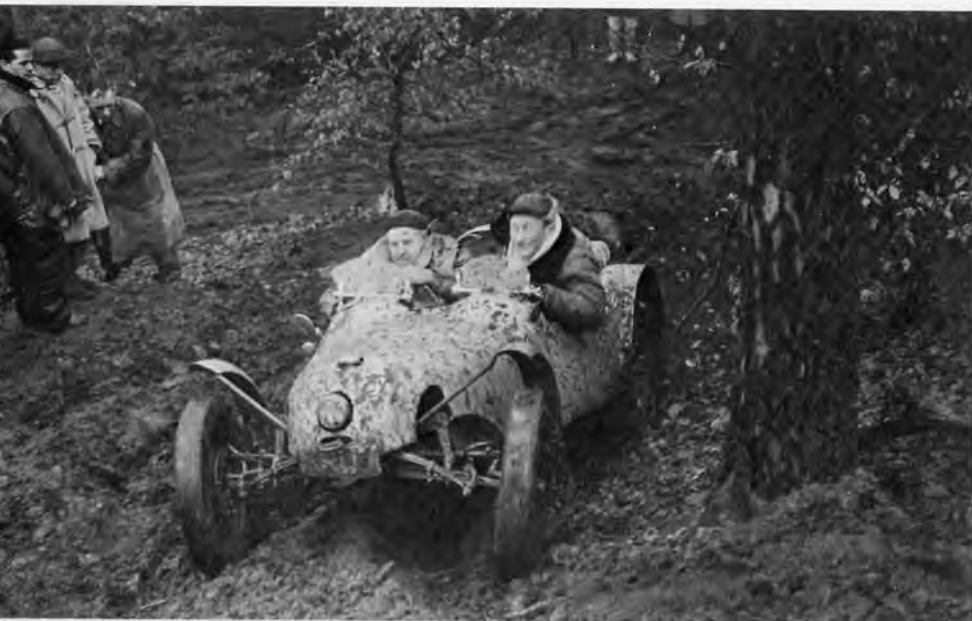
Trials: S. J. Onslow Bartlett's special of 1952 was distinctly unusual in employing a rear-mounted JAP V-twin engine. Photo: Autosport
