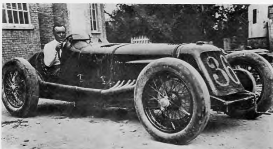
1929 Maserati Tipo V4 16-cylinder car. Borzacchini at the wheel. Photo: Cyril Posthumus Collection
