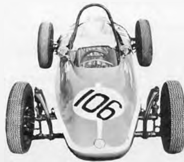
Formula Vee: clothed and unclothed views of a typical Formula Vee car, showing the standard VW suspension Photo: Doug Nye
