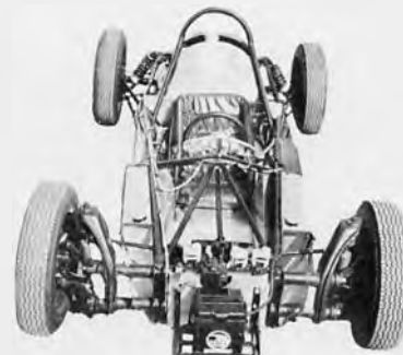
Formula Vee: clothed and unclothed views of a typical Formula Vee car, showing the standard VW suspension Photo: Doug Nye
