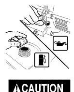
Never fill fuel tank completely. Fill tank to 1/2" below the bottom of the filler neck to provide space for fuel expansion. Wipe any fuel spillage from engine and equipment before starting engine.
