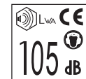
Noise emissions to the surroundings in accordance with the European Union's directive. The machine's emission is stated in the chapter TECHNICAL DATA and on the decals.
