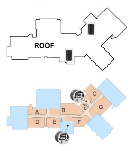
Install the ION Wireless Repeater on the roof (or similar location that is exposed to plenty of sunlight) to ensure proper operation of the solar panel recharging circuitry.
