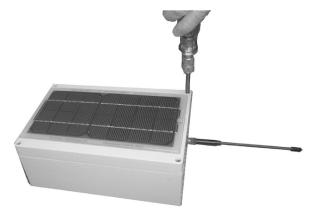
3. Lift the solar panel (lid), taking care not to damage the wiring. Disconnect the wire connectors that secure the wiring between the solar panel (lid) and the charging circuit board (in the chassis). Rest the lid on the ground.
