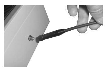
2. Remove the four screws from the front of the unit.
