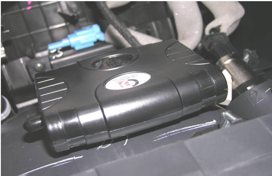
Figure 13: Ensuring the device is located with 30cm free radius
