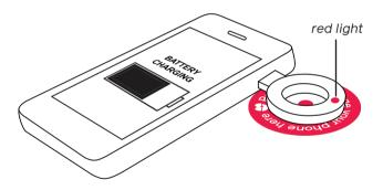
The red light on the Ring indicates ongoing charging and the red indication light on the charging area indicates that the Ring has been recognized by the Hotspot (placed correctly)
