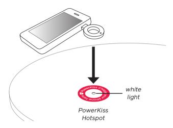
The indication light of the Hotspot should be white before placing the device to charge, if not, please wait for a few seconds for the light to change
