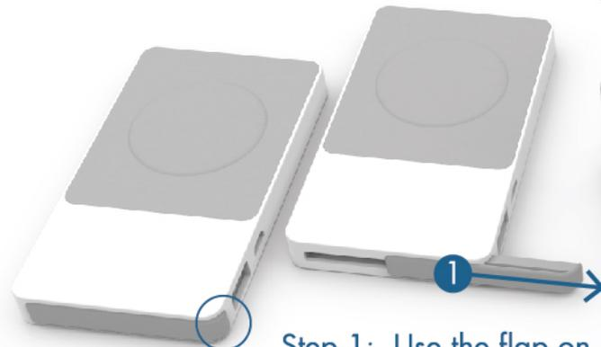
Step 1: Use the flap on the back to slide off the slot cover completely
