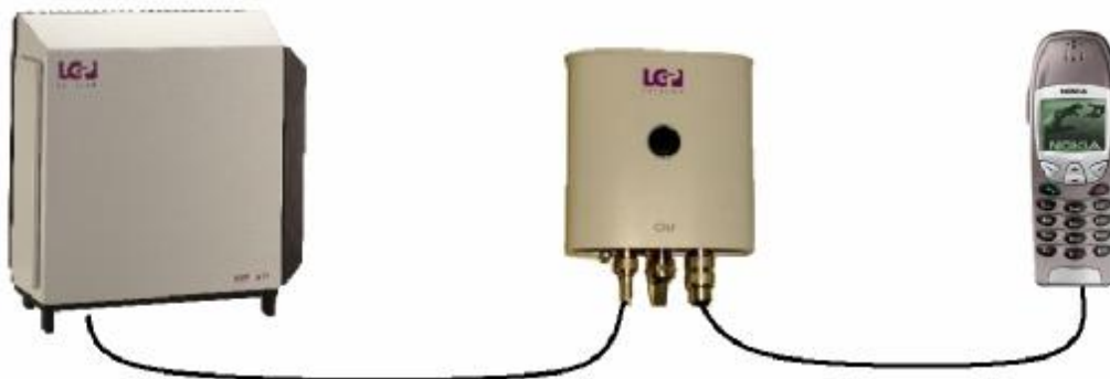
Figure 29 Remote Access to TMB/CIU via GSM modem
