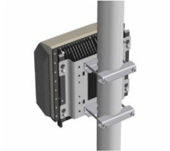
Figure 12 Insert the heads of the screws through the keyhole slots in the mounting plate and lower the TMB until the screw heads are retained by the narrow portions of the slots. (2): Tighten the screws.
