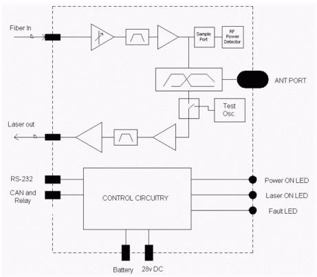
The US series Remote Modules have a Fiber-Optic transceiver pairs downlink and uplink filtering, and an downlink RF Power Amplifier.
