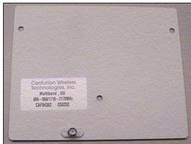
Figure B- 9: GSM Antenna
