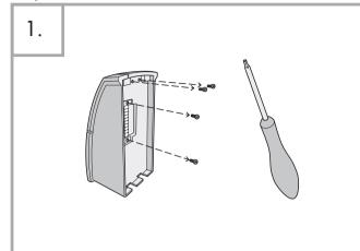
Unscrew the four screws on the back of Precise BioAccess<sup>TM</sup>.
