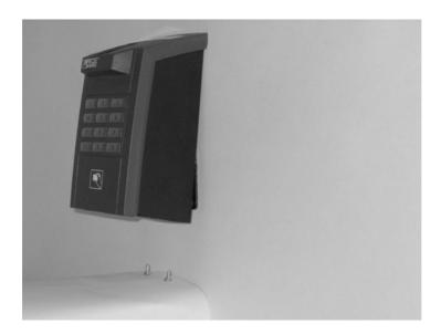
Secure Precise BioAccess™ 200. Use only screw driver Torx T10. Torque max 1.0 Nm.
