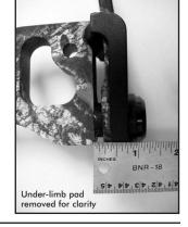
Some PSE bows are equipped with a special asymmetric idler wheel, which is assembled on the top limb. It is essential that the idler be oriented properly. The wide edge of the idler always goes to cable guard side of the bow. The illustration shows the proper orientation of the idler for a right-handed bow when viewed while holding the bow (from behind).
