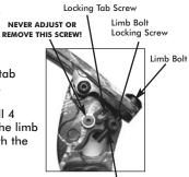
Back limbs out until they are flush with the bottom of anchor
