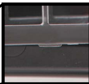
Bottom tabs already pulled loose from the device.
