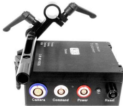
MDR2 with 15mm rod bracket p/n 4335 and swing arm p/n 4302
