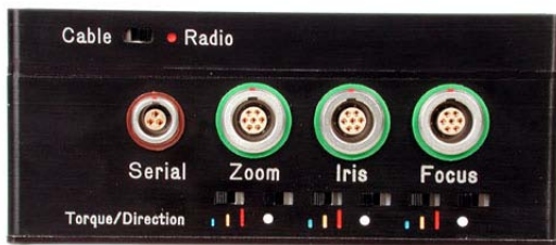
MDR2: Torque and Direction Switches
