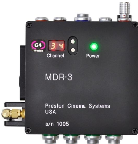
MDR3: Channel Display & Switches – Top
