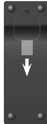
Remove the plastic tab from the back of the Display Remote. Location of plastic tab may differ from the illustration.
