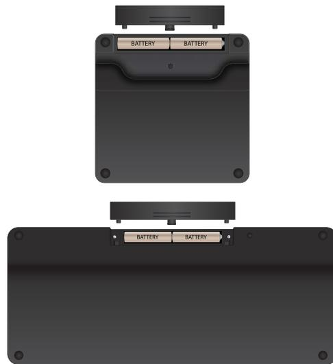
Insert the included AAA batteries into the Wireless Keyboard and Wireless Touchpad. Match the + and - symbols in the battery compartment.
