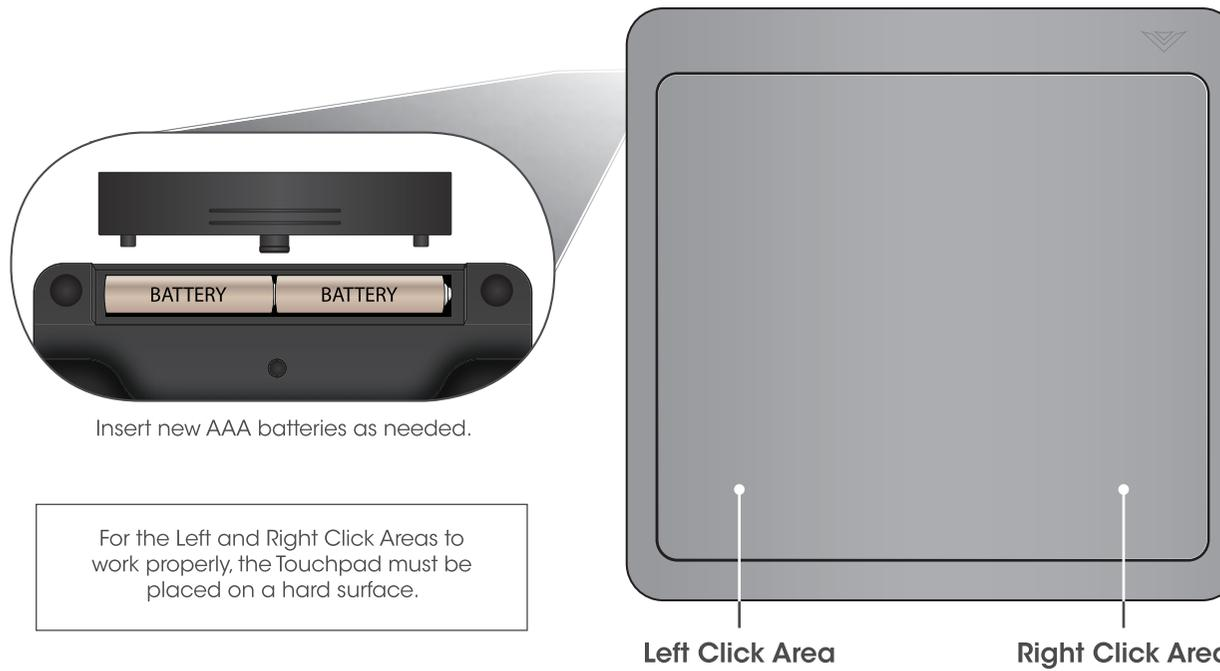
For the Left and Right Click Areas to work properly, the Touchpad must be placed on a hard surface.
