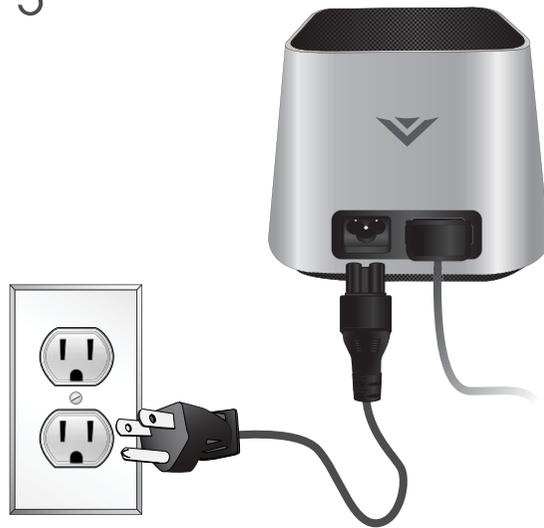
Connect the Power Cable to the Subwoofer, then plug into a grounded electrical outlet or power strip.
