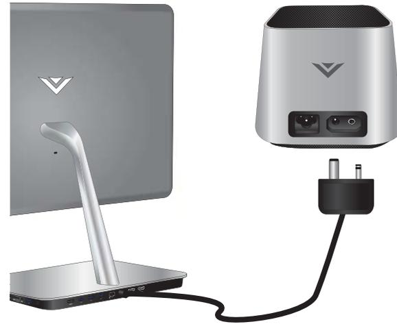
Connect the PC to the Subwoofer. You can use the included Extension Cable if you prefer to place the Subwoofer on the floor.
