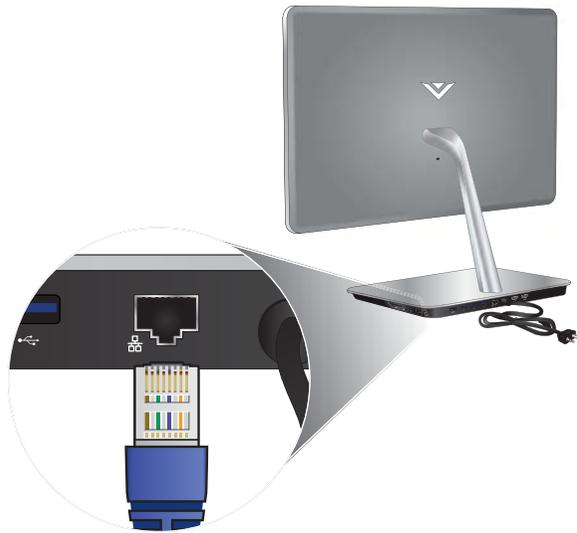
Connect an Ethernet cable\* from your router or modem to the Ethernet port on the back of the PC. If you plan to connect to the internet wirelessly, you can skip this step.
