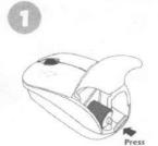
Press the button and open the battery door to insert one AA battery.
