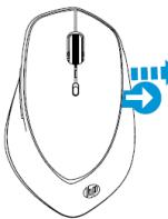
Pull off the battery insulation tap
