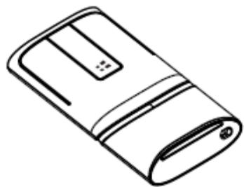
2) Rotate the bottom half of the device 180° angle to switch to mouse mode as shown
