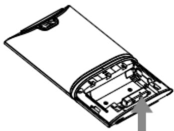
3) Insert two AAA batteries as shown
