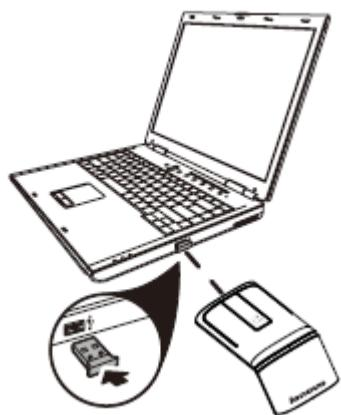
2) Set up the device as shown and switch to BT4.0BLE wireless transmission mode
