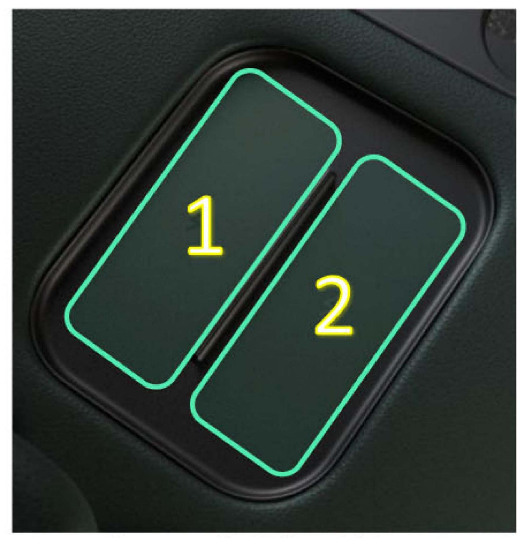
**NOTE:** The Zoox Wireless Charger may not function properly if a device's case is too large to fit fully within a charging zone, too thick, or made of a conductive material such as metal. In these scenarios, remove the case before placing the device on the charger. Do not place metallic or magnetic objects such as credit cards between the device and the charger. Doing so could cause damage to the object and/or charger. Remove any case-mounted wallets prior to charging.
