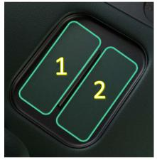
**NOTE:** The Zoox Wireless Charger may not function properly if a device's case is too large to fit fully within a charging zone, too thick, or made of a conductive material such as metal. In these scenarios, remove the case before placing the device on the charger. Do not place metallic or magnetic objects such as credit cards between the device and the charger. Doing so could cause damage to the object and/or charger. Remove any case-mounted wallets prior to charging.
