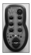
**ON/STOP/OFF BUTTON** [Located on upper right of remote] Press to turn Power ON. Press and hold button down 5 second to turn POWER OFF. Press to STOP sound when sound is playing.
