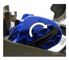
Push down each media holder lock lever to secure the media holders in place
