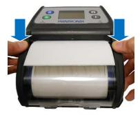
Press down on both sides of the media cover to ensure it is closed correctly.
