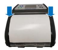
Press down on both sides of the media cover to ensure it is closed correctly.
