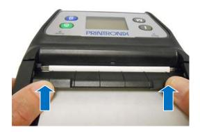
Push the label peel cover toward the front of the printer until it covers the plate roller
