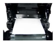
Route the media, printing side out, through the bottom external label slot
