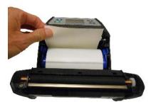
Place the roll, printing side face-out, between the media holders and insert hubs into the core. Pull out enough paper above the printhead
