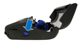
Open the printer media cover by pressing down on the media cover release latch.
