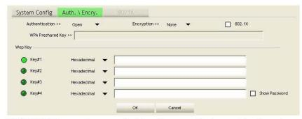
**Profile Name:** User can chose name for this profile, or use default name defined by system. **SSID:** User can key in the intended SSID name or use pull down menu to select from available APs.
