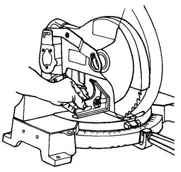
c. Loosen the right side bevel stop lock nut. Lower the bevel stop bolt down as far as it will go.
