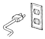
This power tool is equipped with a 2-conductor cord listed by Underwriters Laboratories (UL). The plug permits you to use any conventional 120-volt electrical outlet without necessity for maintaining a ground connection.
