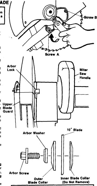
WARNING: After installing a new blade, make sure the blade clears the table slot at the 0° and 45° bevel positions. Lower the blade into the lower table and check for any contact with the base or turn table structure.
