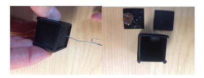
You will need a paper clip for this. Find the bottom of the cube and push the paper clip into the hole to push the bottom electronics and plastic false bottom out of the cube. Remove the electronics and false bottom with your fingers.
