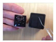
Install the electronics into the base with the batter going in first and covering the hole in the bottom of the box. There are four small posts in the corners of the box to hold it perfectly level. The battery clasp should cover the hold so that when you poke it out with a paper clip you are poking the battery.
