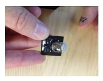
Install the battery with the '+' side up. When installing the battery, the '6' side is up when the battery clasp is up.
