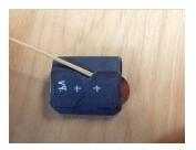
The receiver comes with two CR2032 batteries already installed. When the batteries are drained, the receiver will give one long, weak buzz, or just stop working. You'll notice that the range also decreases when the battery is low.
