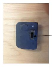
Slide the on/off switch. (See photo, below left.) When you switch the receiver on, it will vibrate for one second, letting you know it is ON. It does not vibrate when you switch it OFF.
