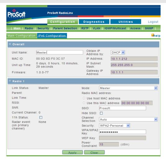
To configure a Master radio, make the following changes to the web configuration form:
