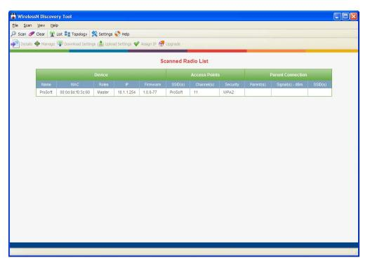
The window lists all the radios your computer can access. The MAC ID number is essentially the serial number of the radio; this number is also printed on the side of the radio. If a radio listing does not appear in the window, click the **SCAN** button on the toolbar. If you still do not see a radio listing, refer to Diagnostics and Troubleshooting (page 41) in the RLXIB-IHN User Manual.
