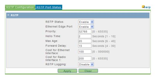
Note: RSTP is not VLAN aware. If RSTP is enabled in a network that uses VLANs, there may be paths that have unblocked loops thereby nullifying the effectiveness of RSTP.
