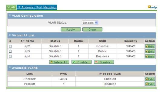
A given radio can have multiple virtual APs (VAPs) configured on it, and these virtual APs can be active concurrently. There is a general mode AP that is the default link for parent and child connections. This general mode AP is VLAN-aware, in that there is filtering for VLAN tags enabled along this link.
