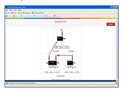
The Topology view shows a diagram of the network's wireless connections. Use this view to see whether all the radios are linked, and that you approve of the way the radios are linked.
