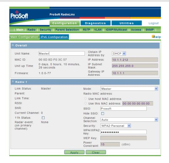
Important: In order to connect to a RLXIB-IHN radio from a web browser or SNMP agent, both your computer and the radio must have IP addresses, and these IP addresses must be on the same subnet.
