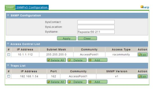
The RLXIB-IHN SNMP agent supports the SNMPv2c and SNMPv3 protocol versions, and can send traps to a specified community.
