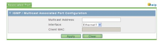
This mapping is used by the device to send directed multicast frames to the client over the 802.11 link.
