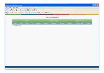
The window lists all the radios your computer can access. The MAC ID number is essentially the serial number of the radio; this number is also printed on the side of the radio. If a radio listing does not appear in the window, click the **SCAN** button. If you still do not see a radio listing, see Troubleshooting (page 46).
