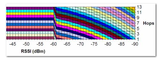
Once per second, the RLXIB-IHN radio evaluates the link it has to its parent to determine if this link is the best parent to use. A cost is calculated for each entry and can be seen in the column labeled "Cost" in the preceding table. The cost calculation is based not only on the strongest signal, but on several other factors to provide optimum network communication. There is built in hysteresis to prevent frequent link fluctuations.
