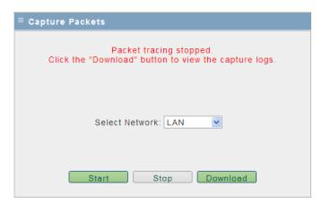
To view the contents of the captured packets, you must download the capture file, and open it in a network protocol analyzer. Click **DOWNLOAD** to retrieve and open the capture file.
