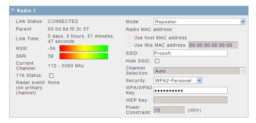
Note: Each Radio's configuration is unique. If the hardware supports two radios, there will be two instances of the Radio Configuration/Status area, one per radio.
