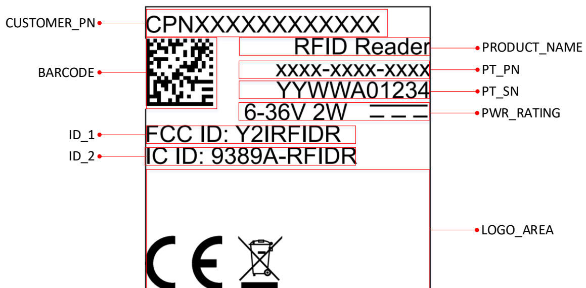
Figure 5-4: Label layout (26x26mm)
